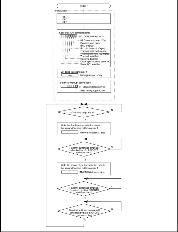
Figure 5 Control procedure of transmitter
