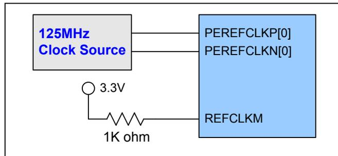
Figure 7 125 MHz Global Reference Clock Selection
