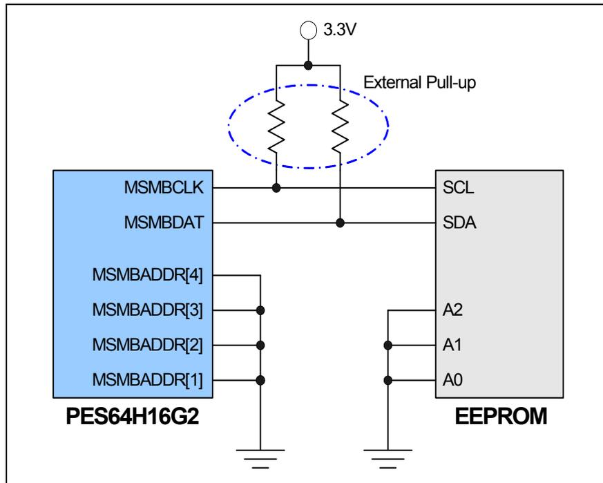
Figure 14 Example of EEPROM Address Configuration for 0x50
