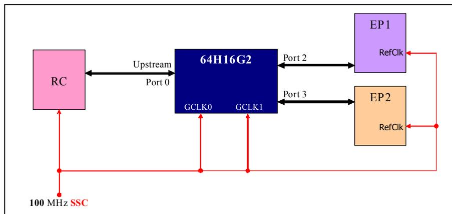
Figure 8 Example of Common Clock Mode with SSC
