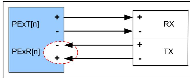
Figure 2 Polarity Inversion
