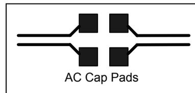
Figure 3 AC Capacitor Placement
