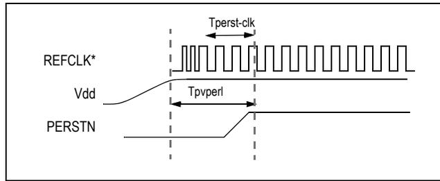
Figure 11 Fundamental Reset
