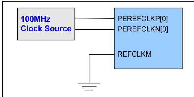
Figure 6 100 MHz Global Reference Clock Selection
