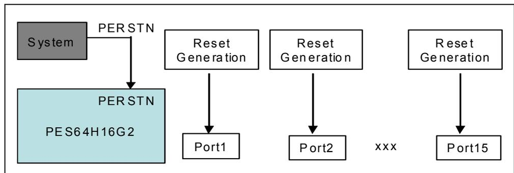
Figure 13 Reset Scheme for Hot Plug Support
