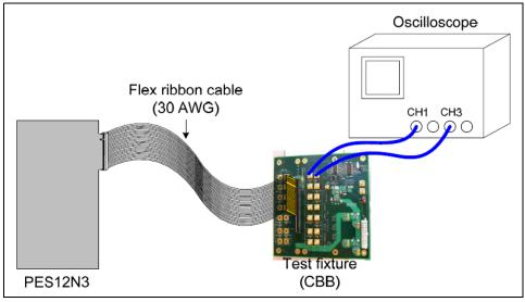
Figure 7 Test 2 Setup
