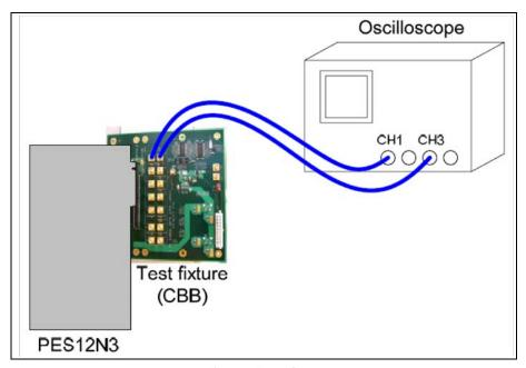
Figure 5 Test 1 Setup
