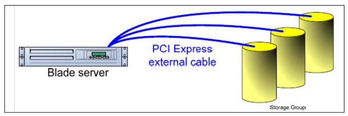
Figure 2 Example of Blade Server Connecting to Storage Group via PCI Express External Cable
