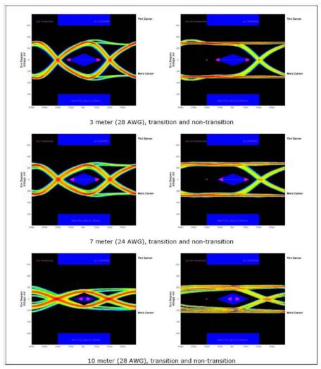
Figure 12 Differential Receiver (Rx) Eye Diagrams at the End of an Infiniband Cable for Lengths of 3, 7, and 10 Meters with Default Tx Setting (-3.35dB Deemphasis, Scale Factor of 1, 20mA Nominal Drive Current, Nominal Tx Termination Value of 50 ohms)
