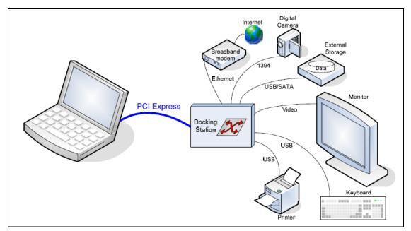
Figure 3 Example of Application Utilizing PCI Express Cable Connecting a Notebook to an I/O Expansion Docking Station
