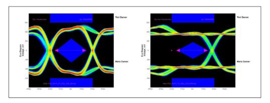
Figure 6 Transmitter Eye Diagrams of PES12N3/PES12NT3 on CBB (no cable) with Default Tx Setting (-3.35dB de-emphasis, Scale Factor of 1, 20mA Nominal Drive Current, Nominal tx Termination Value of 50 ohms)
