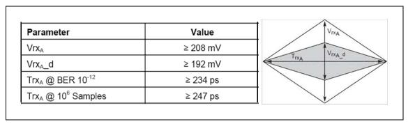
Figure 4 Receiver Path Compliance Eye Requirements and Eye Diagram (from Section 3.3.2 of the External Cabling Specification Rev. 1.0)
