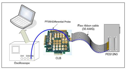
Figure 14 Reference Clock Jitter Test Configuration
