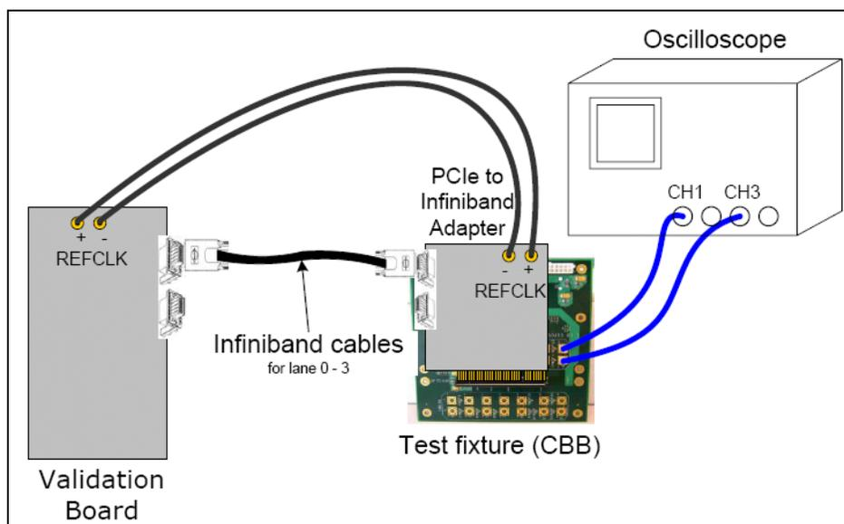
Figure 10 Test 3 Setup
