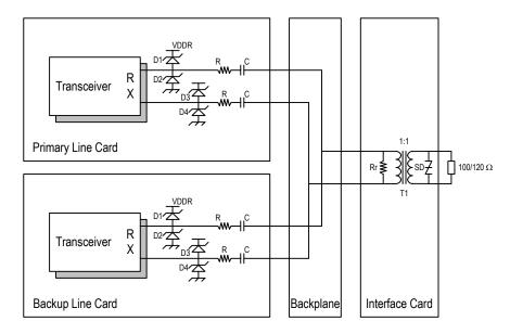
Figure 2. Receive Line Interface Schematic
