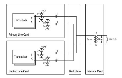
Figure 3. Transmit Line Interface Schematic
