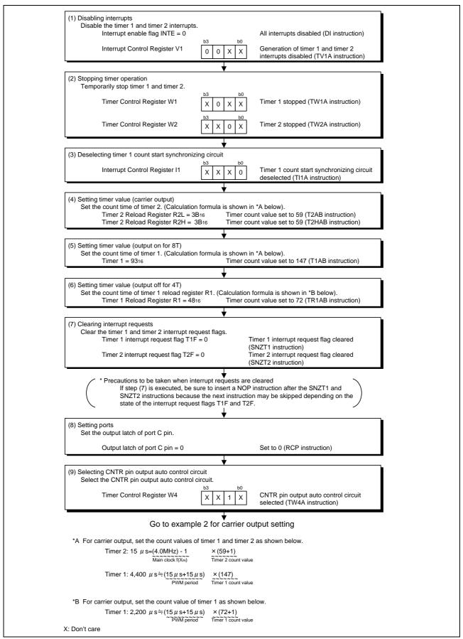
Figure 4.2 Example 1 for Carrier Output Setting
