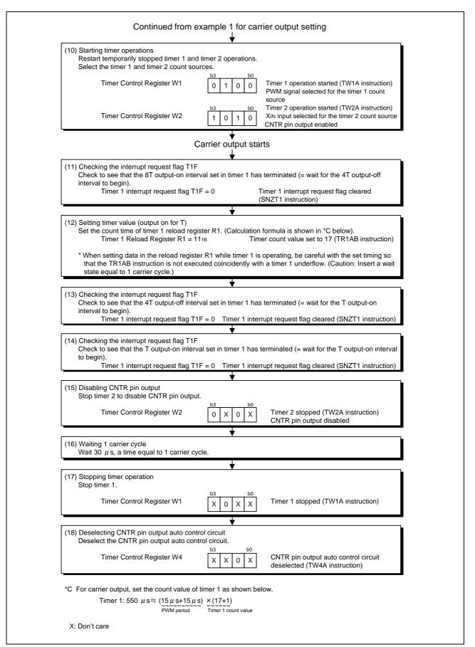
Figure 4.3 Example 2 for Carrier Output Setting
