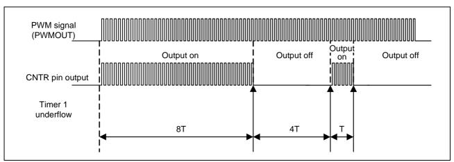
Figure 4.1 Automatic Control of CNTR Output
