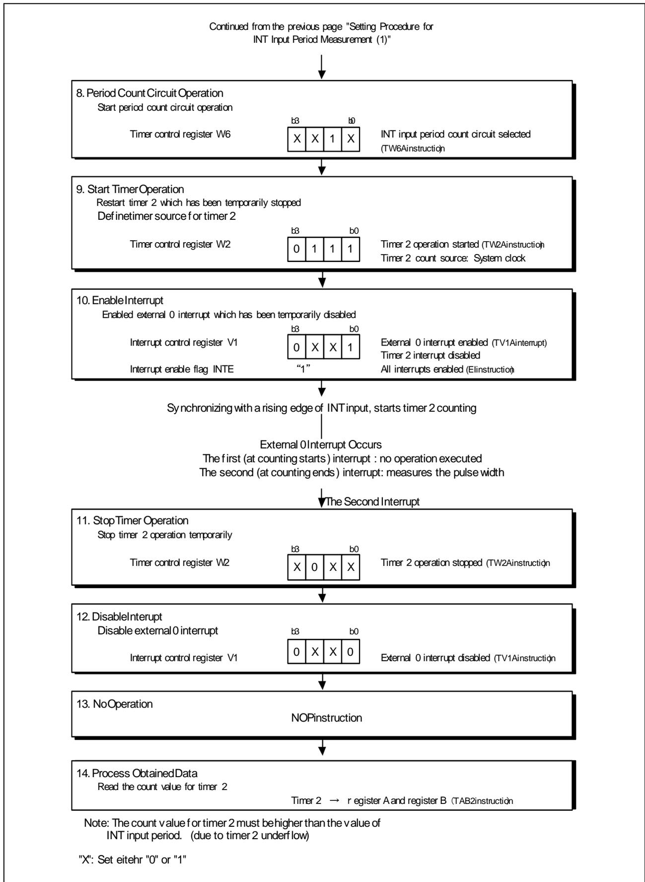
Figure 4.9 Setting Procedure for INT Input Period Measurement (2)
