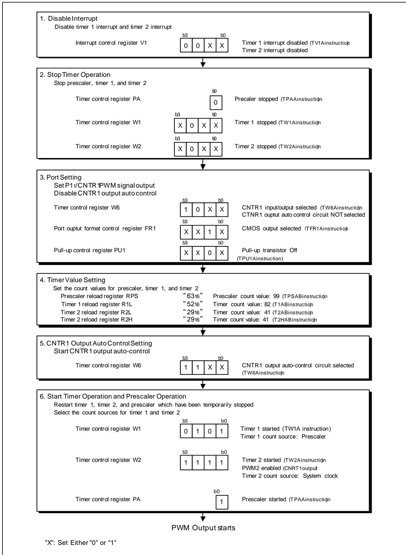
Figure 4.10 Setting Procedure for CNTR1 Output Auto-Control
