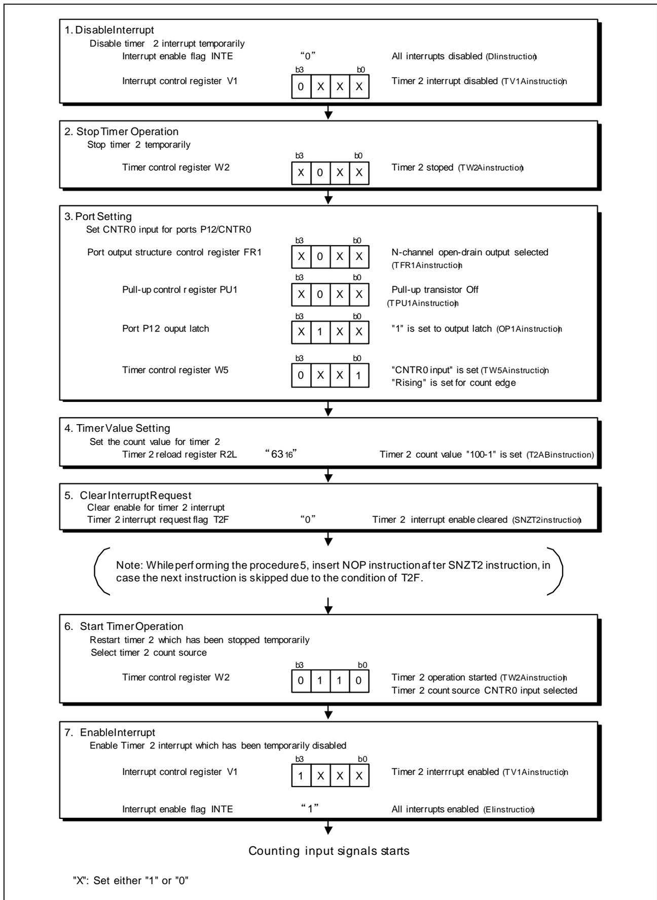
Figure 4.5 CNTR0 Input Setting Procedure
