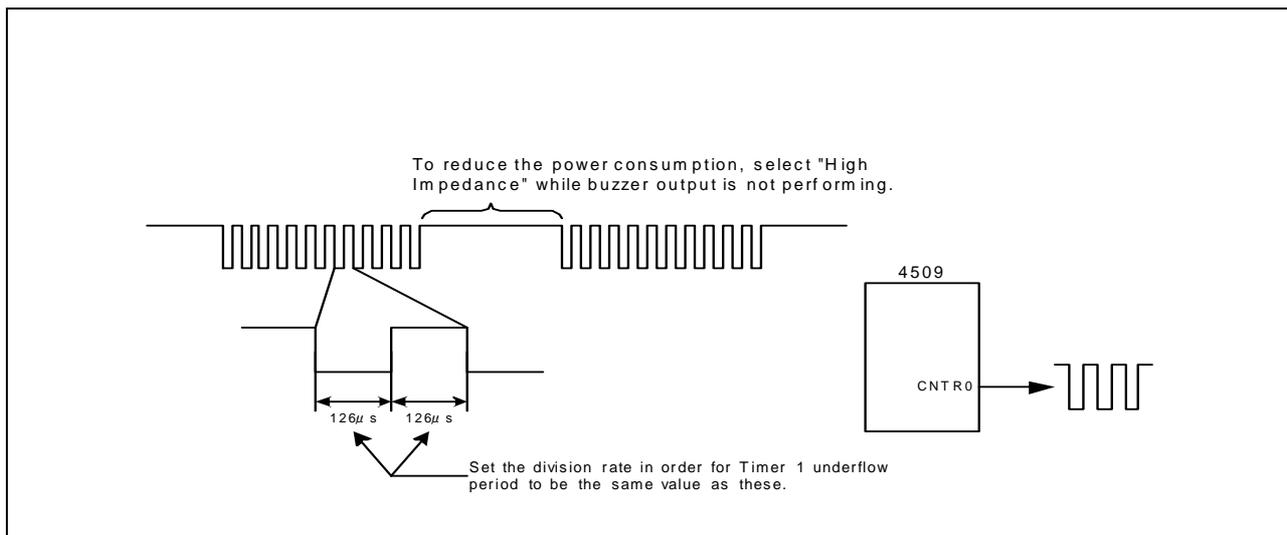
Figure 4.1 Peripheral Circuit
