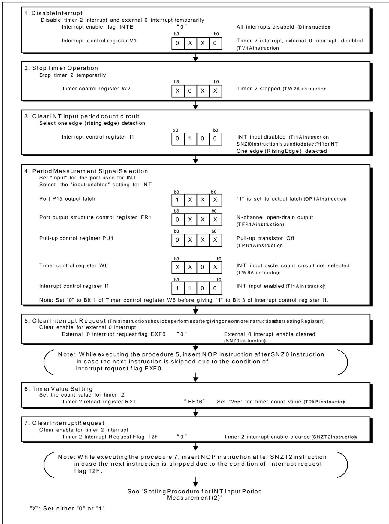
Figure 4.8 Setting Procedure for INT Input Period Measurement (1)
