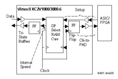
Figure 5. FPGA internal memory performance measurement template
