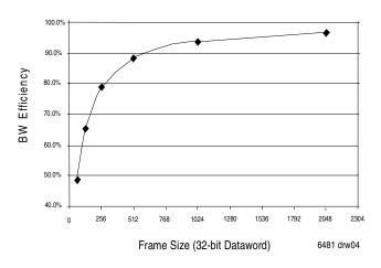
Figure 4. Bandwidth efficiency vs. effective frame size of DSP EMIF interface whil using the DMA
