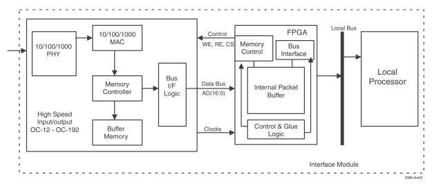
Figure 3. Typical High-Speed Line Interface Module Block Diagram
