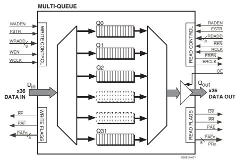
Figure 1. Block Diagram - Multi-queue Flow-control Device
