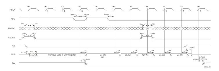
Figure 6. Read Queue Select, Read Operation and OE Timing
