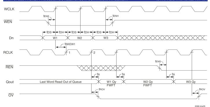
Figure 5. Write Operations & First Word Fall Through
