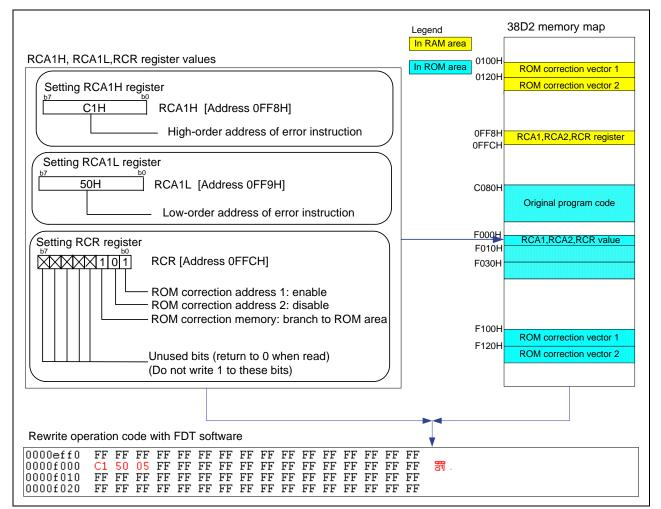
Figure 3 Setting SFR about ROM Correction Function
