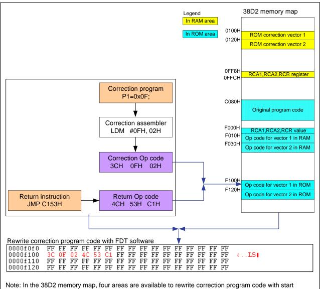
addresses of F010H, F030H, F100H and F120H. They can be used separately or synchronously.
