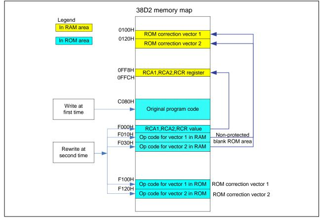
Figure 7 Explanation of Transfer Subroutine
