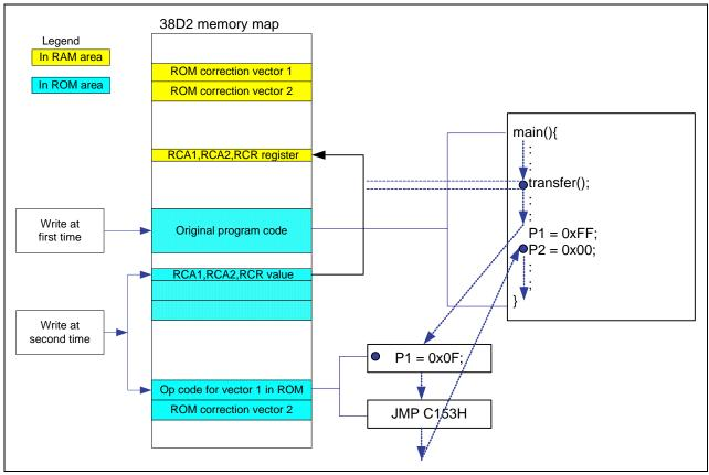
**Figure 6 ROM Correction Function Process**
