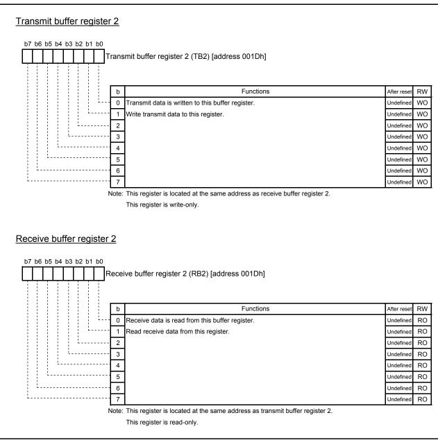
Fig. 4.18 Structure of Transmit buffer register 2/Receive buffer register 2
