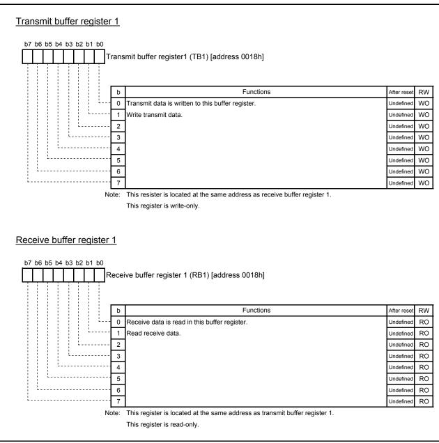
Fig. 4.13 Structures of transmit buffer register 1 and receive buffer register 1
