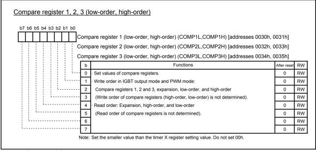
Fig. 4.36 Structure of Compare register 1, 2, 3 (high-order, low-order)
