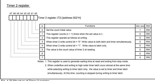
Fig. 4.22 Structure of Timer 2 register
