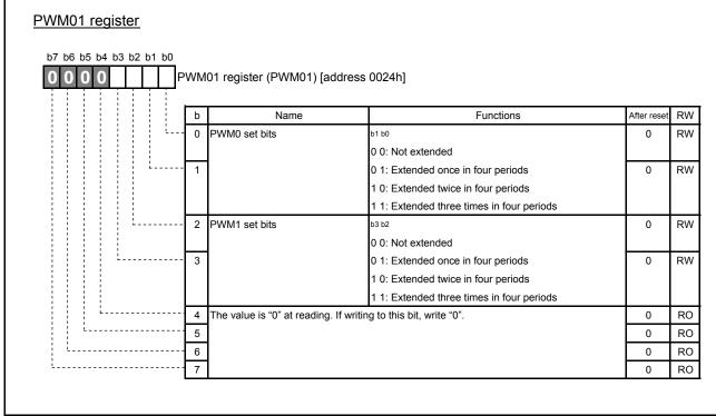
Fig. 4.25 Structure of PWM01 register
