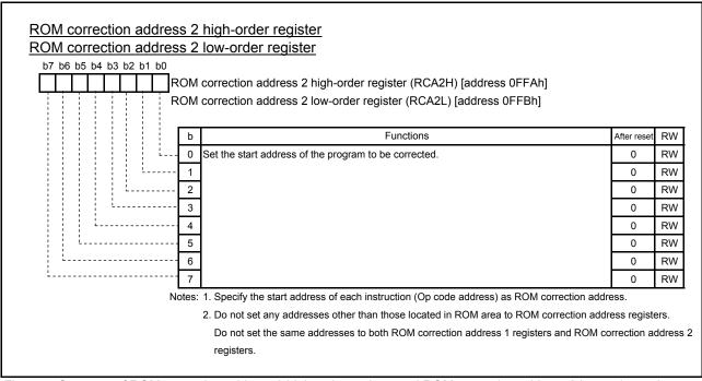
Fig. 4.57 Structure of ROM correction address 2 high-order register and ROM correction address 2 low-order register
