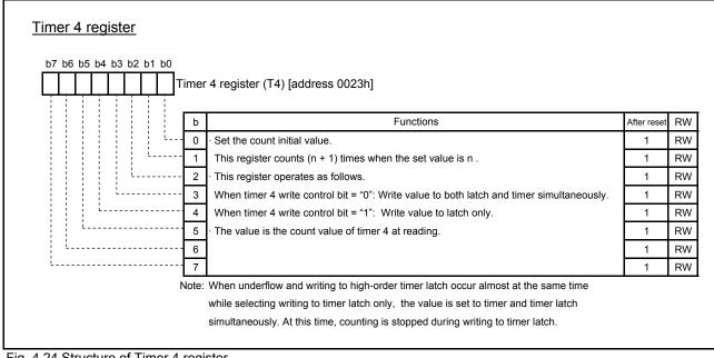
Fig. 4.24 Structure of Timer 4 register
