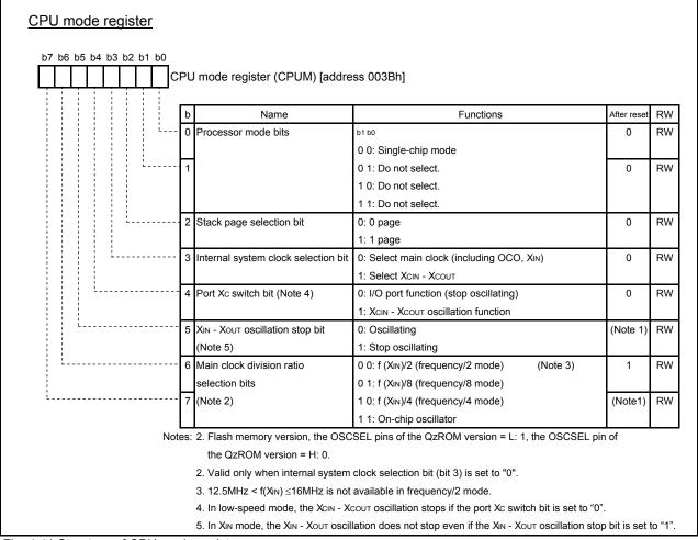
Fig. 4.41 Structure of CPU mode register
