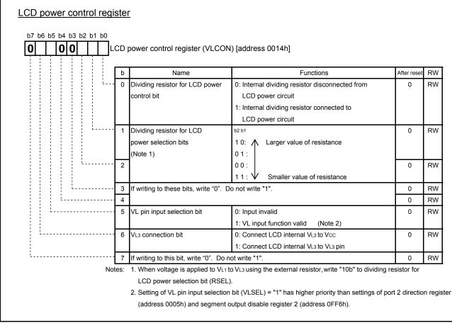
Fig. 4.9 Structure of LCD power control register
