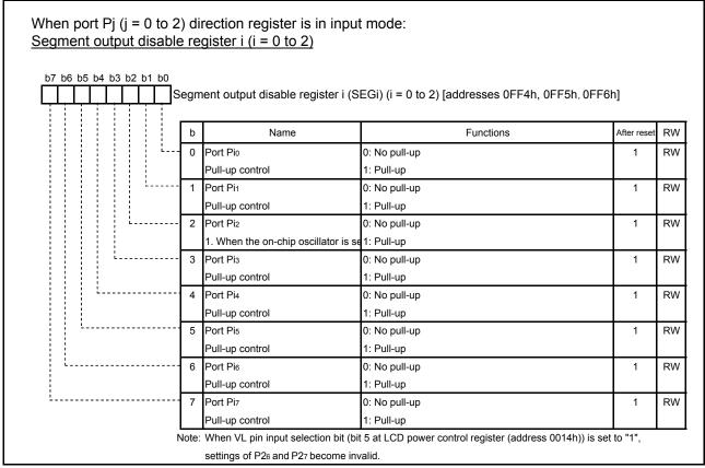
Fig. 4.54 Structure of Segment output disable register i (i = 0 to 2)
