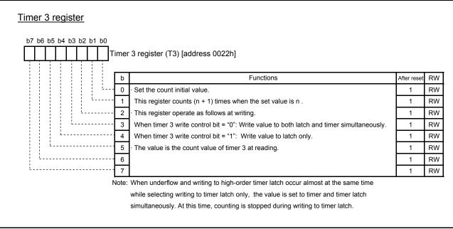
Fig. 4.23 Structure of Timer 3 register
