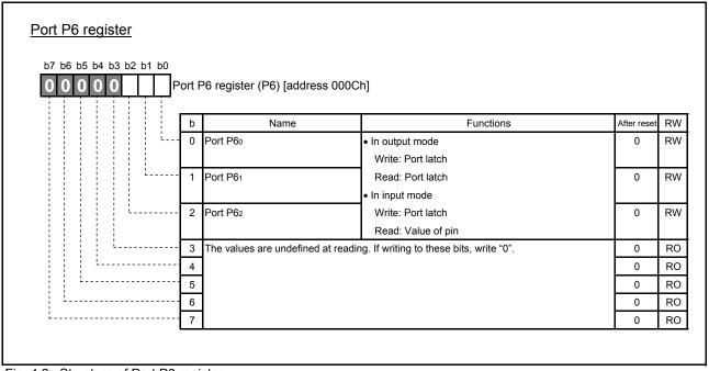
Fig. 4.2 Structure of Port P6 register
