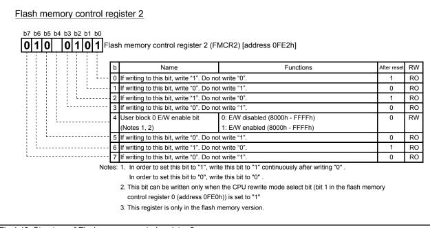
Fig.4.48 Structure of Flash memory control register 2
