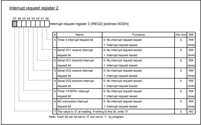
Fig. 4.43 Structure of Interrupt request register 2
