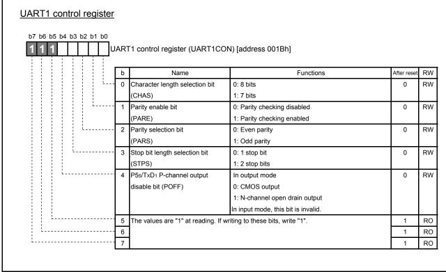
Fig. 4.16 Structure of UART1 control register
