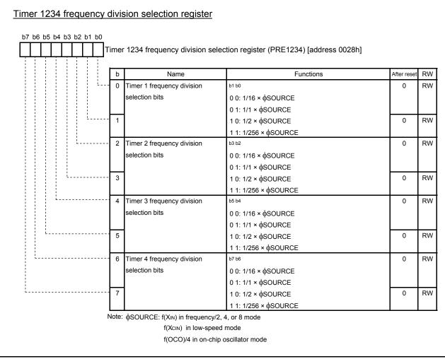
Fig. 4.29 Structure of Timer 1234 frequency division selection register
