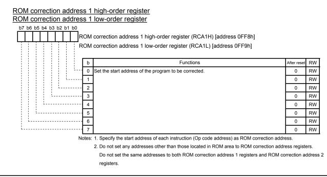
Fig. 4.56 Structure of ROM correction address 1 high-order register and ROM correction address 1 low-order register
