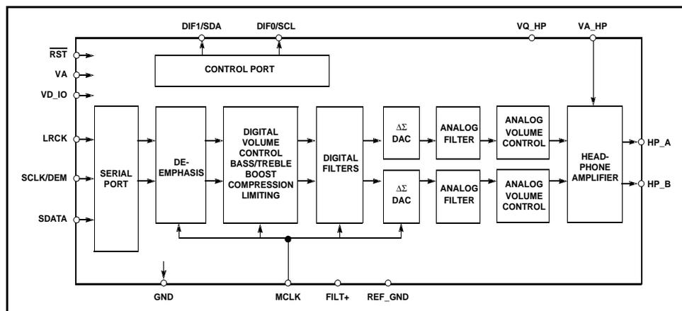
Figure 5 CS4343 Block Diagram (Figure Courtesy Cirrus Logic)
