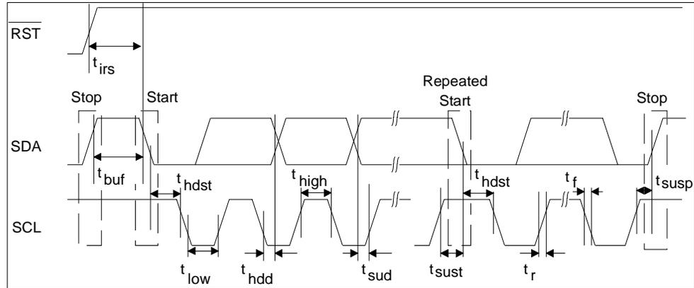
Figure 6 Control Port Timing (Figure Courtesy Cirrus Logic)
