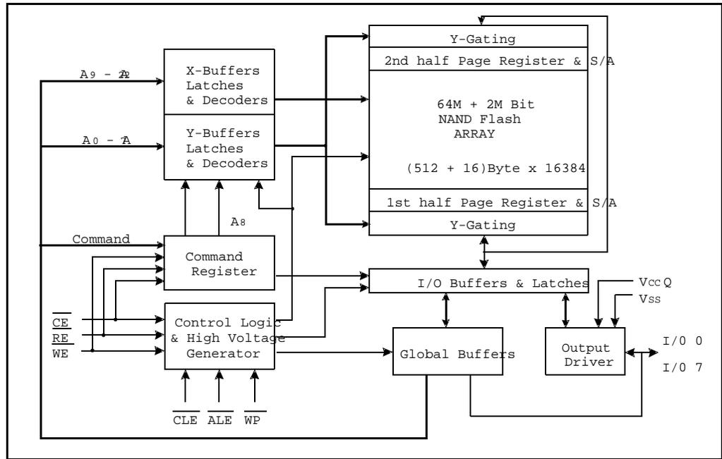
Figure 8 KM29U64000T Block Diagram (Figure Courtesy Samsung Semiconductor)
