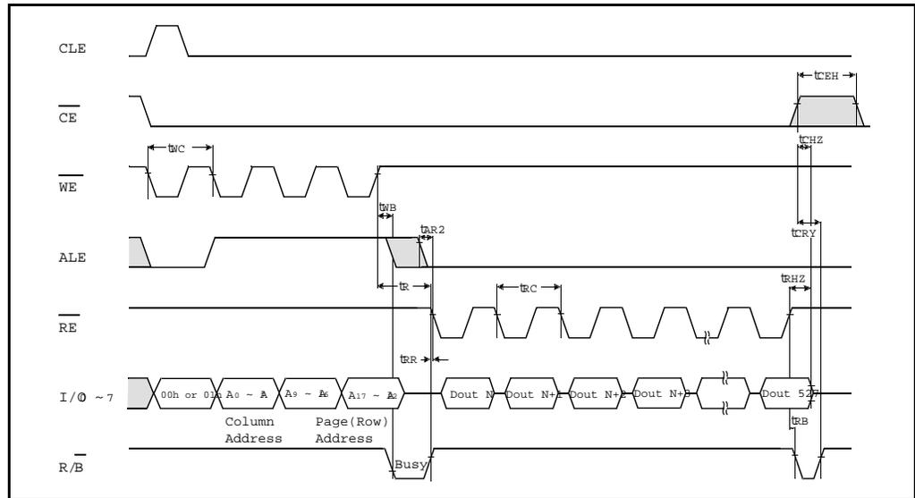
Figure 9 KM29U64000T Read Timing (Figure Courtesy Samsung Semiconductor)
