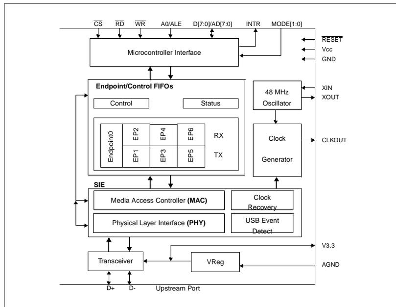
Figure 12 USBN9602 Block Diagram (Figure Courtesy National Semiconductor)
