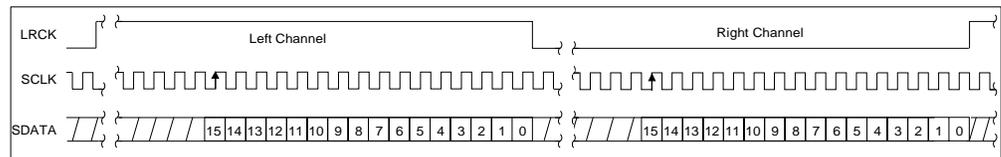
Figure 7 Serial Port Timing (Figure Courtesy Cirrus Logic)
