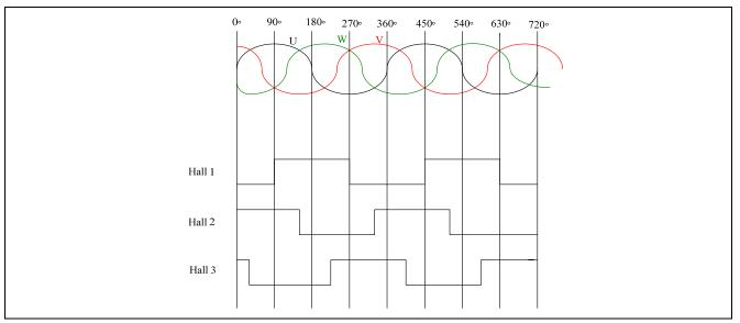
Figure 4 Relationship of Back-EMF and hall sensor signal
