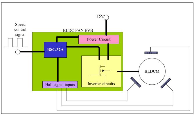
Figure 1 Configuration of system
