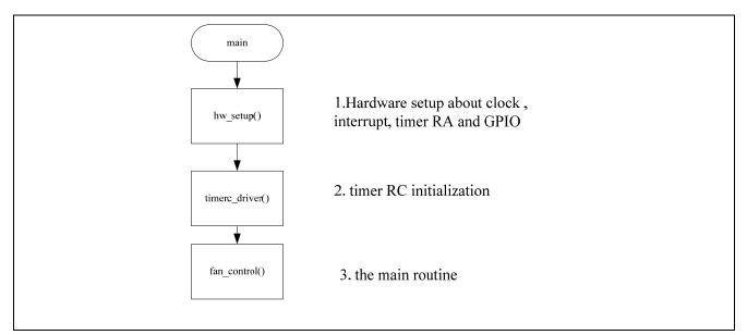
Figure 6 System operation procession
