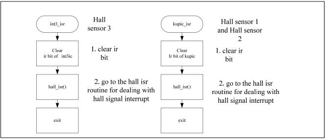
Figure 9 Hall sensor signal interrupt routine
