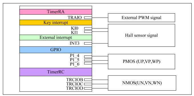
Figure 3 Used modules of R8C/32A
