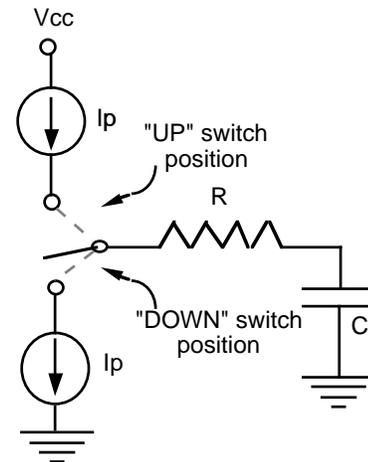
Figure 4. Charge Pump & Loop Filter configuration
