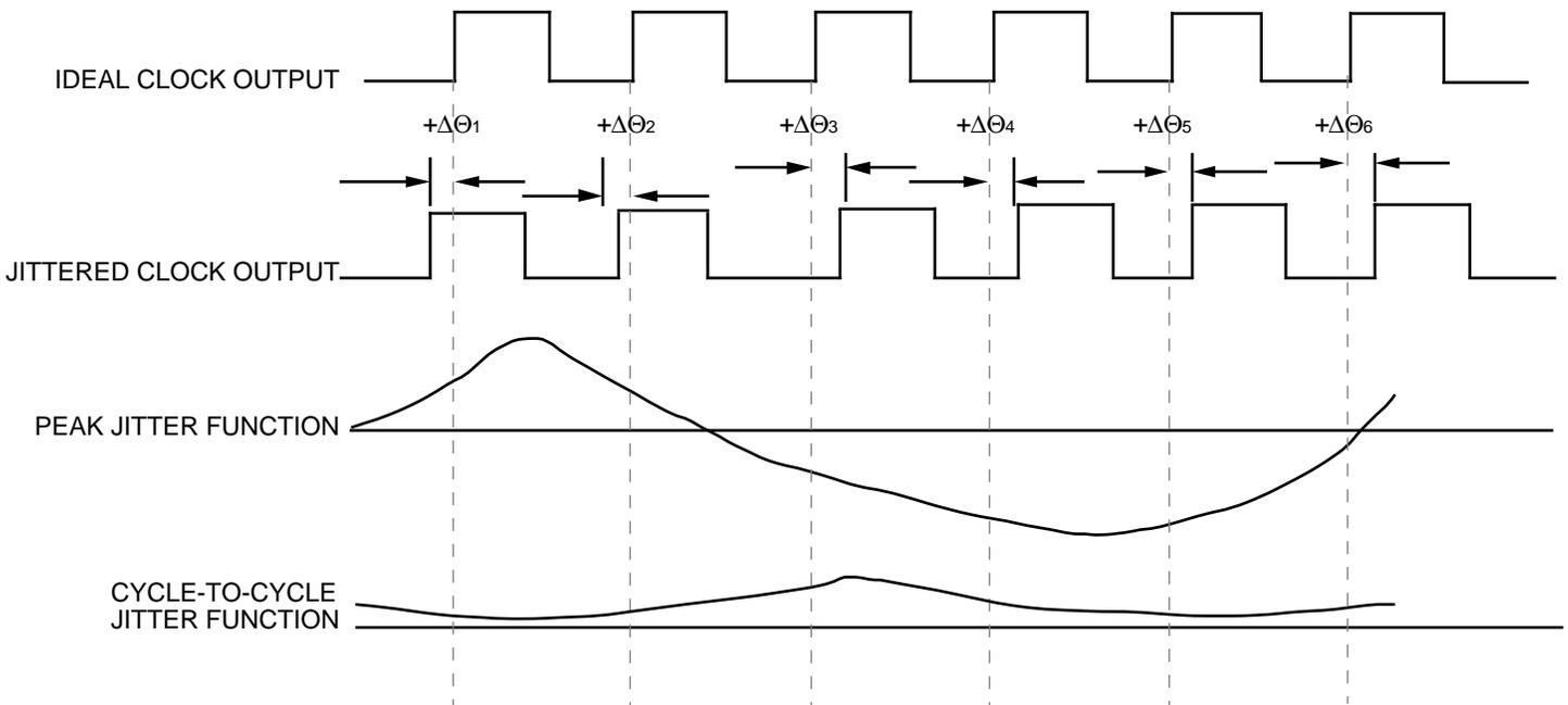
Figure 9. Output jitter
