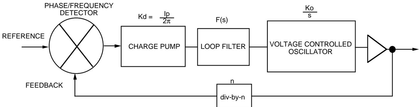
Figure 1. Phase-Lock Loop
