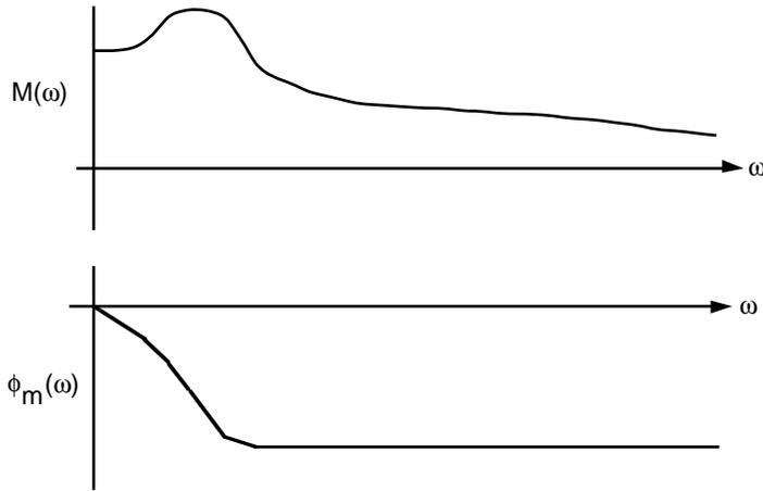
Figure 6. Example of Bode magnitude and phase plots
