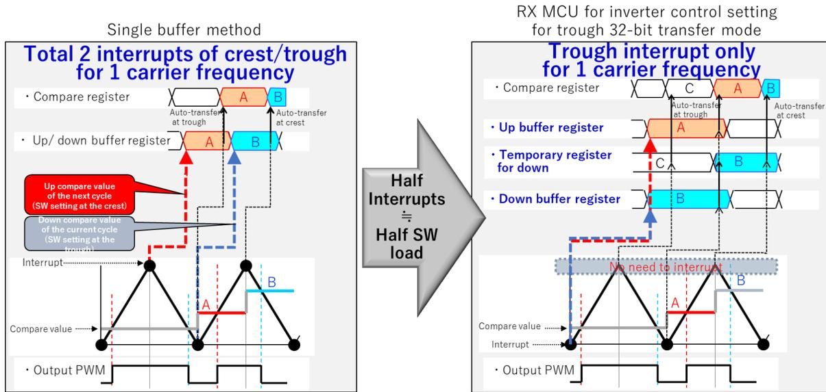
**Figure 3: Double Buffer Function of Three-Phase Complementary PWM Timer**
