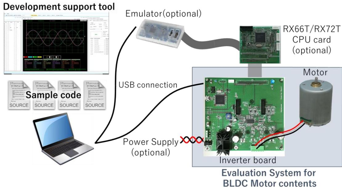
**Figure 12:** Configuration of Evaluation System for BLDC Motor
