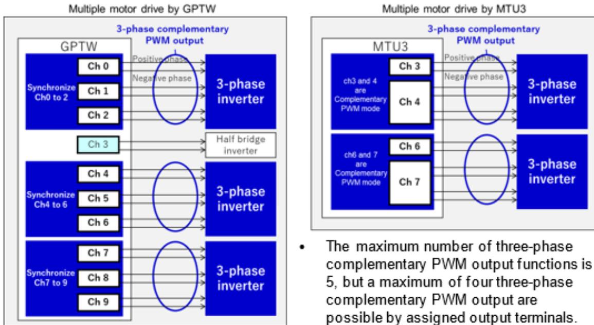
Figure 2: The Number of Three-Phase Complementary PWM Timer
