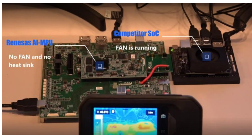
Figure 12: Comparison of Heat Generation between a Fanless DRP-AI Test Board and a GPU with Fan
