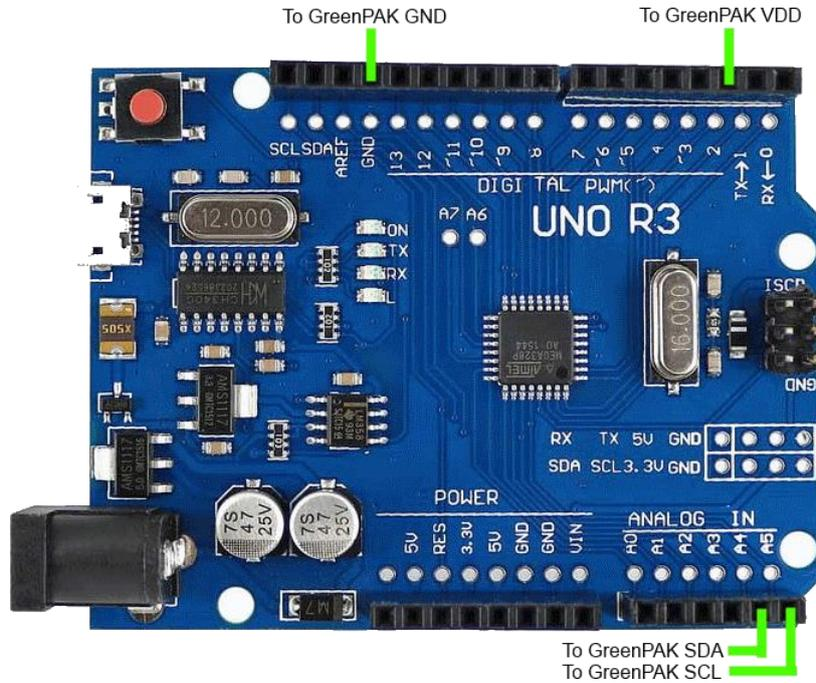
Figure 1. Arduino Connections
