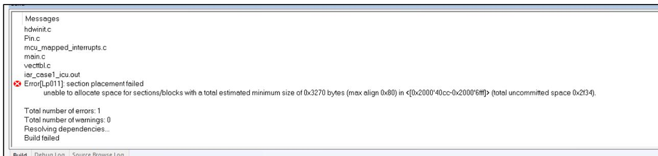
Figure 4-5 IAR build error for section placement failed
