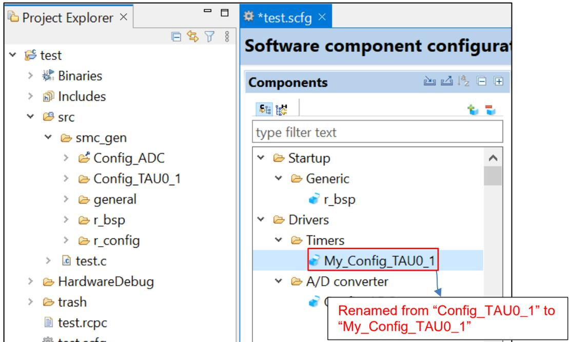
Figure 4-2 The Interval Timer component configuration after renaming
