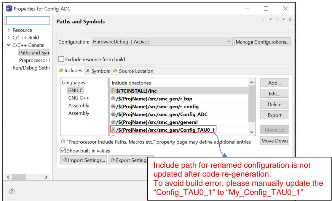
Figure 4-3 Include path setting for the “Config\_ADC” configuration
