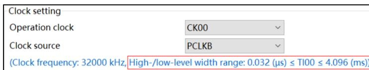
Figure 4-4 High/Low level width min value
