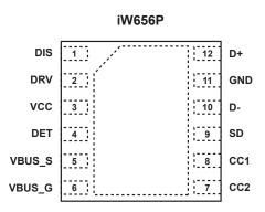
Figure 4.1 : 12-Lead TDFN 3x3mm Package (Top View, Transparent)
