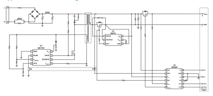
Figure 3.1: iW656P Typical Application Circuit (with iW1791 as the Primary-Side Controller and the iW676 as the Synchronous Rectifier Controller)
