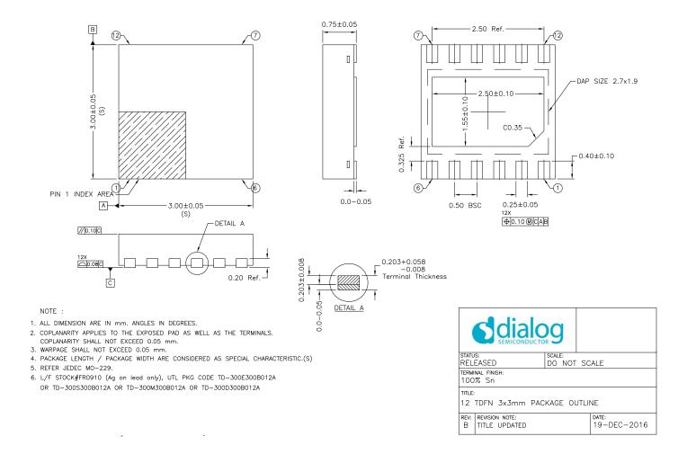
Figure 6.1: 12-Lead TDFN 3x3mm Package
