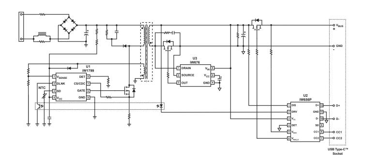
Figure 3.2 : iW656P Typical Application Circuit (with iW1799 as the Primary-Side Controller and the iW676 as the Synchronous Rectifier Controller)
