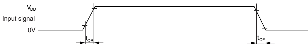
Figure 27-5: Output Rise and Fall Time
