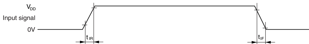
Figure 27-4: Input Rise and Fall Time
