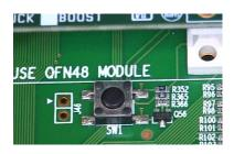
Figure 113. R365 (10 k $\Omega$ ) added next to Reset button
