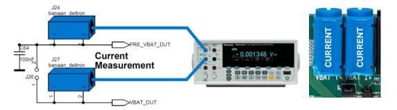
Figure 11. VBAT DUT current measurement setup
