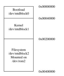
The above diagram shows the physical addresses of the partitions, and the logical naming of the partitions in the /dev subsystem.
