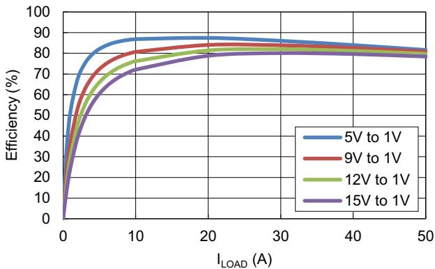
**Figure 18. Conversion Efficiency for Various  $V_{IN}$**
