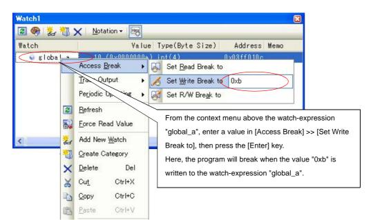
When you have performed the above operation, the set break event (access type) is managed in the Events panel as a Hardware Break event (access type) (see "2.15 Manage Events" for details).
