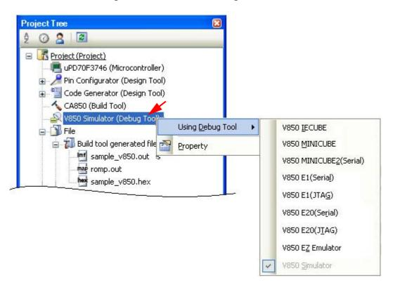
Figure 2-9. Select/Switch Debug Tool to Use
