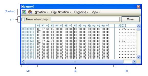
Figure A-34. Memory Panel (When Microcontroller without Data Flash Memory)
