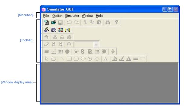
Figure A-93. Simulator GUI Window
