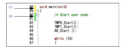
Furthermore, when connected to the debug tool and the downloaded source file is opened, the following mark will be displayed if the update time and date of the source file opened are later than the one of the downloaded load module file (the color of the mark depends on the "Warning" color of the [General - Font and Color] category of the Option dialog box).
