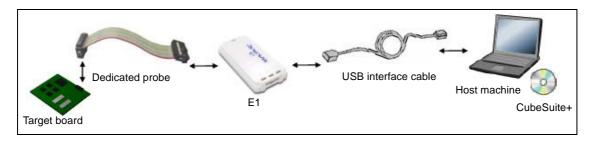
**Remark** You can make a choice among serial communications **[E1(Serial)]**, LPD communications **[E1(LPD)]** and JTAG communications **[E1(JTAG)]** as the communication method to the target board (see "2.3.1 Select the debug tool to use").
