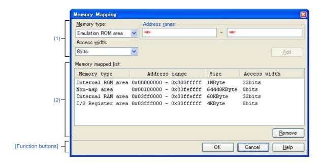
Figure A-51. Memory Mapping Dialog Box [IECUBE[V850E1]]
