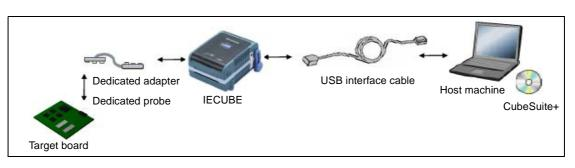
Figure 2-1. Connection Example [IECUBE]
