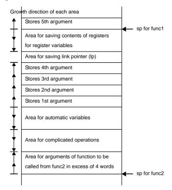
Figure 3-19. Stack Growth Direction of Each Area of Stack Frame
