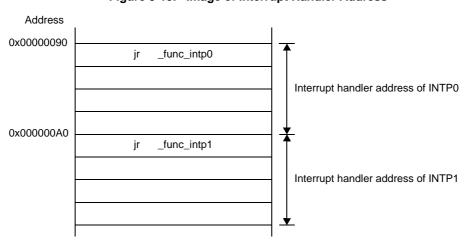
Figure 3-15. Image of Interrupt Handler Address
