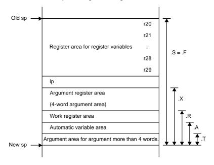
Figure 3-17. Stack Frame (When Argument Register Area Is Located at Beginning of Stack)
