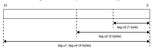
Figure 3-7. Internal Representation of Union Type
