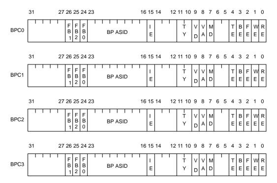
Figure 4-37. Breakpoint Control Register [V850E2]
