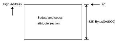
Data with initial values is allocated to the sedata attribute section, and data without initial values is allocated to sebss attribute section. If variables that exceed the upper limit of the sdata and sbss attribute sections that can be accessed from gp with 1 instruction, but which need to be accessed with 1 instruction still exist, they can be allocated in the range that can be accessed with 1 instruction using ep.
