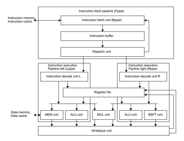
Figure 4-83. Pipeline Configuration (V850E2)
