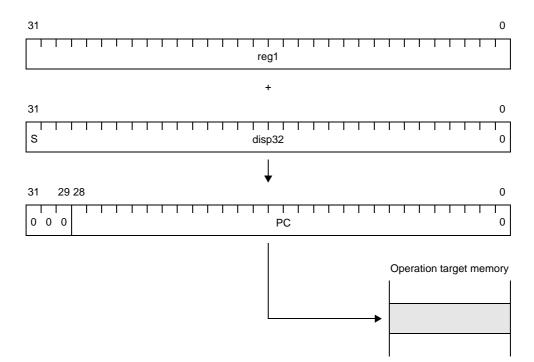
Figure 4-57. Register Addressing (JMP disp32[reg1])[V850E2]
