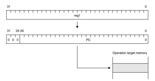
Figure 4-56. Register Addressing (JMP [reg1])[V850E2]
