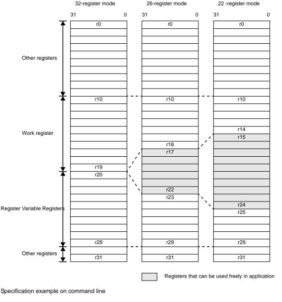
Figure 3-9. Register Modes and Usable Registers
