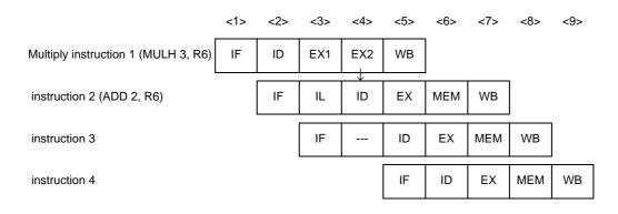
Remark IL: Idle inserted for data wait by interlock function
