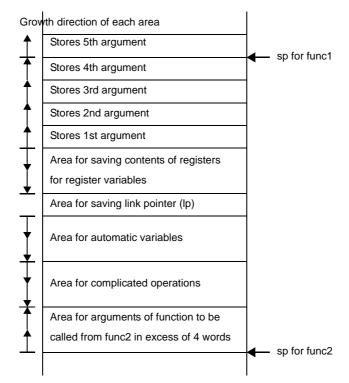
Figure 3-21. Stack Growth Direction of Each Area of Stack Frame
