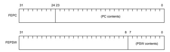
Figure 4-17. NMI Status Saving Registers [V850]
