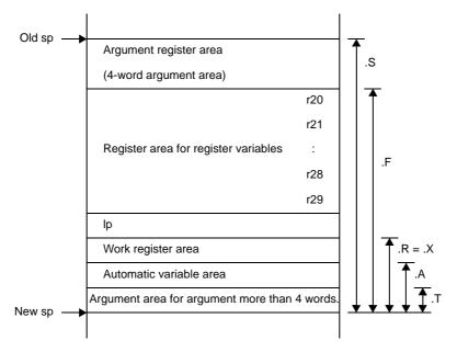
".S, .F, .X, .R, .A, and .T" in the figure are macros for functions output by the compiler internally. macros are used for a specific purpose, as shown in the following table.
