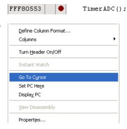
The code will run to the selected line and stop. A temporary breakpoint was automatically inserted in the code and then removed when the program stopped at the breakpoint.
