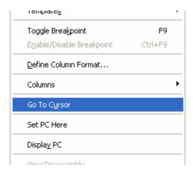
The code will execute to the selected line and stop. An automatic breakpoint was inserted in the code and then removed after calling the break.
