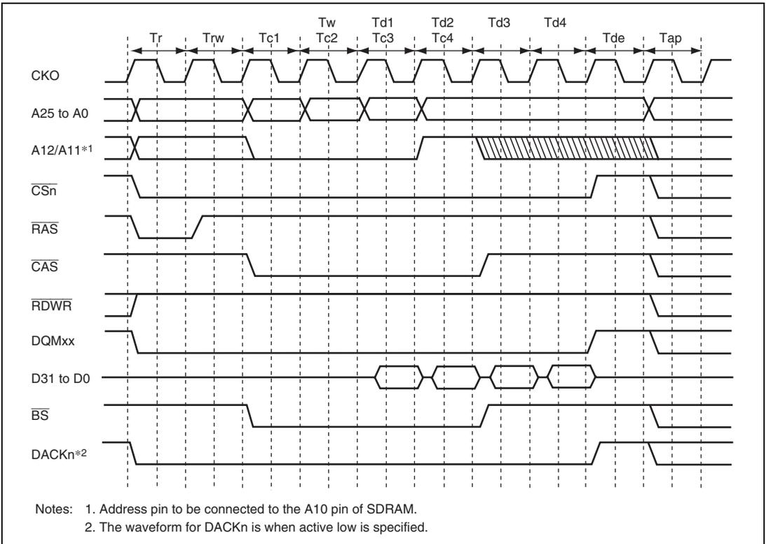
**Figure 11.15 Burst Read Wait Specification Timing (Auto-Precharge)**
