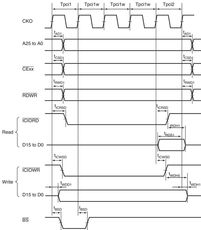
Figure 33.37 PCMCIA I/O Card Interface Bus Timing
