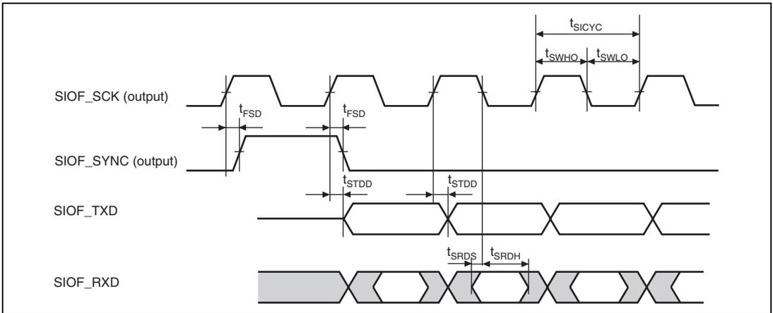
**Figure 33.47 SIOF Transmission/Reception Timing (Master Mode 1, Fall Sampling)**
