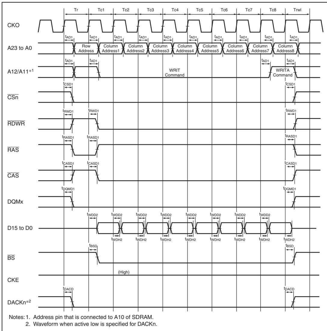
**Figure 33.22 Burst Write Bus Cycle of SDRAM (Single Write × 8)
