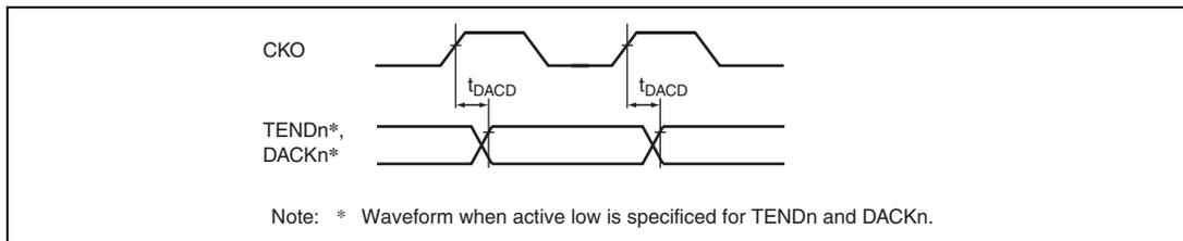
**Figure 33.42 TEND, DACK Output Timing**
