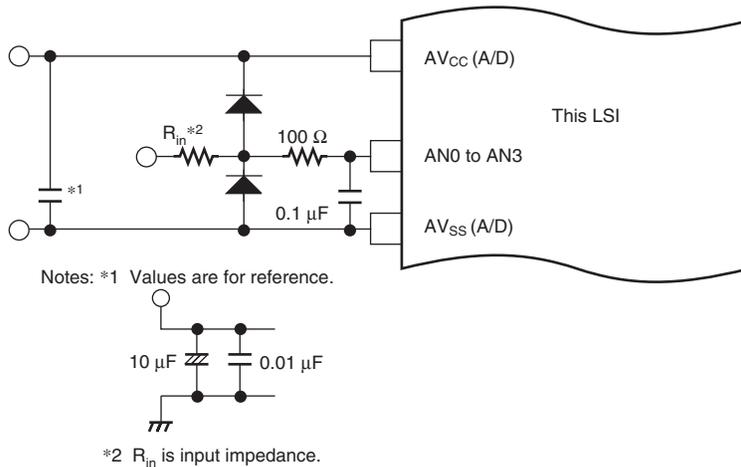
**Figure 26.9 Example of Analog Input Protection Circuit**
