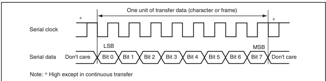
**Figure 22.11 Data Format in Clock Synchronous Communication**
