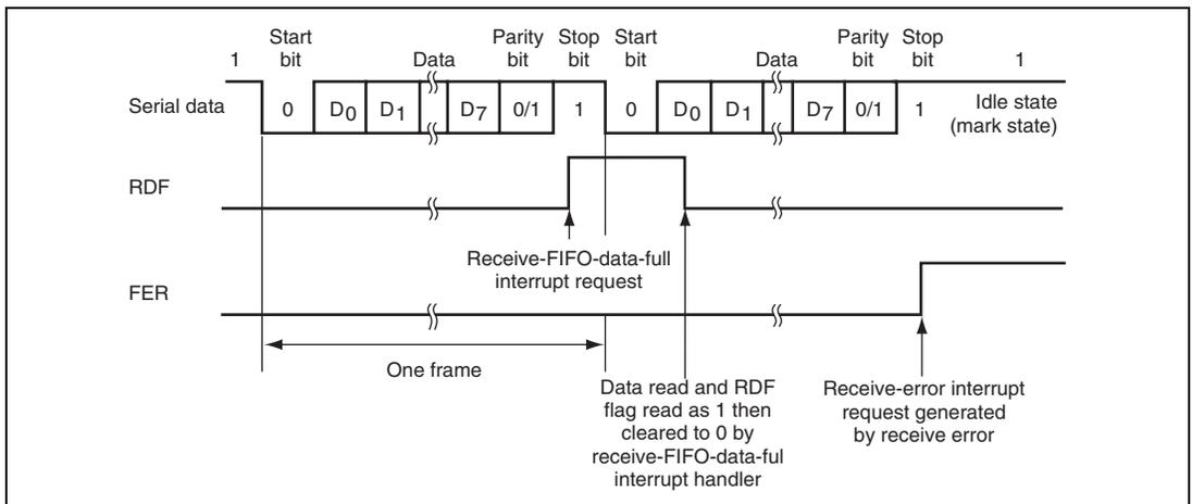
**Figure 23.9 Example of SCIFA Receive Operation
