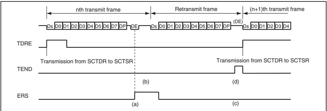
**Figure 25.9 Retransmit Standby Mode (Clock Stopped)
