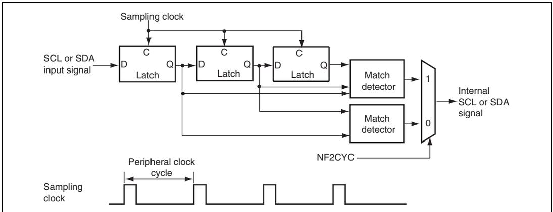
**Figure 20.13 Block Diagram of Noise Filter**
