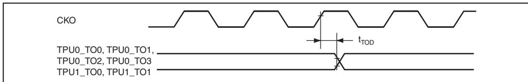
**Figure 33.43 TPU Output Timing**
