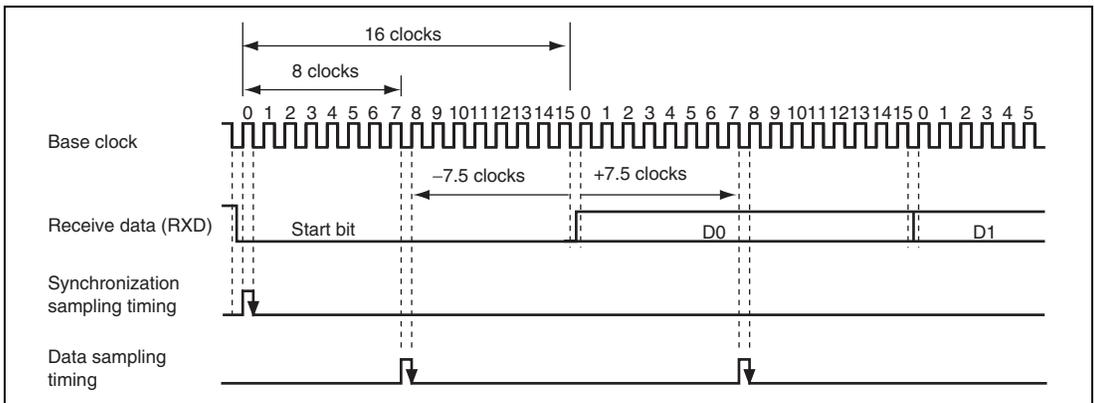
**Figure 23.22 Receive Data Sampling Timing in Asynchronous Mode**
