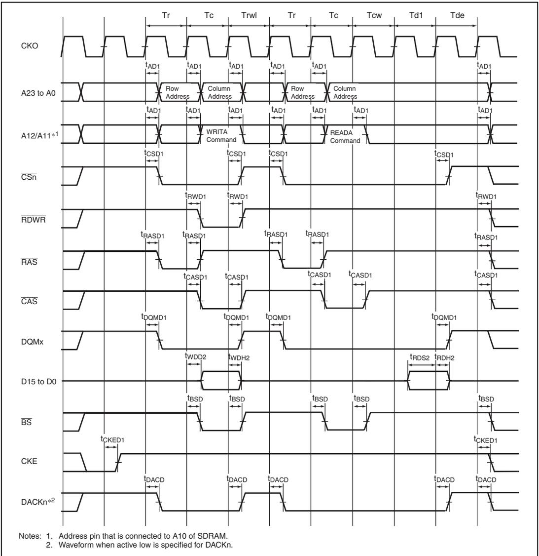
**Figure 33.33 Write-to-Read Bus Cycle in Power-Down Mode of SDRAM
