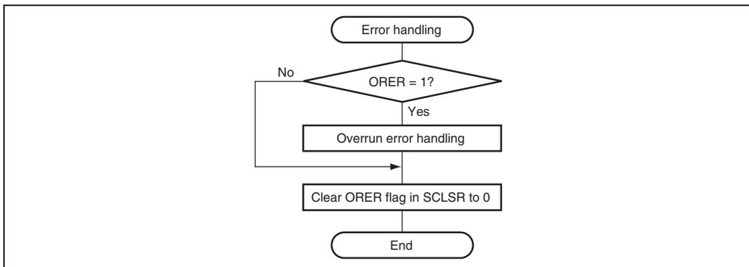
**Figure 22.16 Sample Flowchart for Receiving Serial Data (2)**
