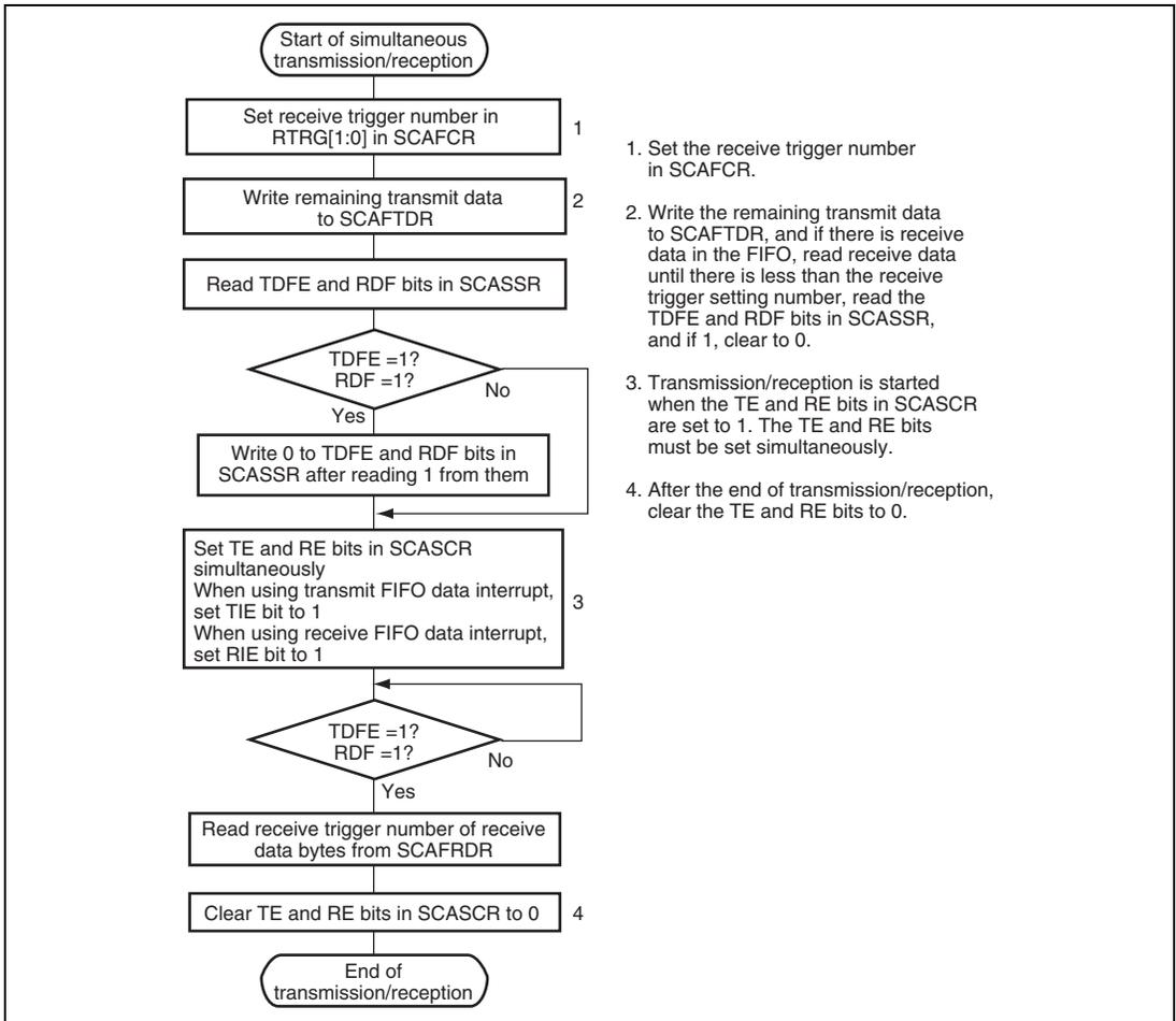
**Figure 23.20 Sample Simultaneous Serial Transmission and Reception Flowchart (1)
