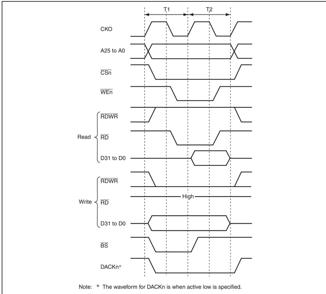
**Figure 11.30 Basic Access Timing for Byte-Selection SRAM (BAS = 0)**
