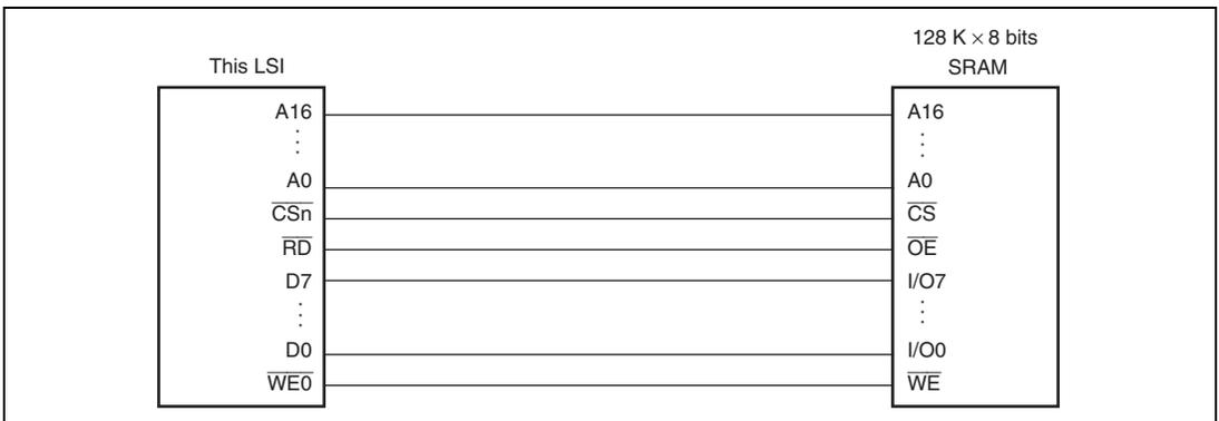
**Figure 11.8 Example of 8-Bit Data-Width SRAM Connection**
