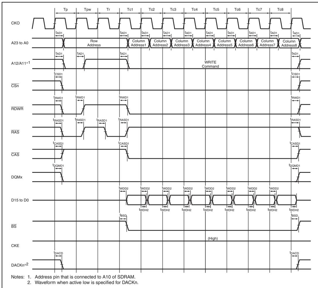
**Figure 33.29 Burst Write Bus Cycle of SDRAM (Single Write × 8)**
