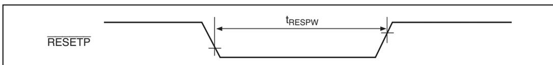
**Figure 33.4 Reset Input Timing**
