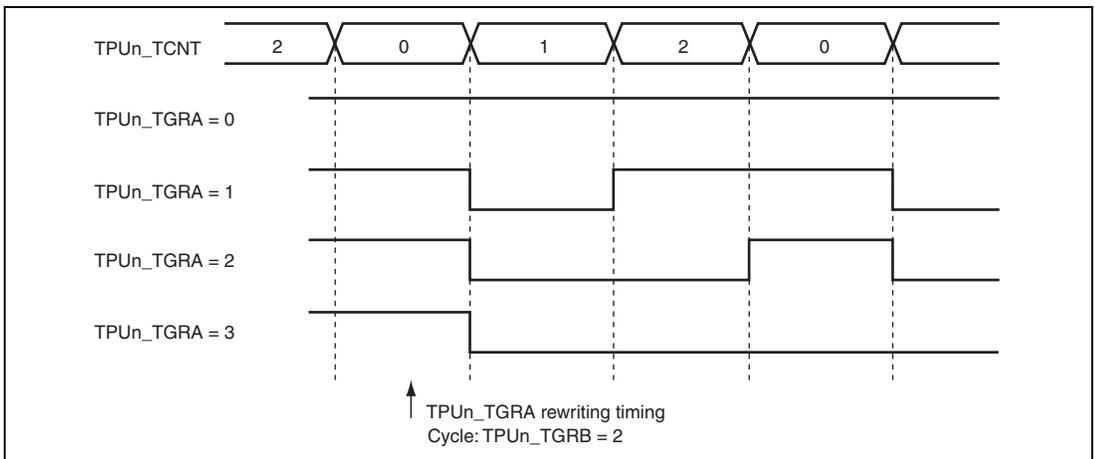
**Figure 16.13 Example of PWM Mode Operation (2)**
