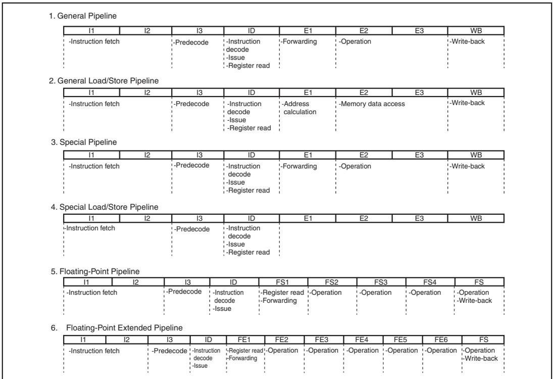
**Figure 4.1 Basic Pipelines**
