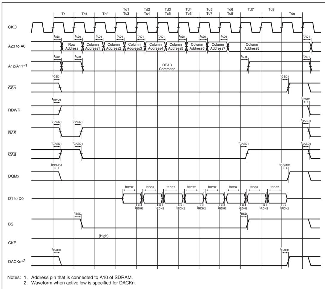
**Figure 33.24 Burst Read Bus Cycle of SDRAM (Single Read × 8)**
