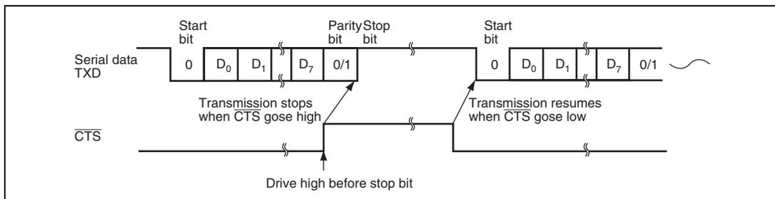
**Figure 22.6 Example of Operation Using Modem Control ( $\overline{\text{CTS}}$ )**
