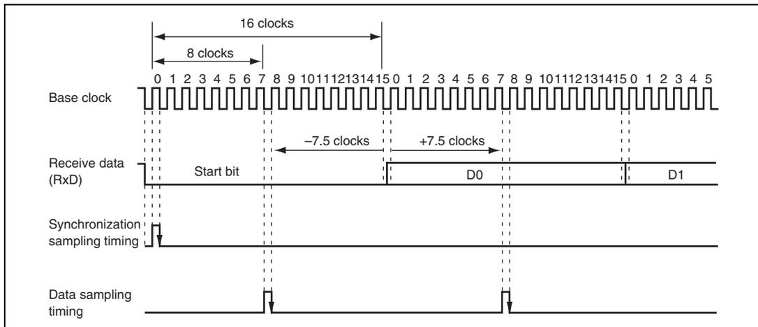
**Figure 22.19 Receive Data Sampling Timing in Asynchronous Mode**
