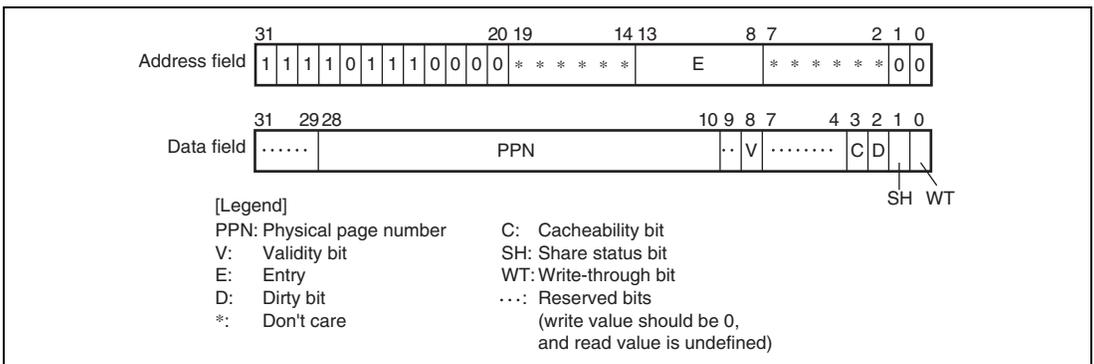
**Figure 7.24 Memory-Mapped UTLB Data Array 1 (TLB Extended Mode)**
