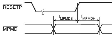
**Figure 33.58  $\overline{MPMD}$  Input Timing**
