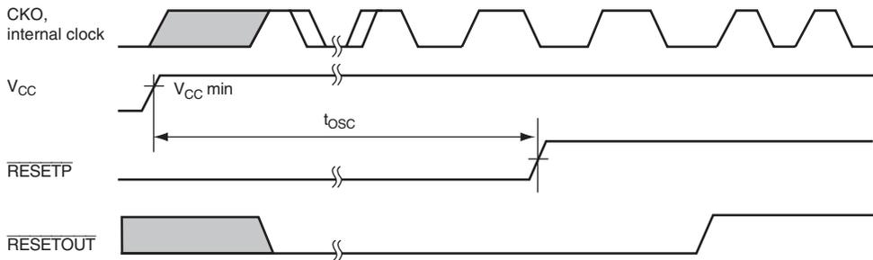
Note: Oscillation settling time when on-chip oscillator is used
