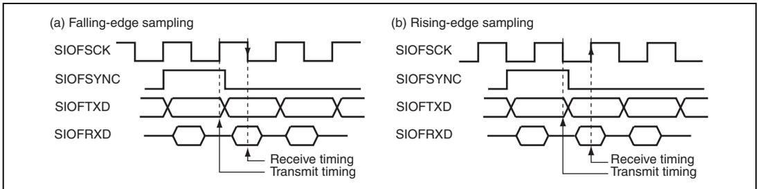
**Figure 21.4 SIOF Transmit/Receive Timing**
