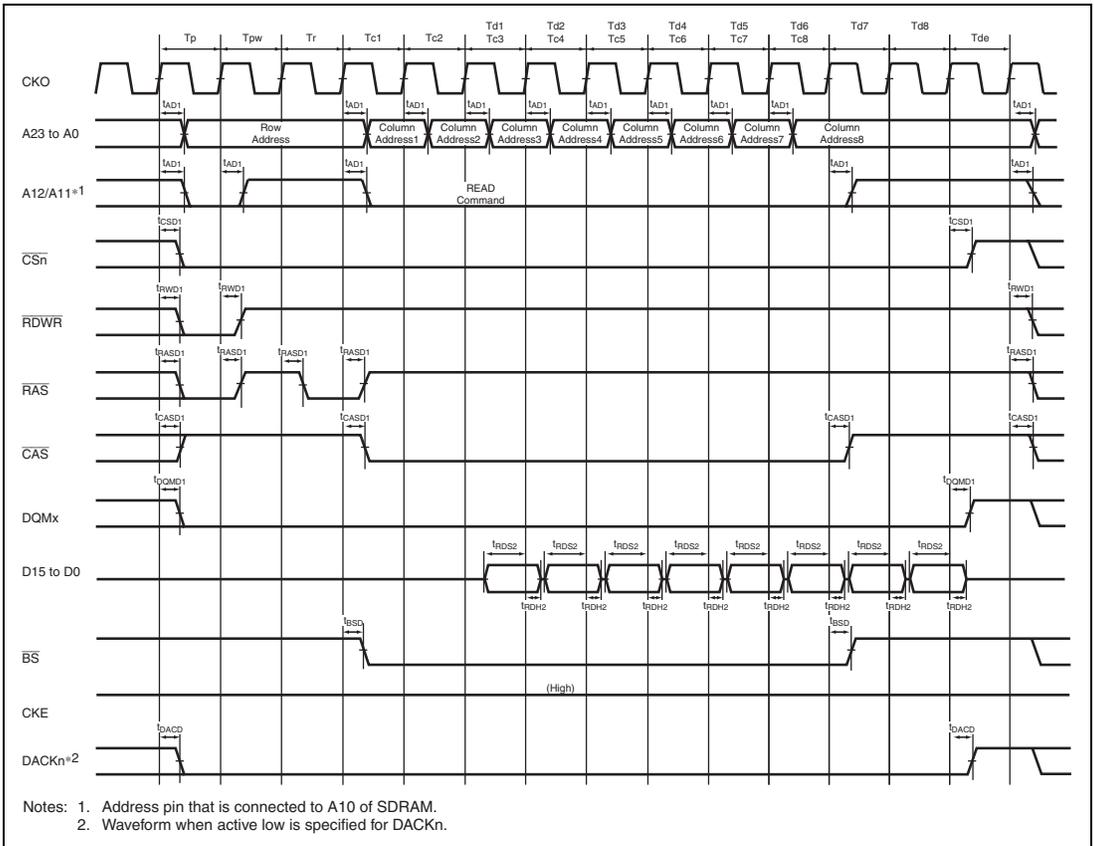
**Figure 33.26 Burst Read Bus Cycle of SDRAM (Single Read × 8)**
