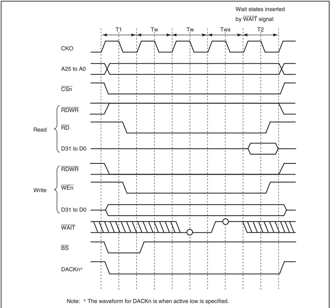
**Figure 11.10 Wait State Timing for Normal Space Access
