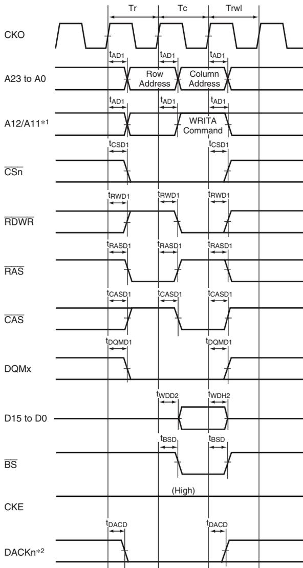
Notes: 1. Address pin that is connected to A10 of SDRAM.
