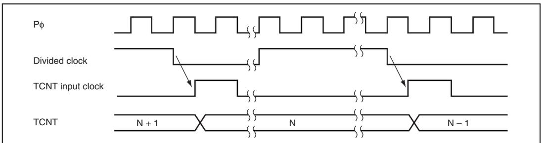
**Figure 18.4 Count Timing when Internal Clock is Operating**
