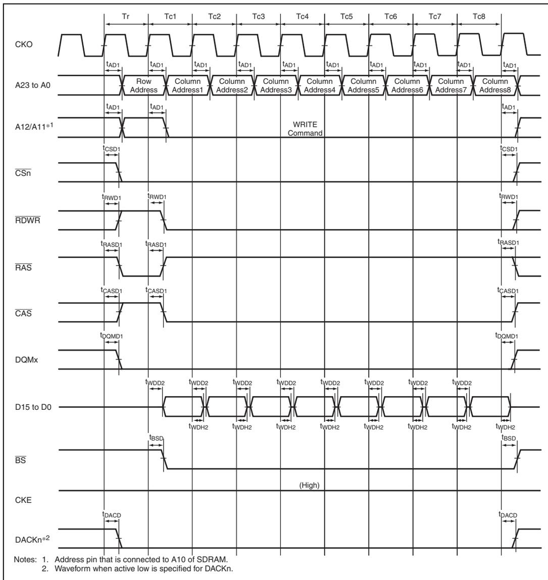
**Figure 33.27 Burst Write Bus Cycle of SDRAM (Single Write × 8)
