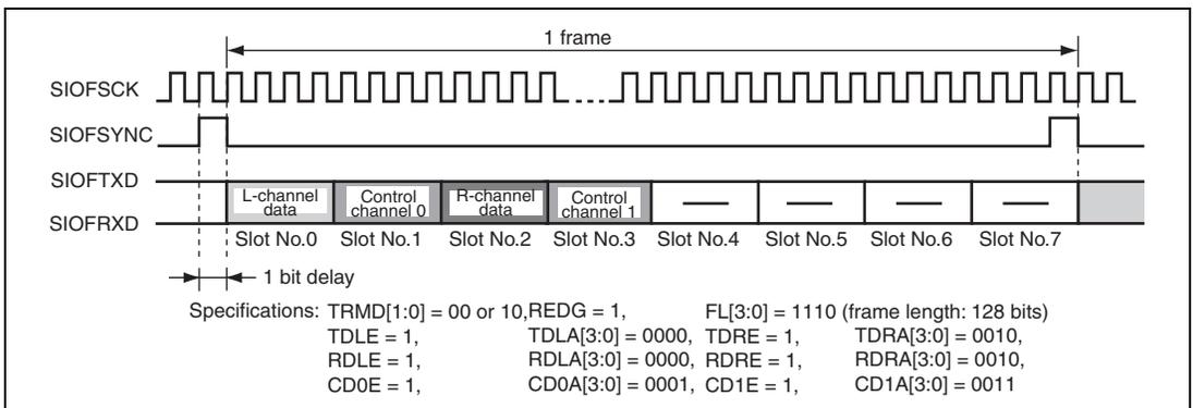
**Figure 21.19 Transmit and Receive Timing (16-Bit Stereo Data (4))**
