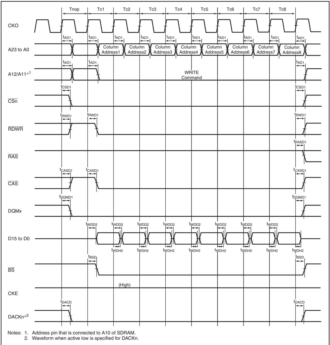
**Figure 33.28 Burst Write Bus Cycle of SDRAM (Single Write × 8)
