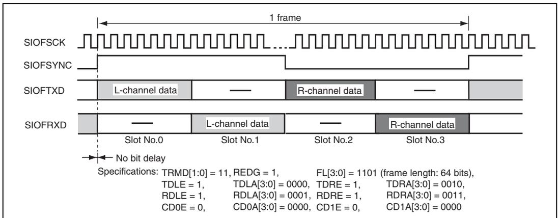
**Figure 21.17 Transmit and Receive Timing (16-Bit Stereo Data (2))**
