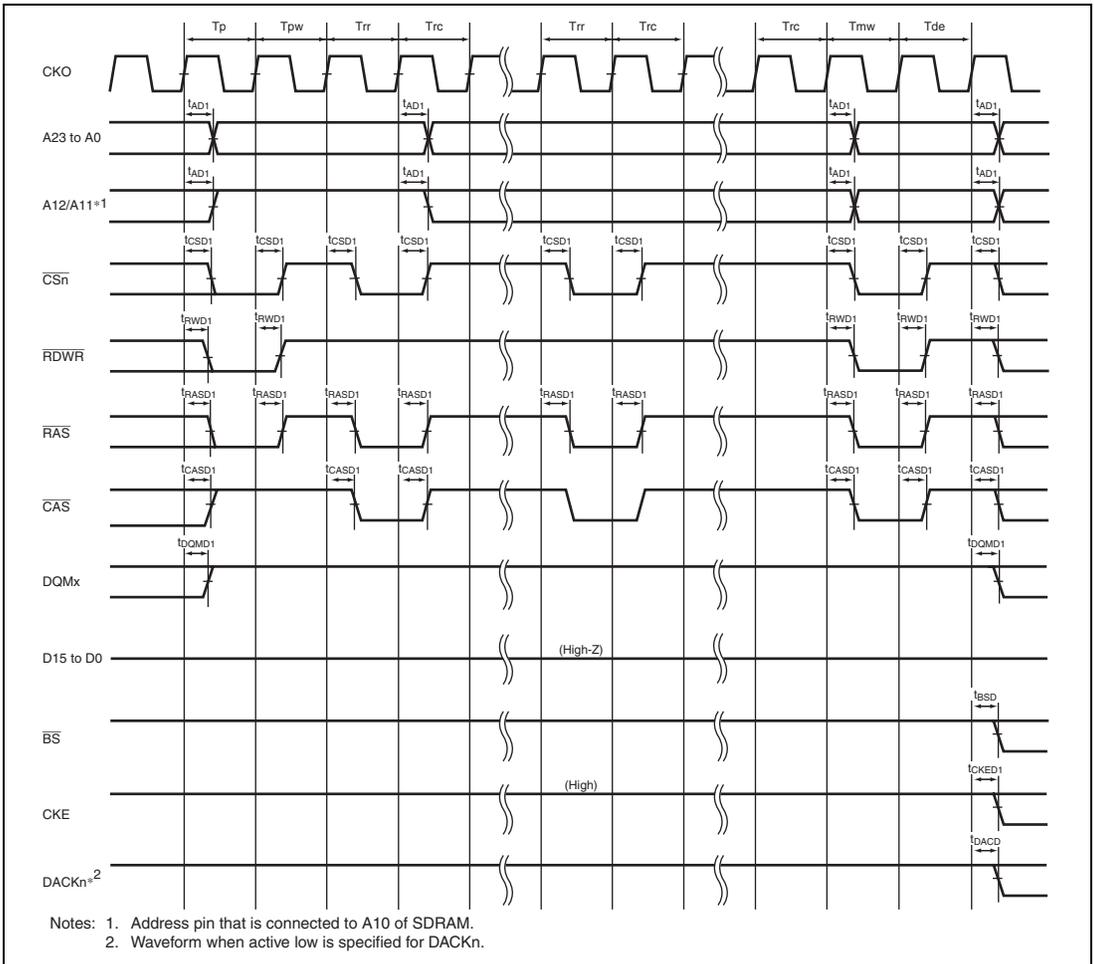
**Figure 33.32 Power-On Sequence of SDRAM
