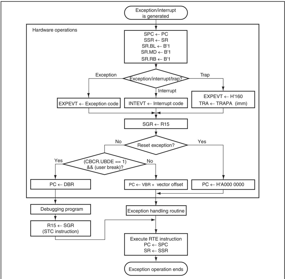
**Figure 30.2 Flowchart of User Break Debugging Support Function**
