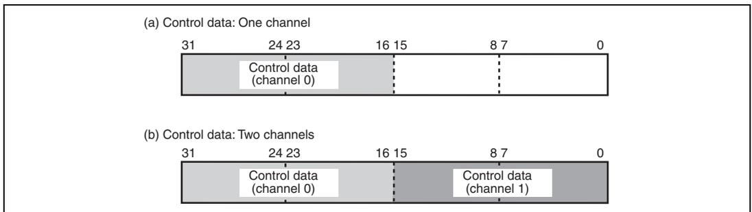
**Figure 21.6 Control Data Bit Alignment**
