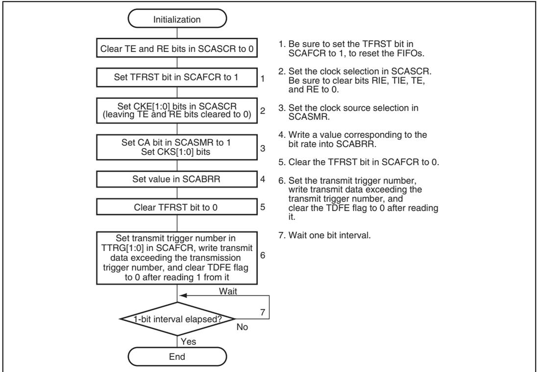
**Figure 23.13 Sample SCIFA Initialization Flowchart (1) (Transmission)**
