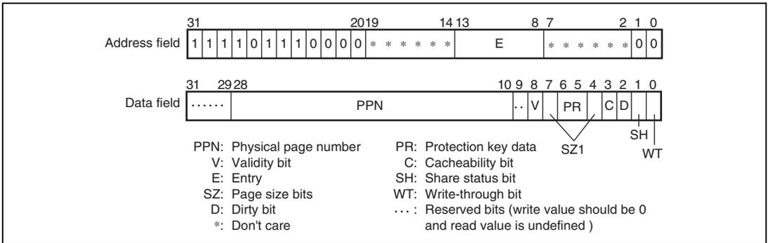
**Figure 7.23 Memory-Mapped UTLB Data Array (TLB Compatible Mode)**
