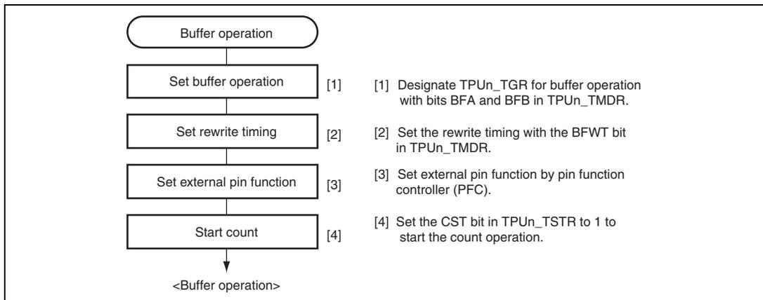
**Figure 16.9 Example of Buffer Operation Setting Procedure**
