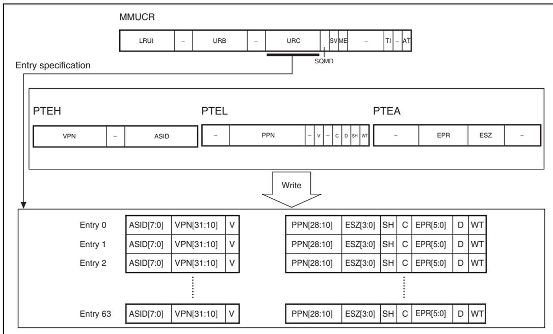
**Figure 7.17 Operation of LDTLB Instruction (TLB Extended Mode)**
