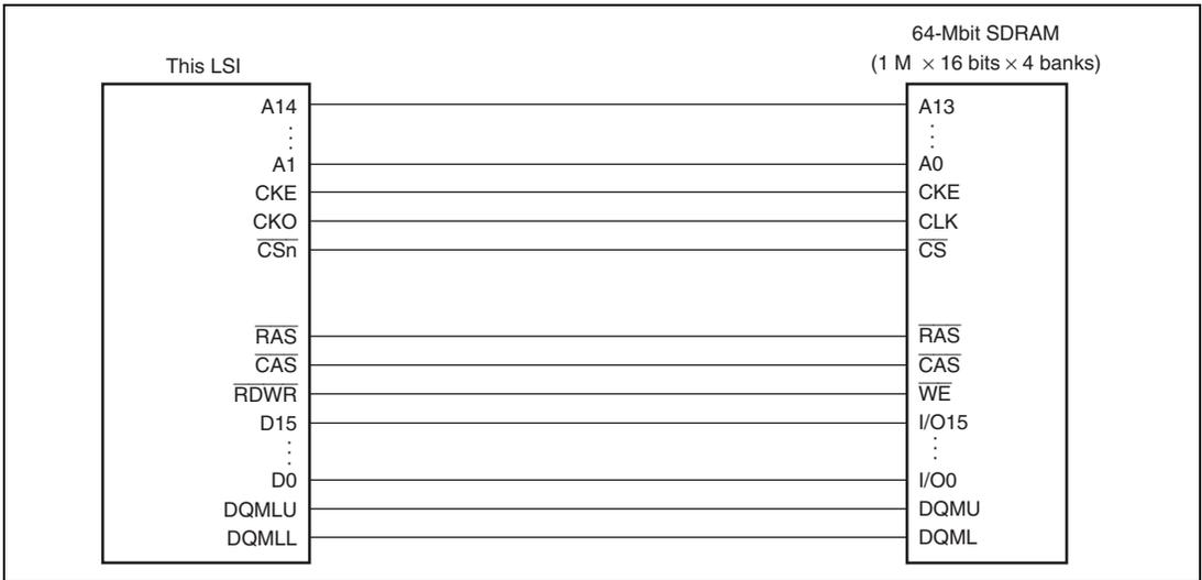
**Figure 11.13 Example of 16-Bit Data-Width SDRAM Connection**
