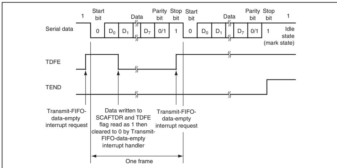
**Figure 23.4 Example of Transmit Operation
