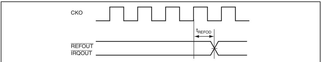
**Figure 33.39 REFOUT, IRQOUT Delay Time**
