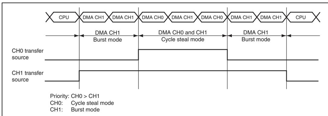
**Figure 12.9 Bus State when Multiple Channels are Operating**
