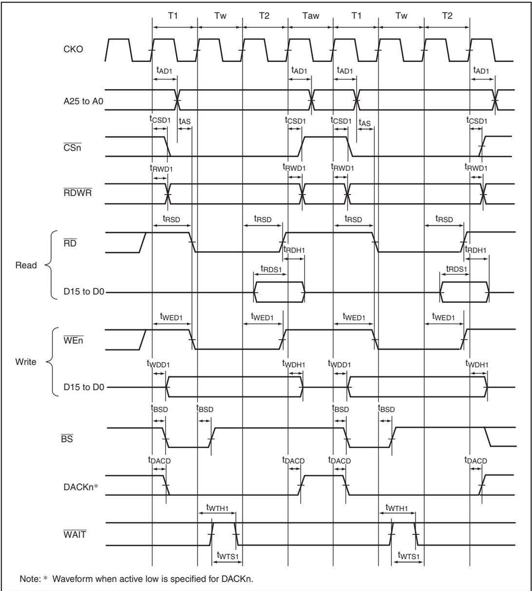
**Figure 33.11 Basic Bus Cycle in Normal Space**
