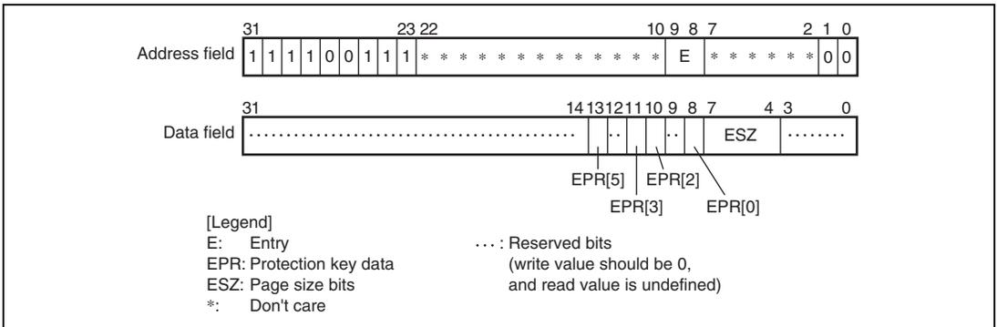
**Figure 7.21 Memory-Mapped ITLB Data Array 2 (TLB Extended Mode)**
