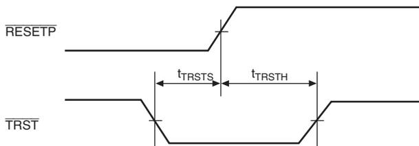
Figure 33.56 TRST Input Timing (Reset Hold)
