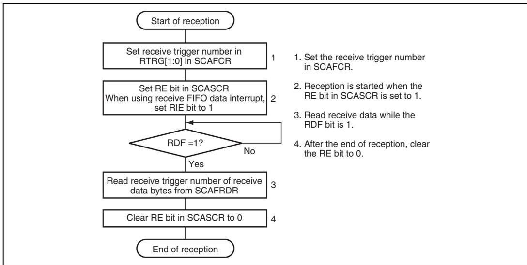
**Figure 23.18 Sample Serial Reception Flowchart (1)
