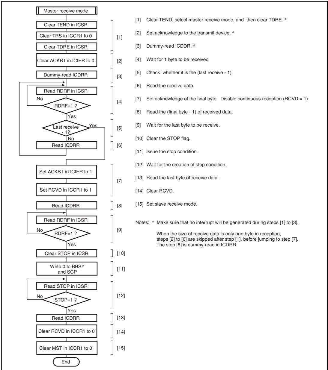
**Figure 20.15 Sample Flowchart for Master Receive Mode**
