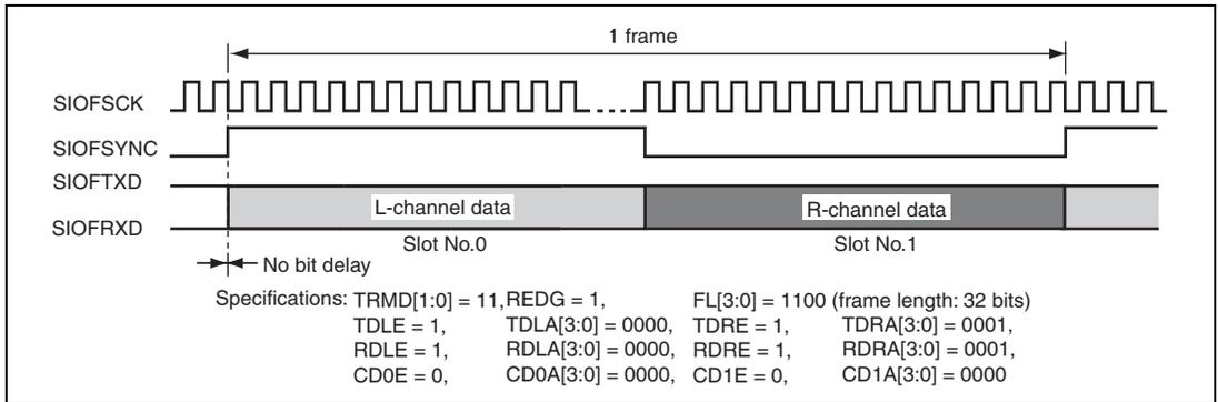
**Figure 21.16 Transmit and Receive Timing (16-Bit Stereo Data (1))**
