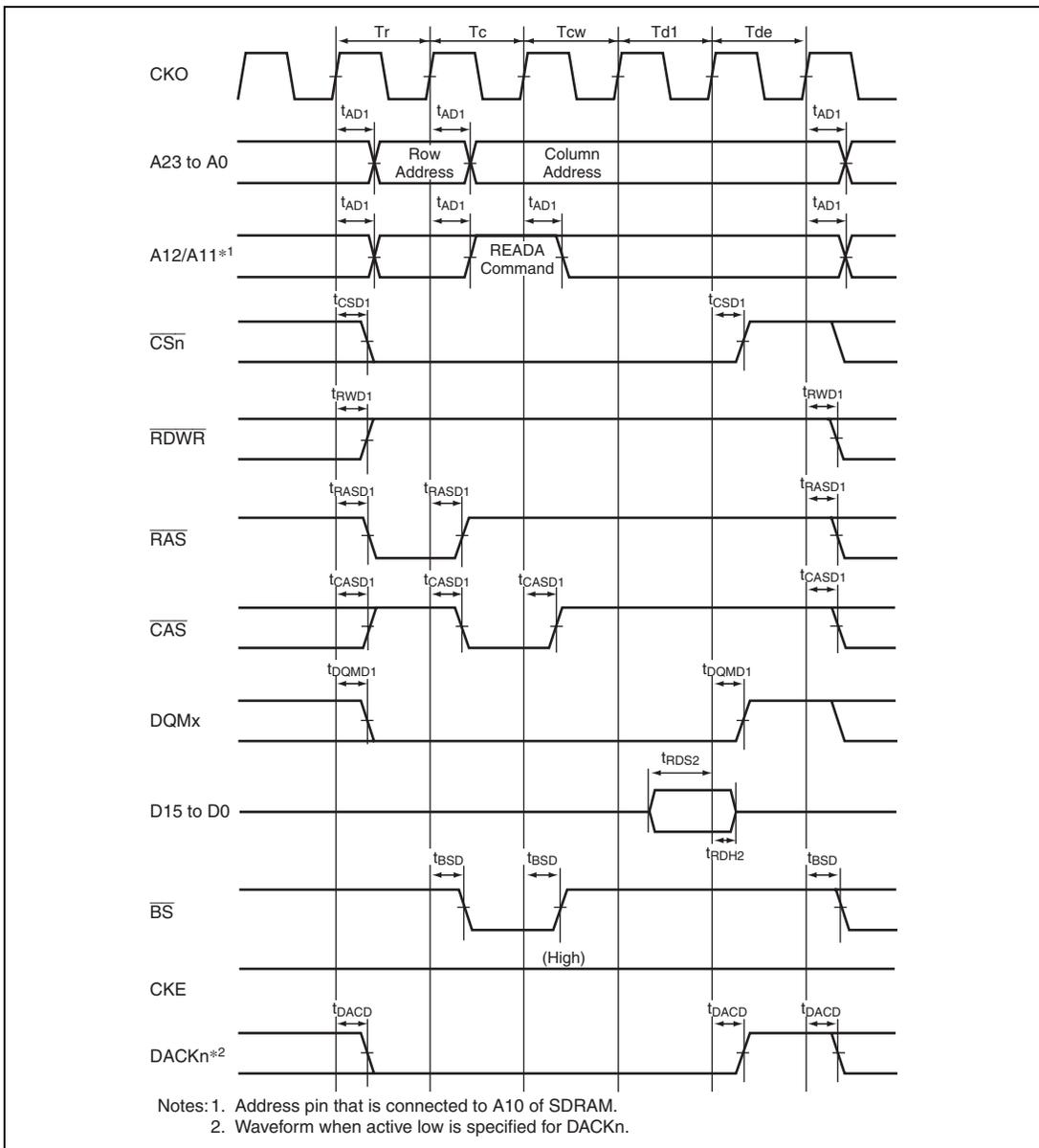
**Figure 33.16 Single Read Bus Cycle of SDRAM**
