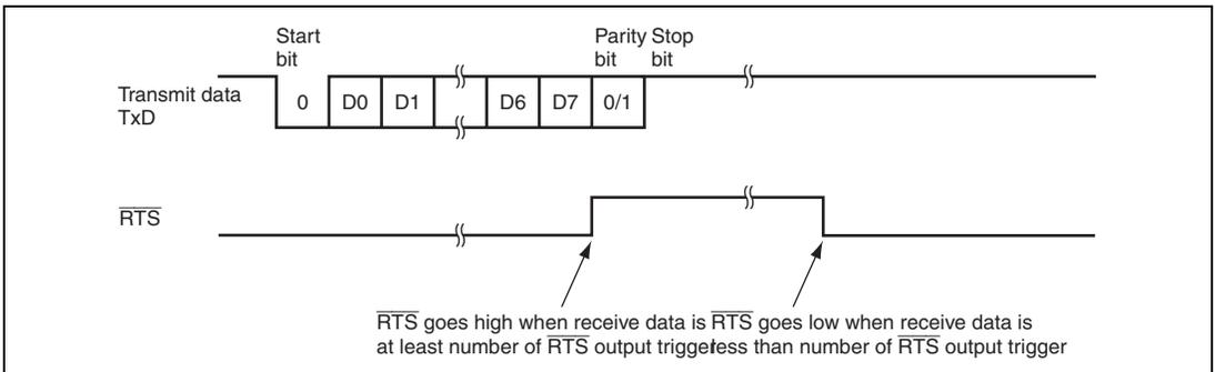
**Figure 23.11 Example of  $\overline{\text{RTS}}$  Control Operation**
