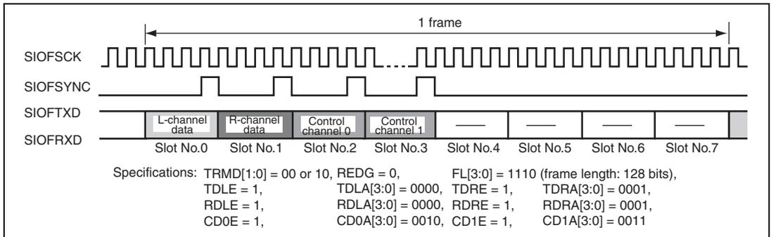
**Figure 21.20 Transmit and Receive Timing (16-Bit Stereo Data)**
