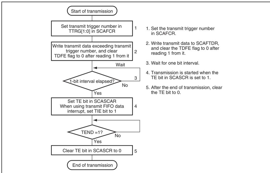
**Figure 23.17 Sample Serial Transmission Flowchart (2)
