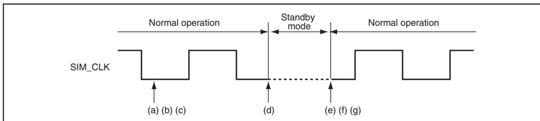
**Figure 25.11 Procedure for Stopping Clock and Restarting**
