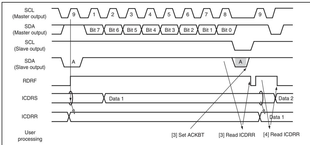
**Figure 20.12 Slave Receive Mode Operation Timing (2)**
