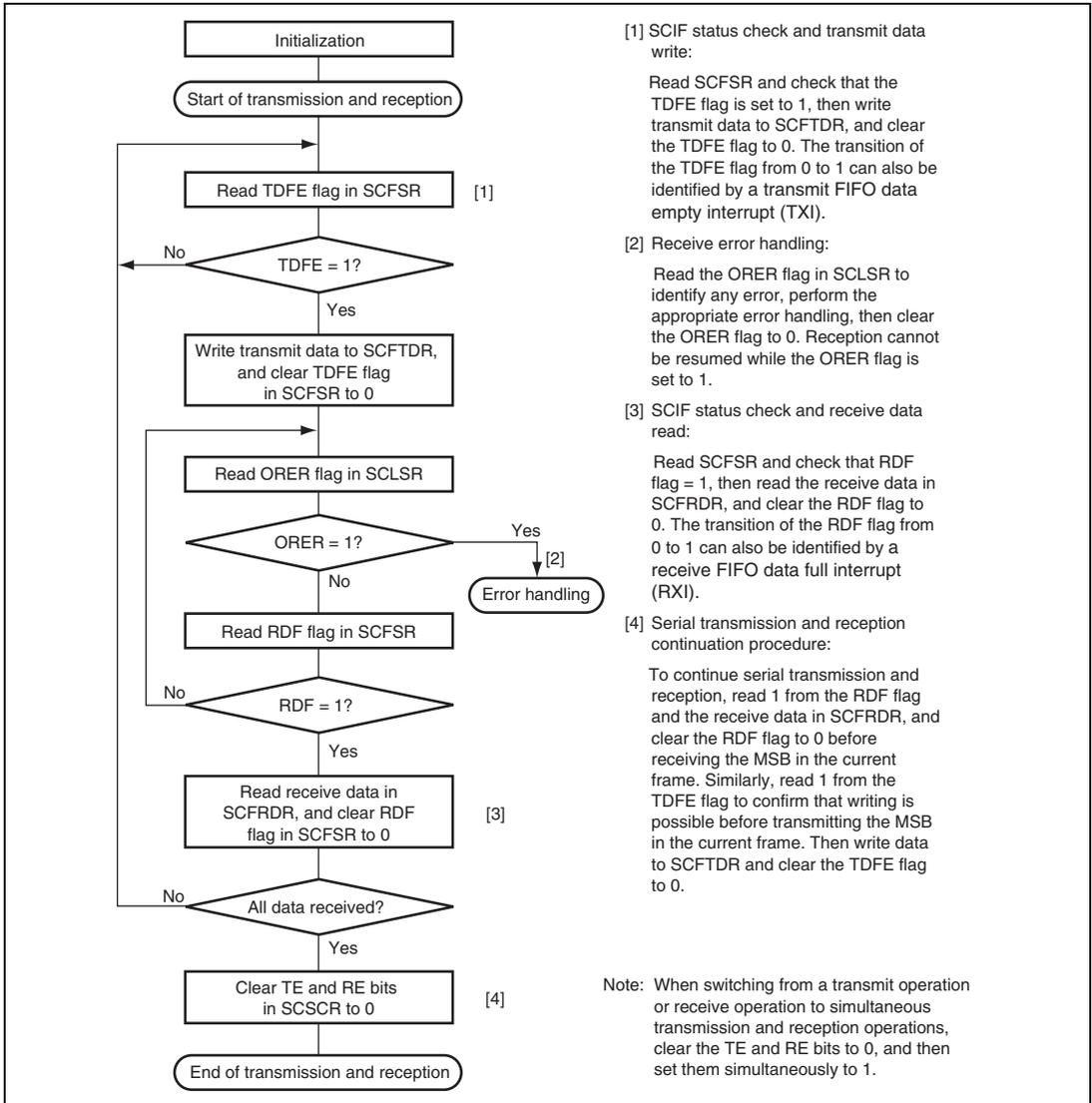
**Figure 22.18 Sample Flowchart for Transmitting/Receiving Serial Data**
