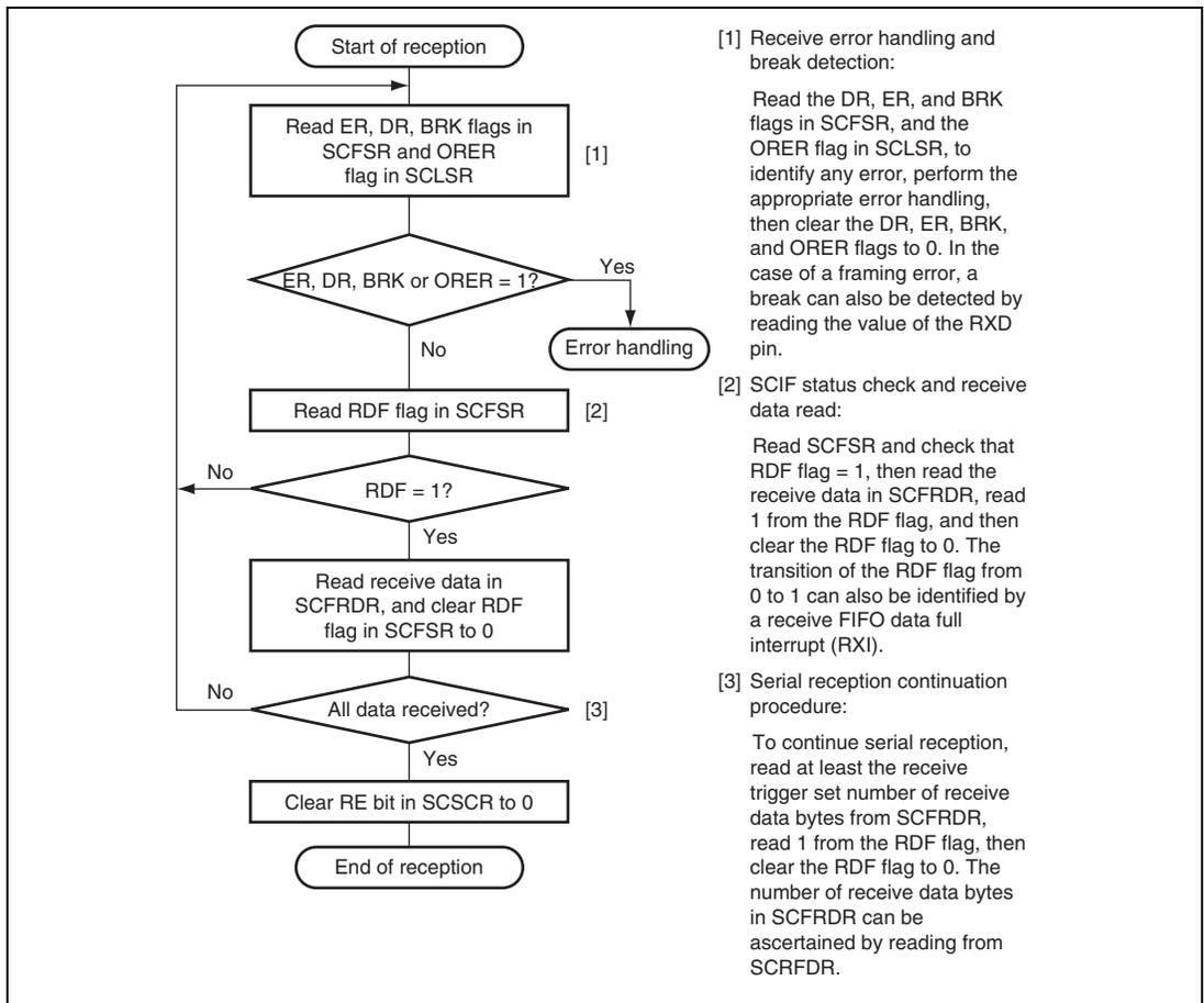
**Figure 22.7 Sample Flowchart for Receiving Serial Data**
