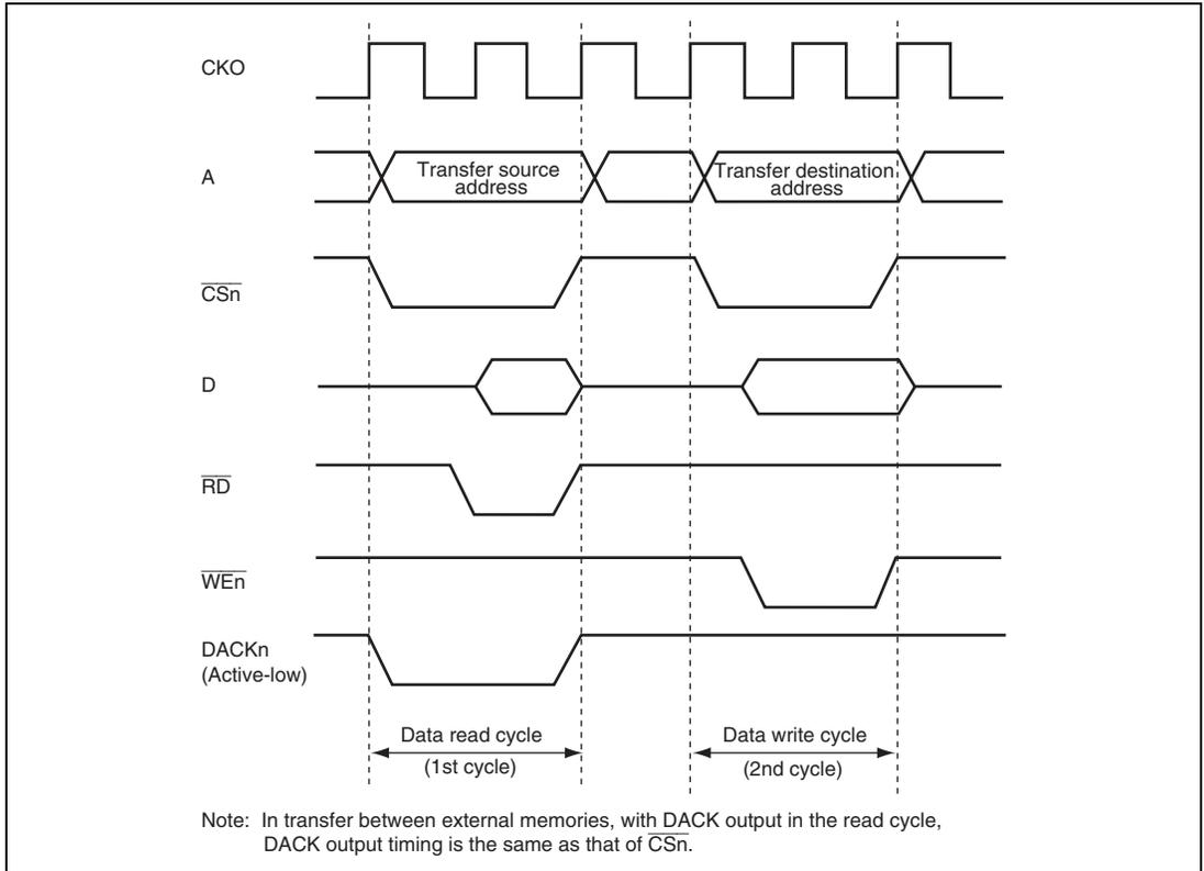
**Figure 12.5 Example of DMA Transfer Timing in Dual Mode
