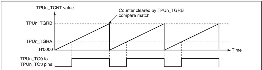
**Figure 16.12 Example of PWM Mode Operation (1)**
