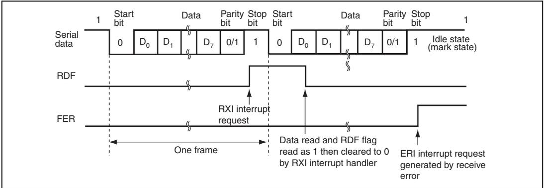
**Figure 22.9 Example of SCIF Receive Operation
