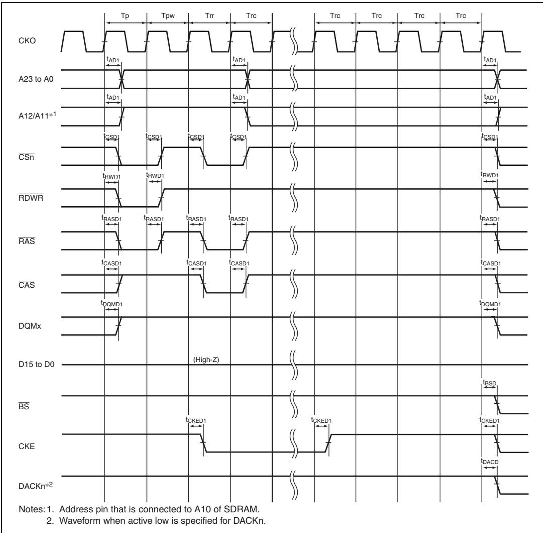
**Figure 33.31 Self Refresh Timing of SDRAM (TRP = 2 Cycles)**
