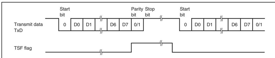
**Figure 23.5 Example of Transmit Data Stop Function**
