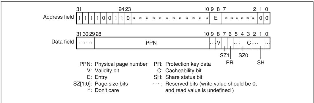
**Figure 7.19 Memory-Mapped ITLB Data Array (TLB Compatible Mode)**
