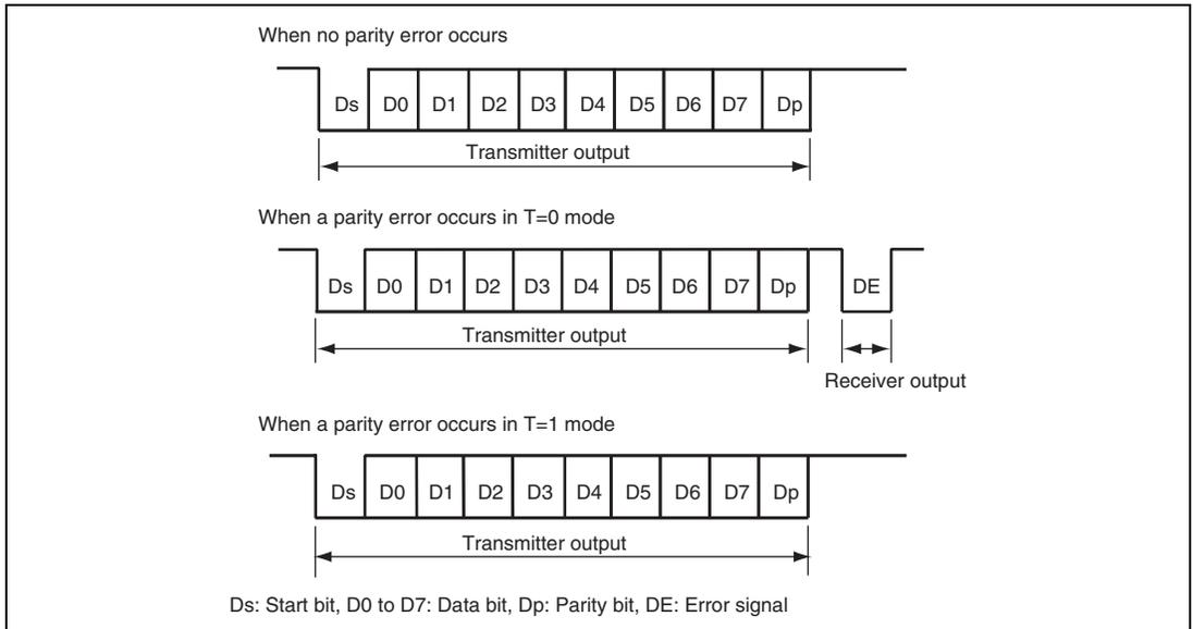
**Figure 25.2 Data Format Used by Smart Card Interface**
