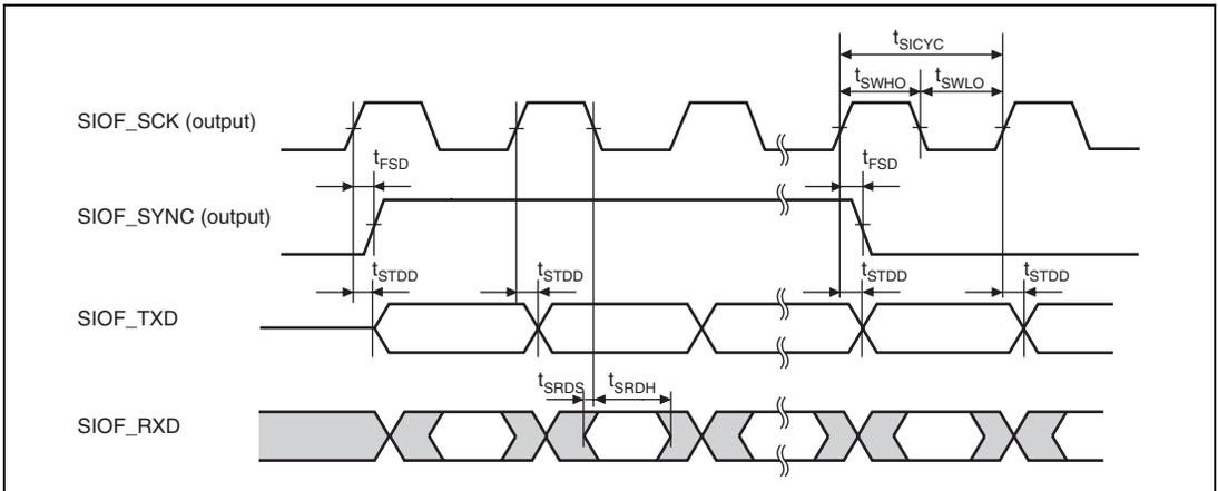
**Figure 33.49 SIOF Transmission/Reception Timing (Master Mode 2, Fall Sampling)**
