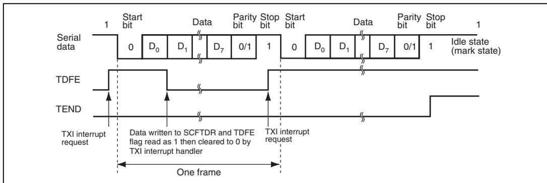
**Figure 22.5 Example of Transmit Operation
