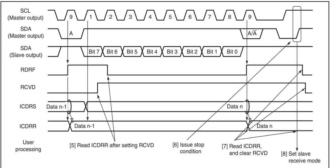
**Figure 20.8 Master Receive Mode Operation Timing (2)**
