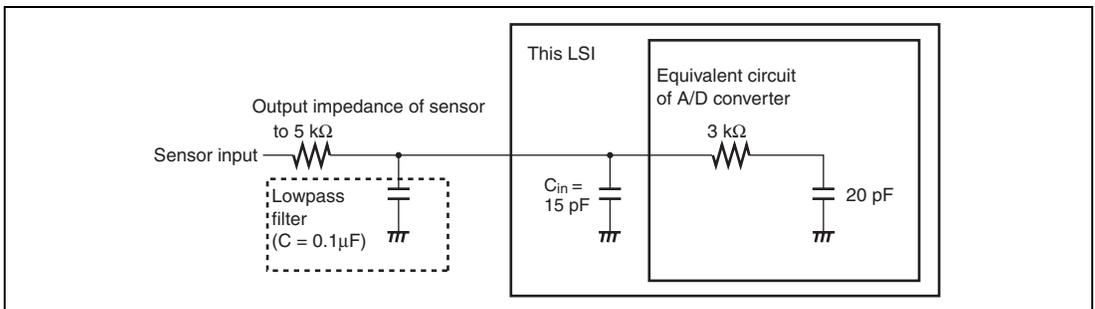
**Figure 26.8** Analog Input Circuit Example
