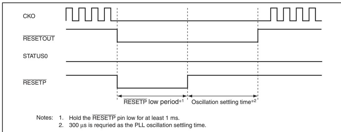
**Figure 14.2 State of Output Pins at Power-On Reset**
