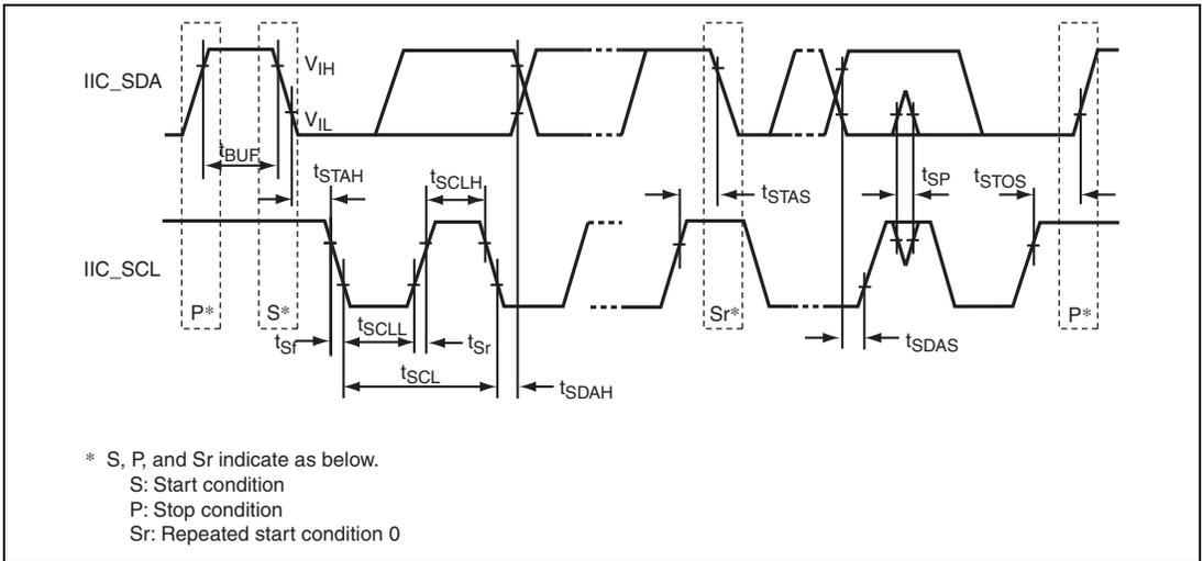
**Figure 33.45 I<sup>2</sup>C Bus Interface Input/Output Timing**
