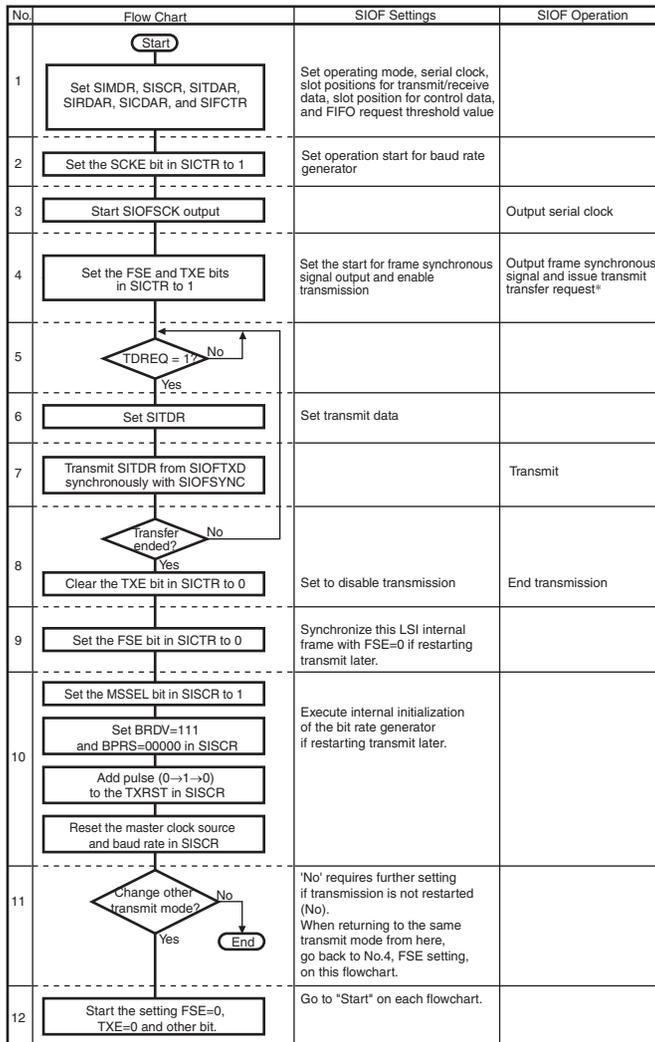
Note: \* When interrupts due to transmit data underflow are enabled, after setting the no. 6 transmit data, the TXE bit should be set to 1.
