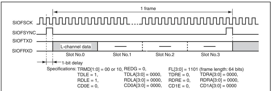
**Figure 21.15 Transmit and Receive Timing (16-Bit Monaural Data)**
