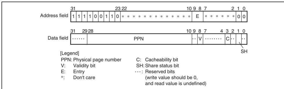
**Figure 7.20 Memory-Mapped ITLB Data Array 1 (TLB Extended Mode)**
