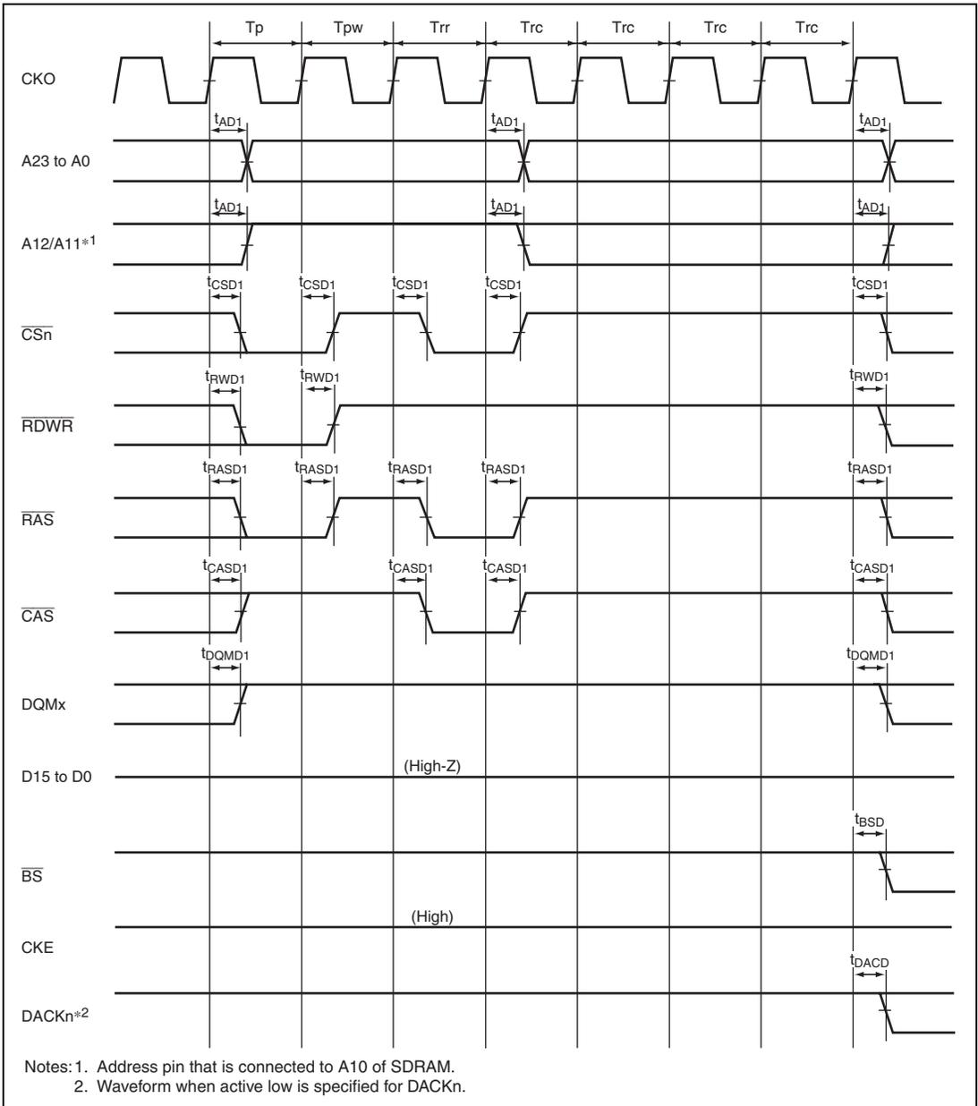
**Figure 33.30 Auto Refresh Timing of SDRAM (TRP = 2 Cycles)**
