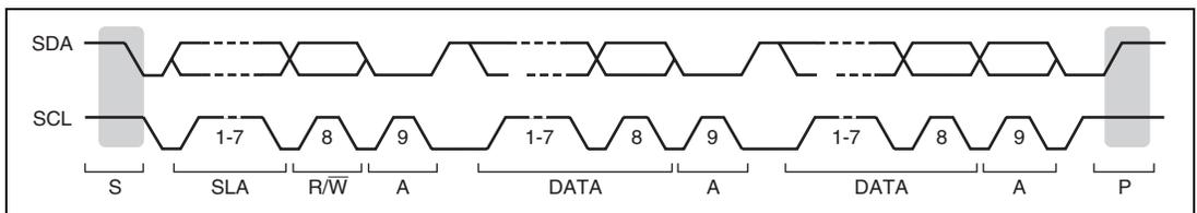
**Figure 20.4 I<sup>2</sup>C Bus Timing**
