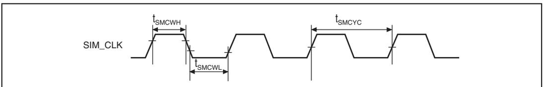
**Figure 33.54** SIM Module Signal Timing
