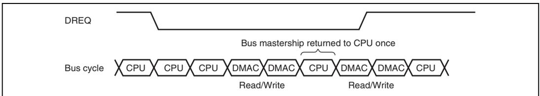
**Figure 12.6 DMA Transfer Example in Cycle-Steal Normal Mode
