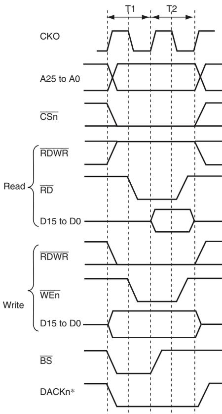
Note: \* The waveform for  $\overline{DACKn}$  is when active low is specified.
