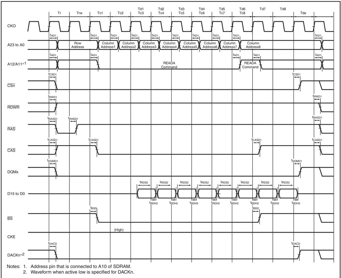
**Figure 33.19 Burst Read Bus Cycle of SDRAM (Single Read × 8)**
