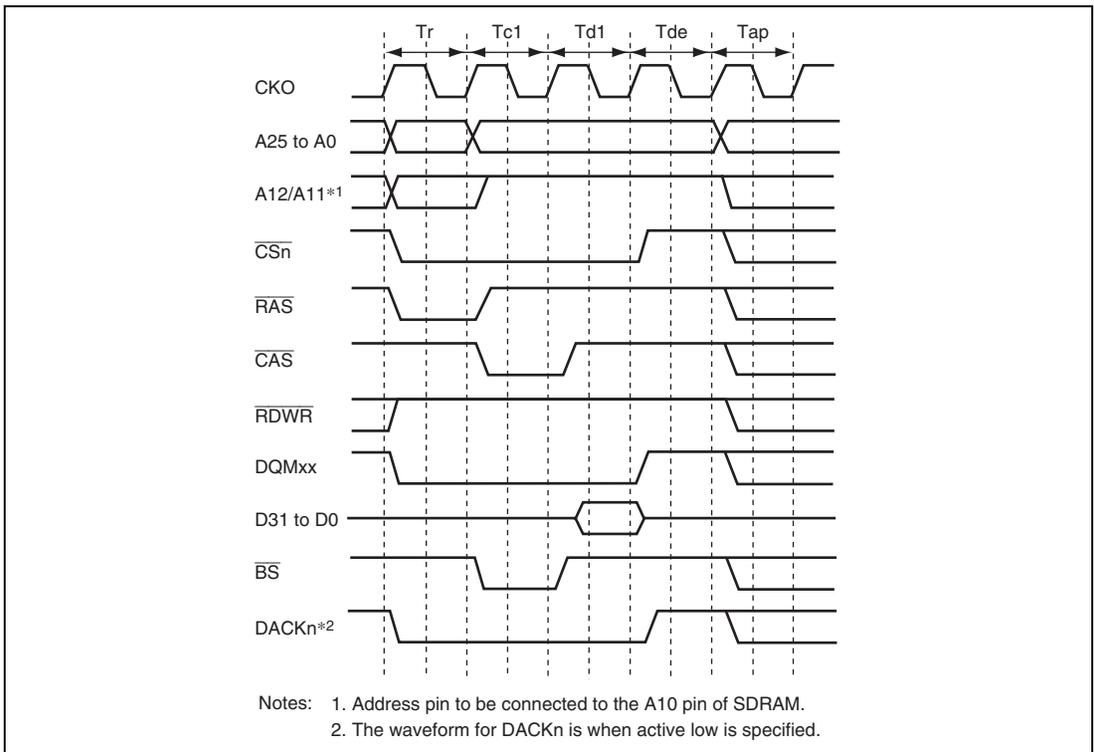
**Figure 11.16 Basic Timing for Single Read (Auto-Precharge)**
