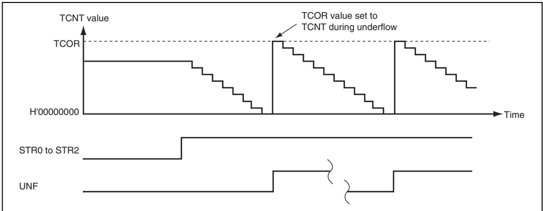
**Figure 18.3 Auto-Reload Count Operation**
