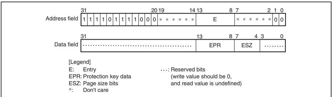
**Figure 7.25 Memory-Mapped UTLB Data Array 2 (TLB Extended Mode)**
