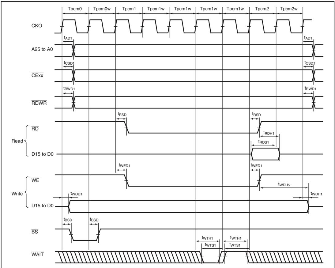
**Figure 33.36 PCMCIA Memory Card Interface Bus Timing**
