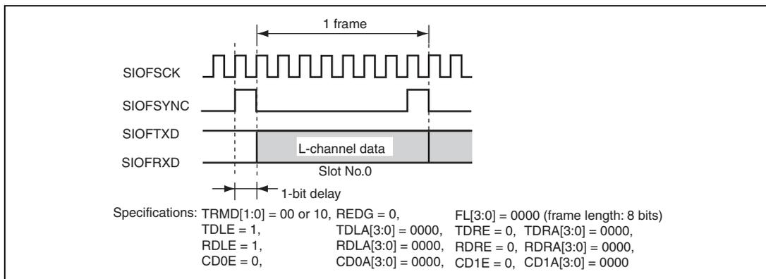
**Figure 21.13 Transmit and Receive Timing (8-Bit Monaural Data (1))**
