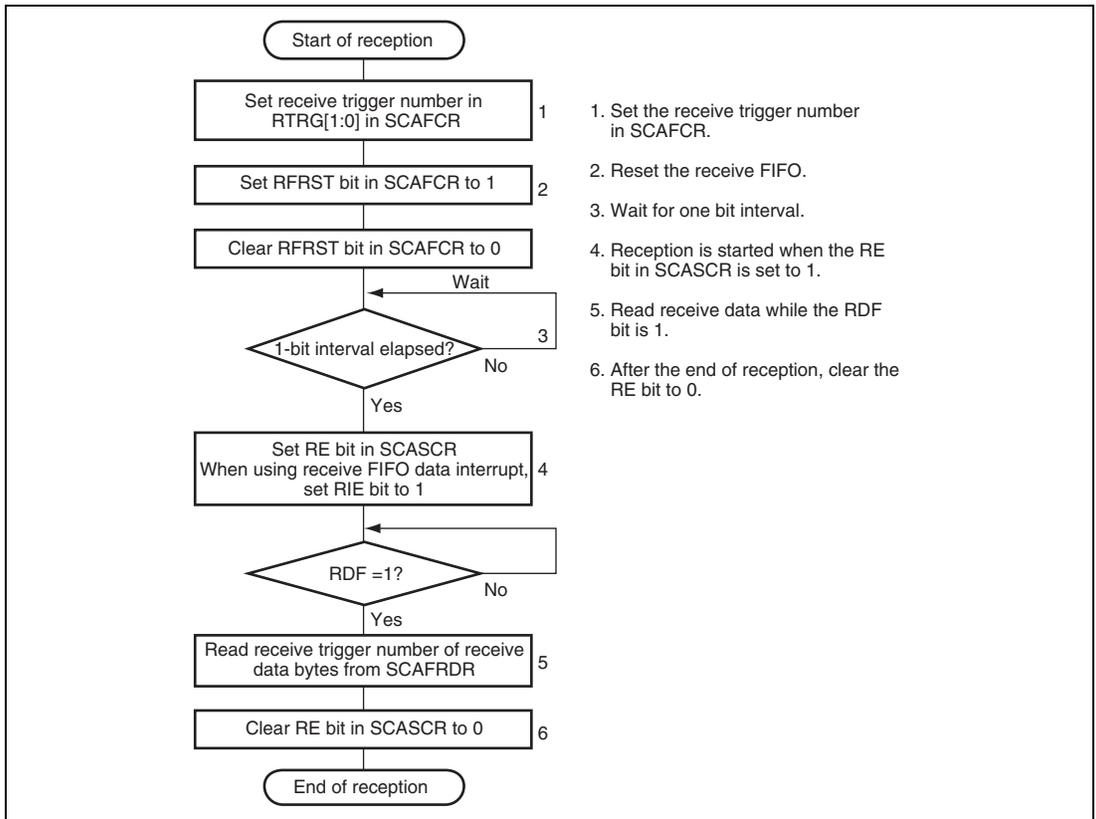
**Figure 23.19 Sample Serial Reception Flowchart (2)**
