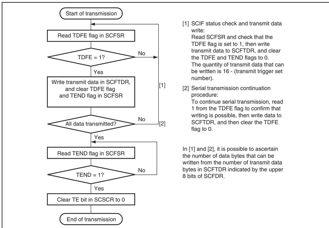
**Figure 22.4 Sample Flowchart for Transmitting Serial Data**
