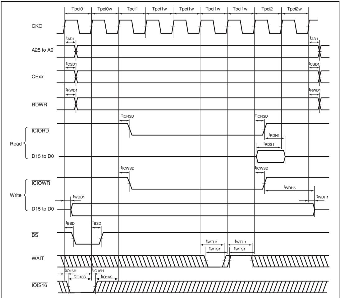
**Figure 33.38 PCMCIA I/O Card Interface Bus Timing**
