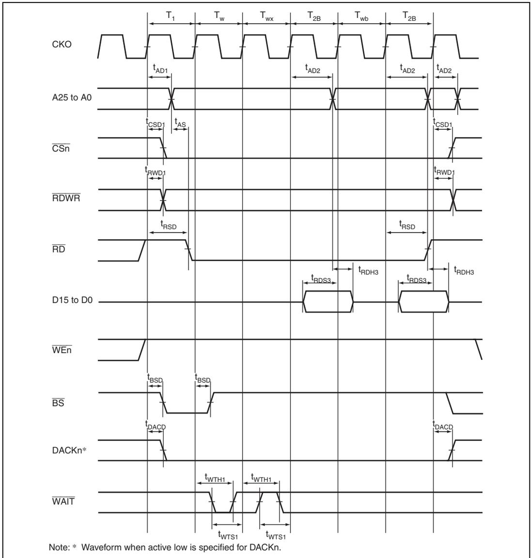
**Figure 33.15 Read Bus Cycle of Burst ROM**
