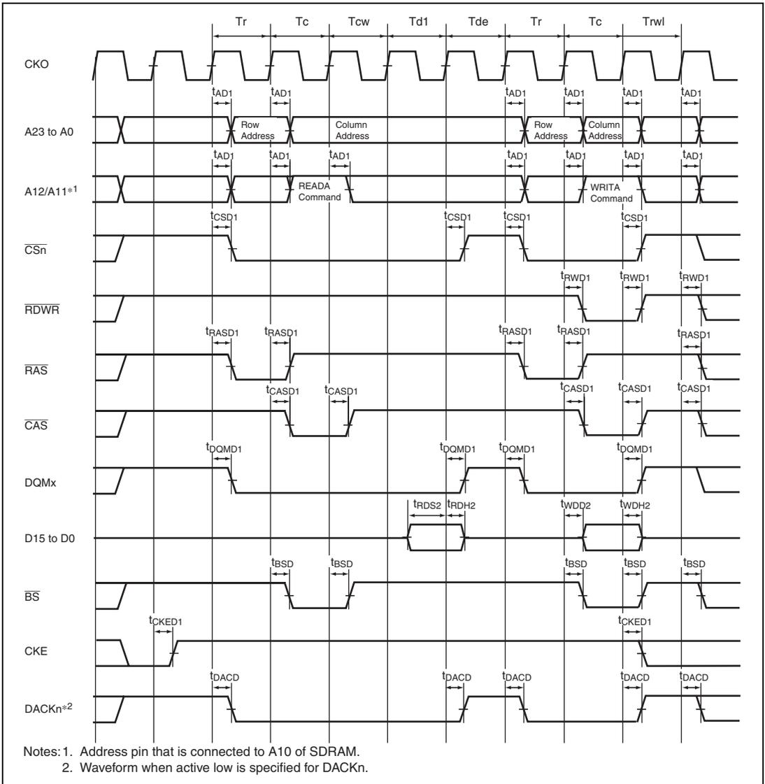
**Figure 33.34 Read-to-Write Bus Cycle in Power-Down Mode of SDRAM
