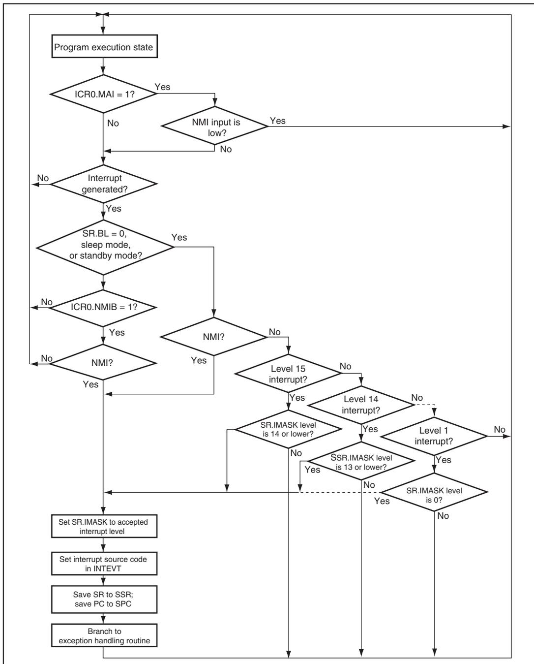
**Figure 10.4** Interrupt Operation Flowchart (when CPUOPM.INTMU = 1)
