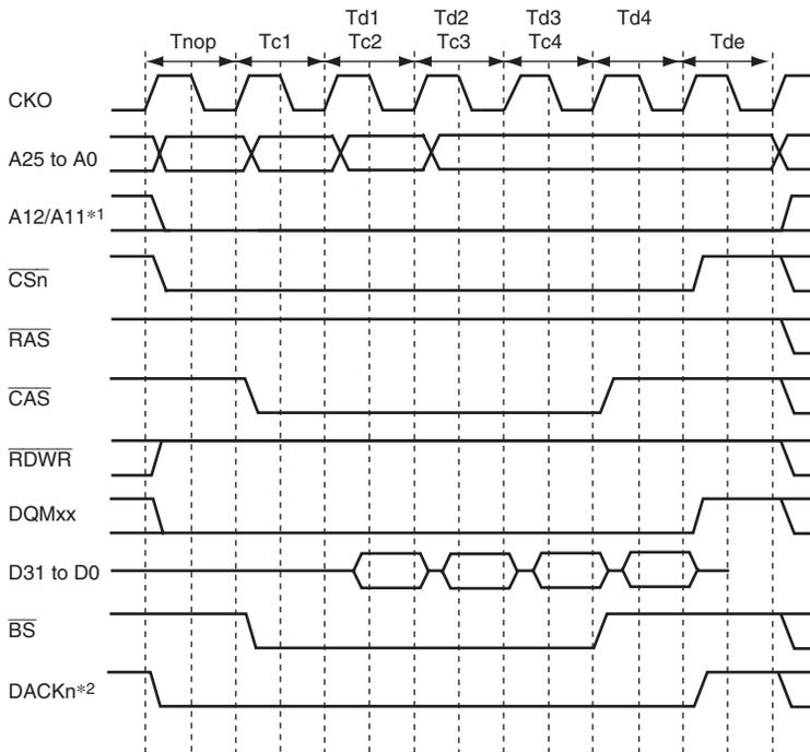
Notes: 1. Address pin to be connected to the A10 pin of SDRAM.
