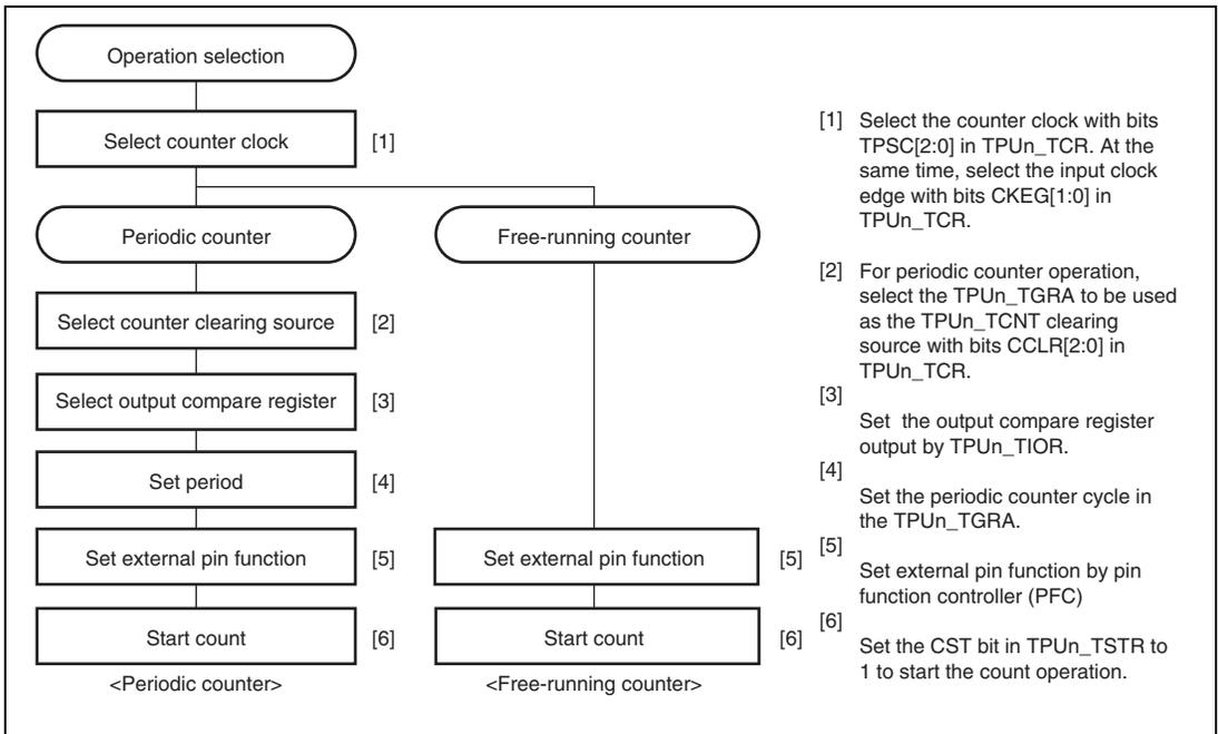
**Figure 16.2 Example of Counter Operation Setting Procedure**
