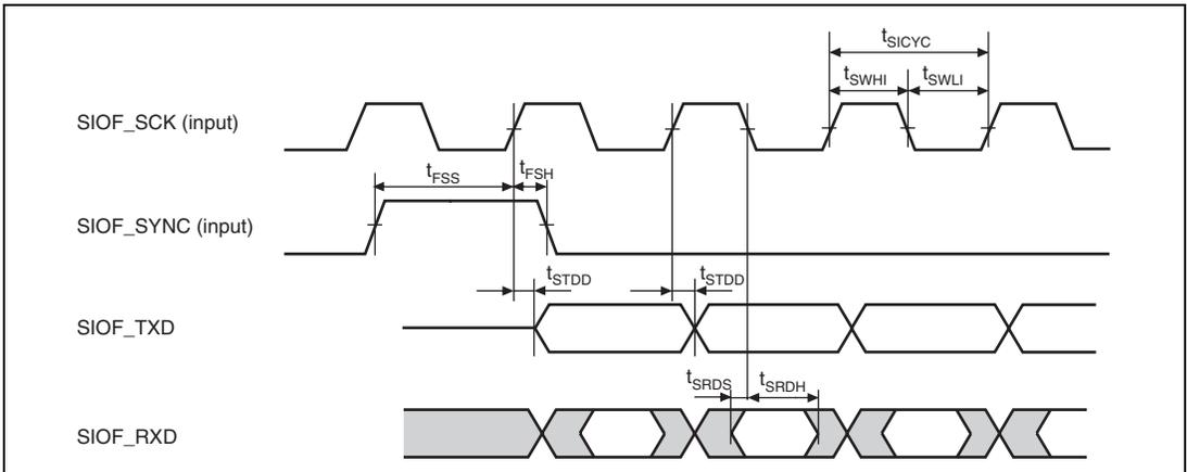
**Figure 33.51 SIOF Transmission/Reception Timing (Slave Mode 1, Slave Mode 2)**
