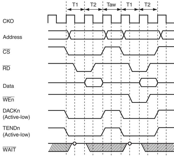
Note: TEND is asserted for the last transfer unit of the DMA transfer.
