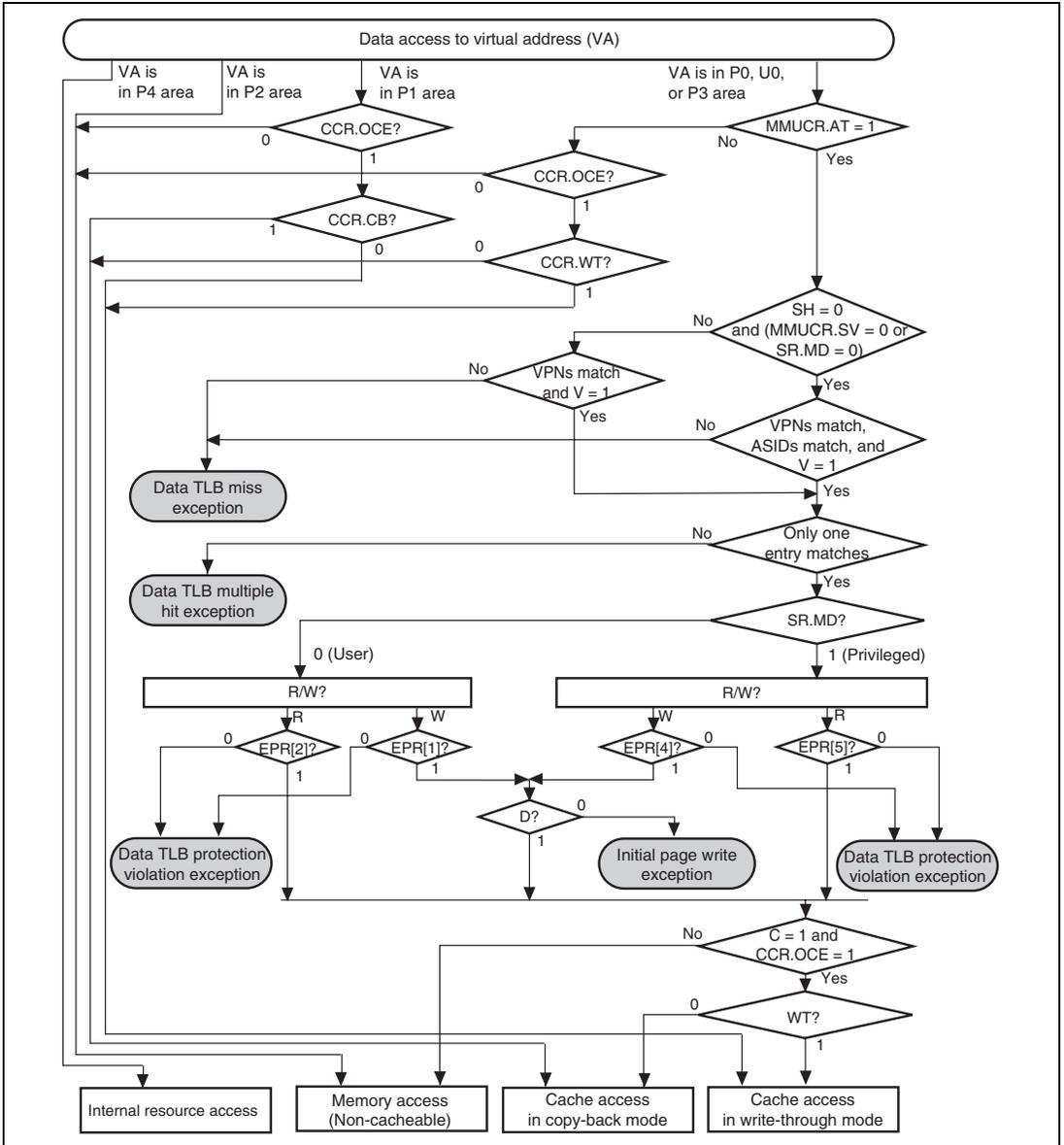
**Figure 7.14 Flowchart of Memory Access Using UTLB (TLB Extended Mode)**
