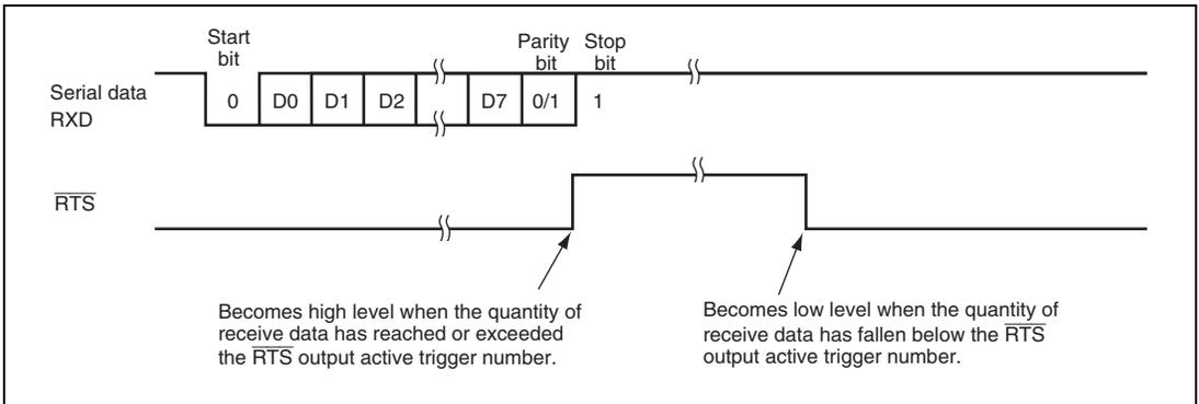
**Figure 22.10 Example of Operation Using Modem Control ( $\overline{\text{RTS}}$ )**
