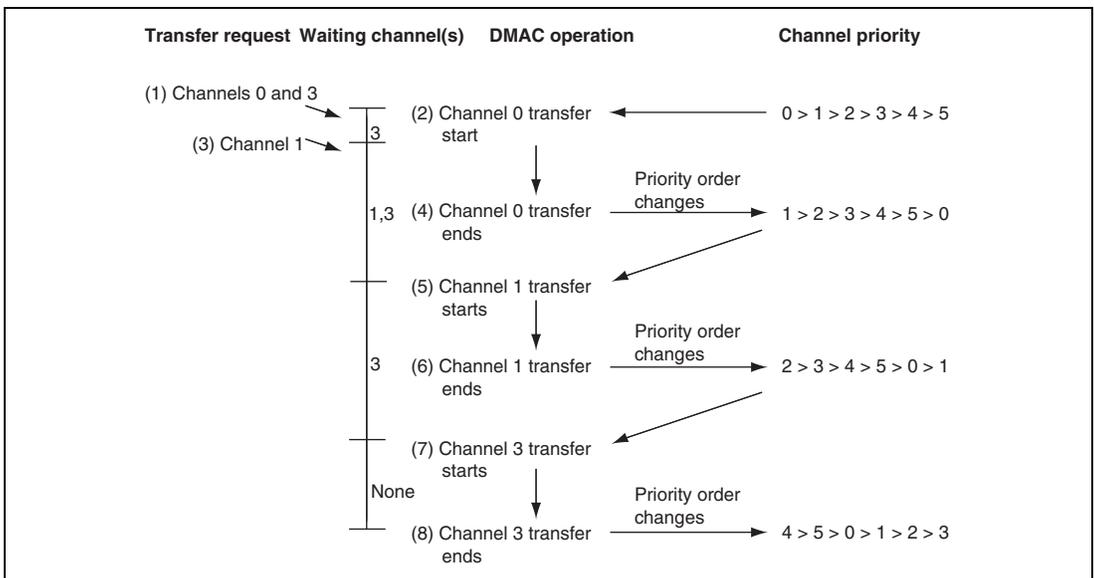
**Figure 12.3 Changes in Channel Priority in Round-Robin Mode**
