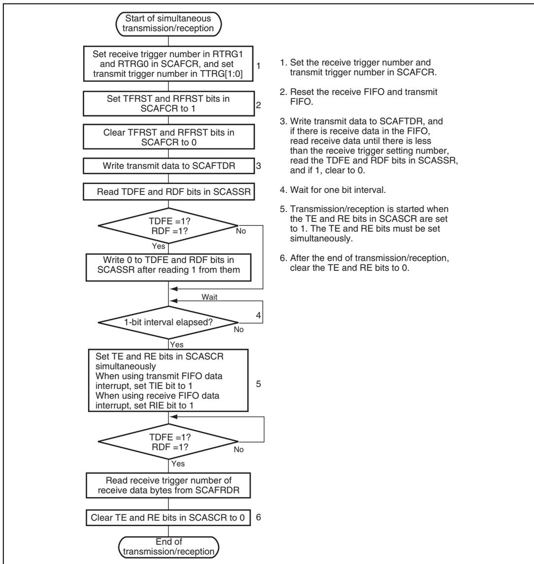
**Figure 23.21 Sample Simultaneous Serial Transmission and Reception Flowchart (2)
