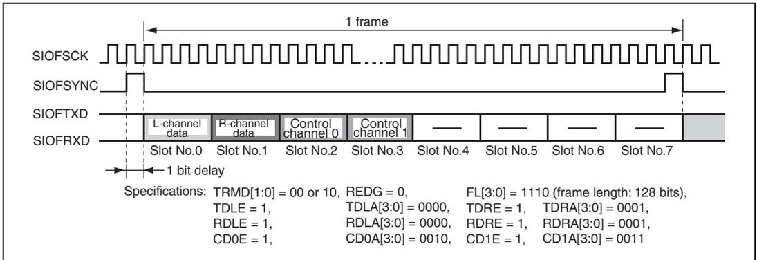
**Figure 21.18 Transmit and Receive Timing (16-Bit Stereo Data (3))**
