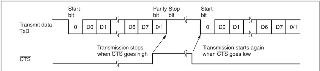
**Figure 23.10 Example of  $\overline{\text{CTS}}$  Control Operation**
