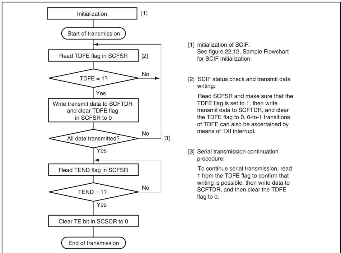
**Figure 22.13 Sample Flowchart for Transmitting Serial Data**
