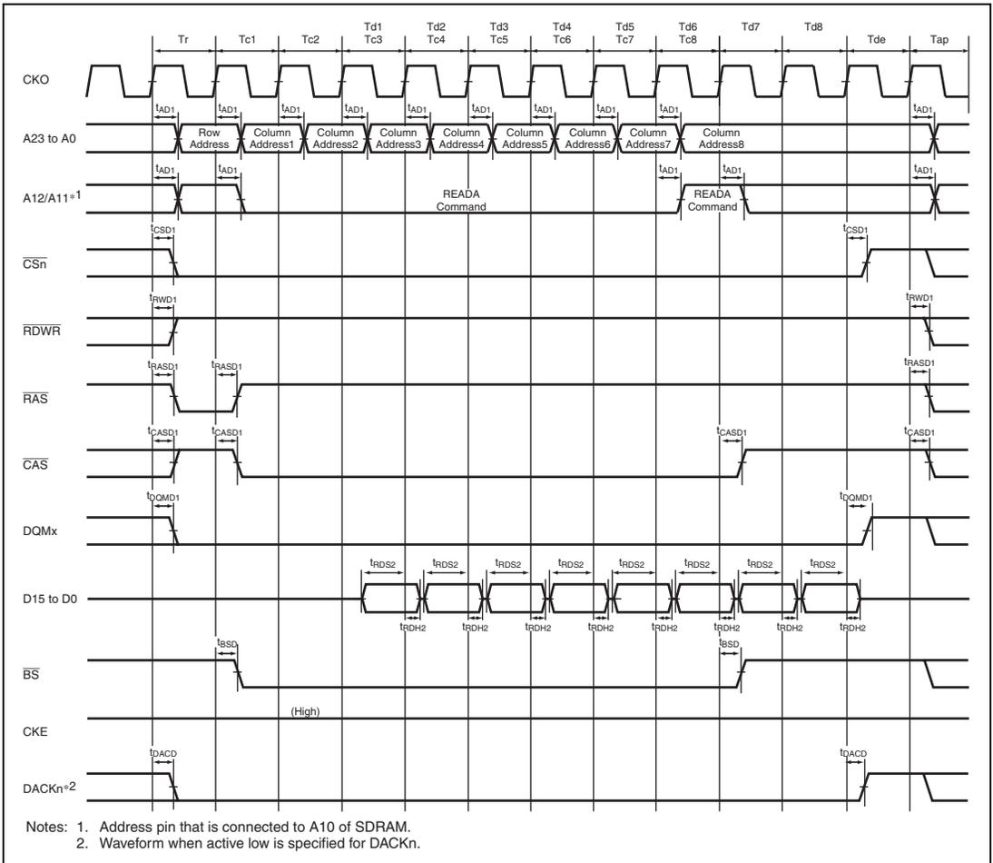
**Figure 33.18 Burst Read Bus Cycle of SDRAM (Single Read × 8)**
