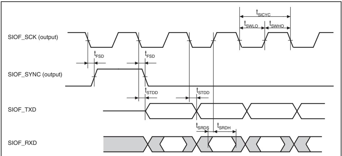
**Figure 33.48 SIOF Transmission/Reception Timing (Master Mode 1, Rise Sampling)**
