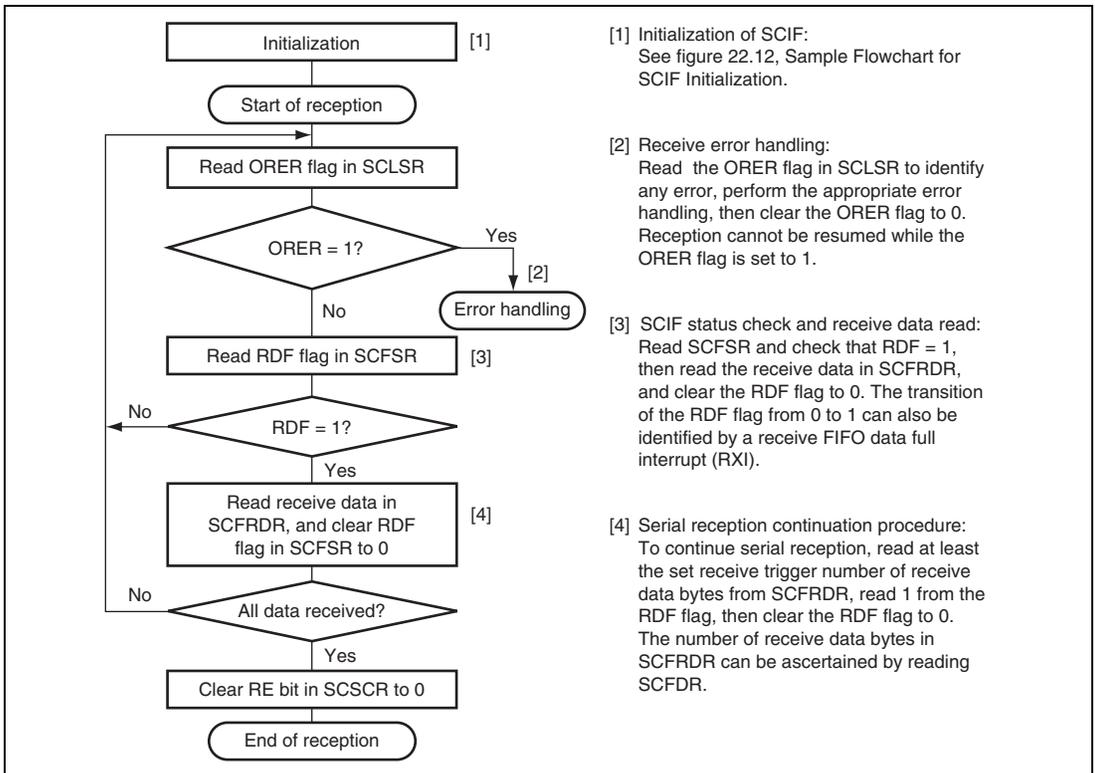
**Figure 22.15 Sample Flowchart for Receiving Serial Data (1)**
