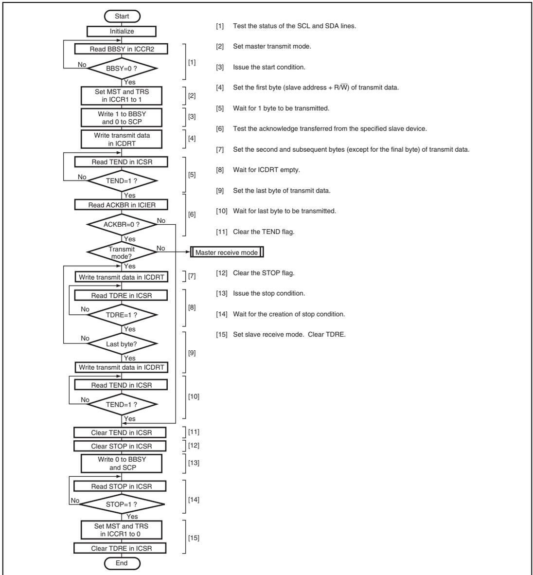
**Figure 20.14 Sample Flowchart for Master Transmit Mode**
