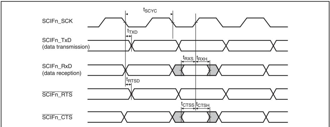
**Figure 33.53** SCI Input/Output Timing in Clock Synchronous Mode
