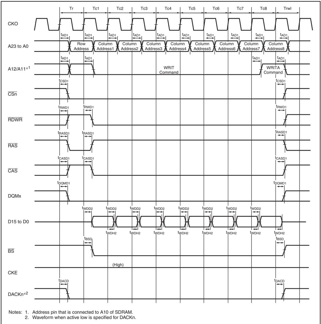
**Figure 33.23 Burst Write Bus Cycle of SDRAM (Single Write × 8)**
