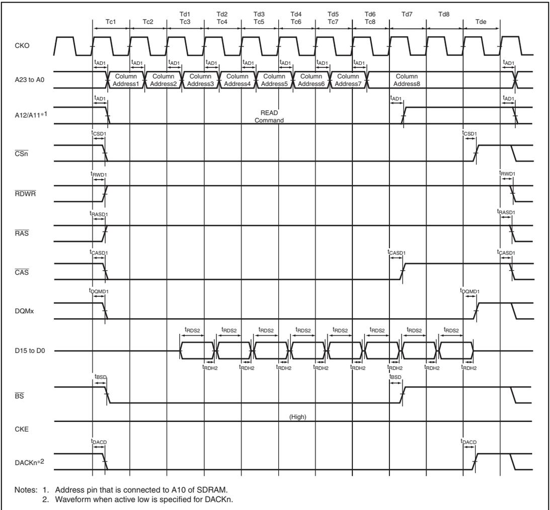
**Figure 33.25 Burst Read Bus Cycle of SDRAM (Single Read × 8)**
