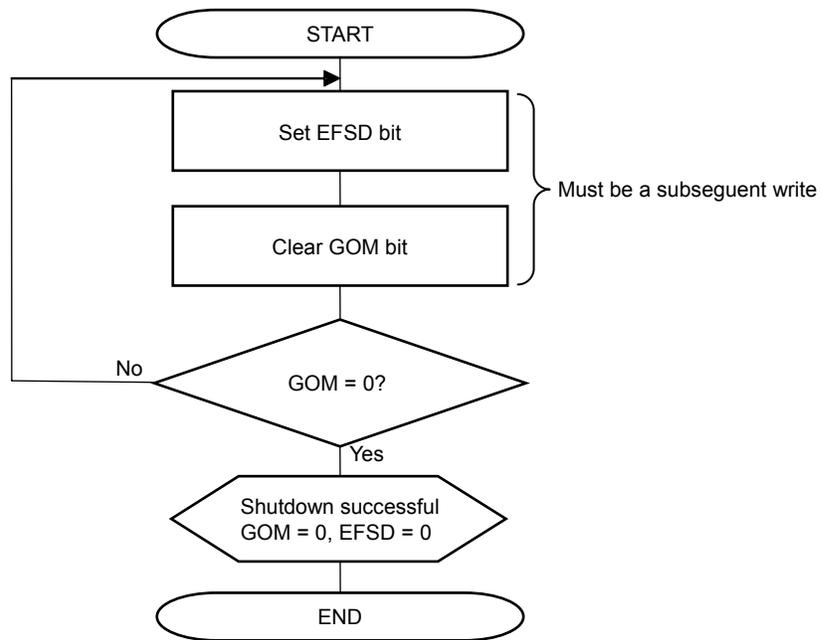
**Caution** Do not read- or write-access any registers by software between setting the EFSD bit and clearing the GOM bit.
