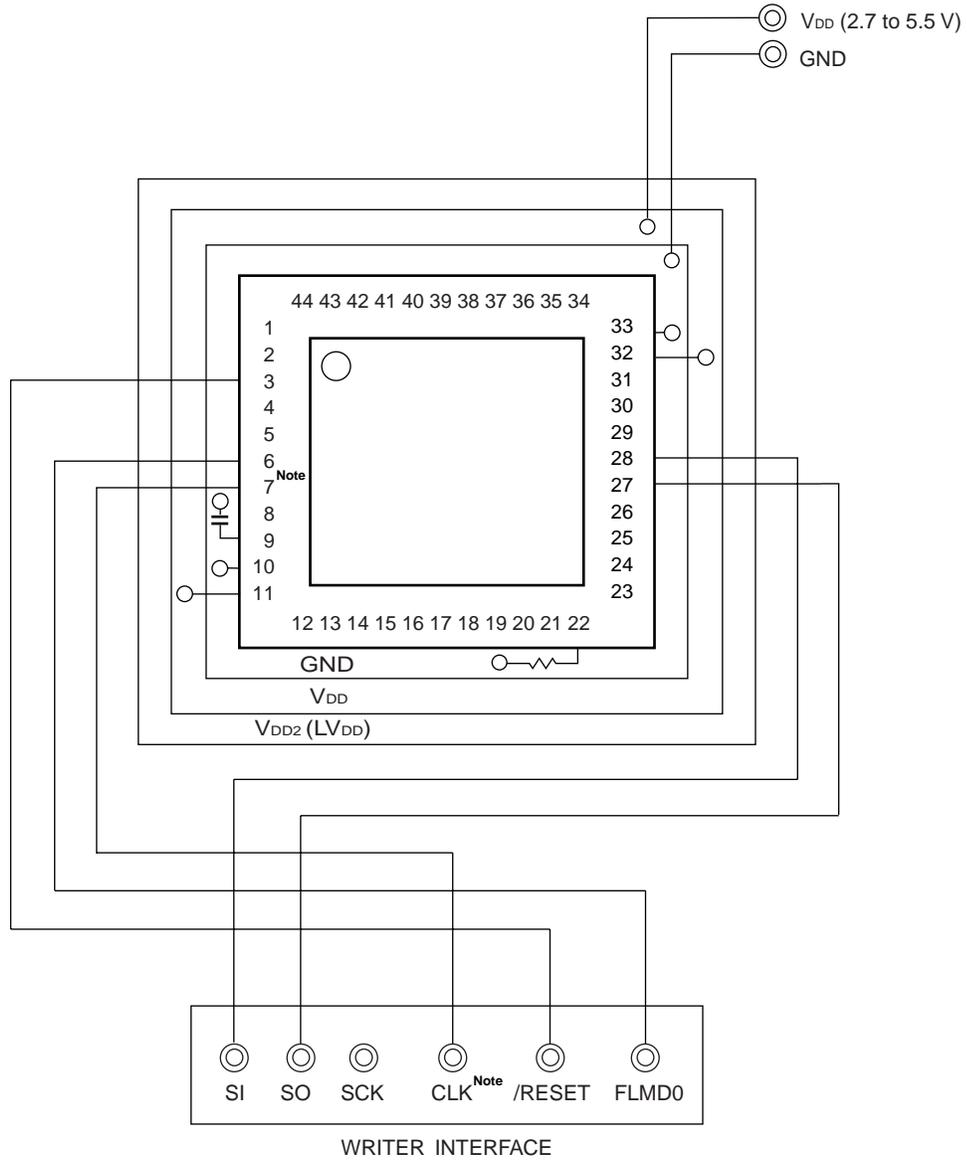
**Note** The above figure illustrates an example of wiring when using the clock output from the PG-FP5 or FL-PR5 or PG-FP4 or FL-PR4.
