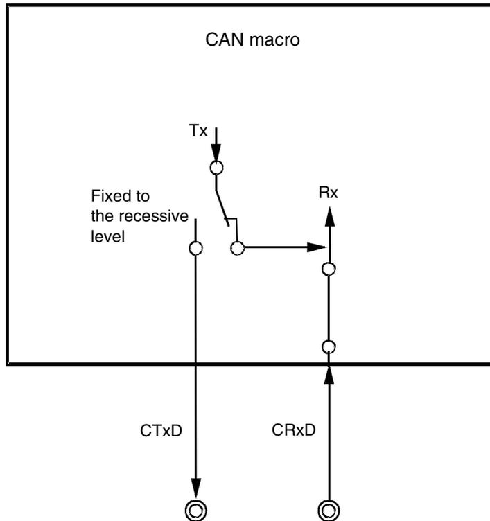
In the receive-only mode, no message frames can be transmitted from the CAN module to the CAN bus. Transmit requests issued for message buffers defined as transmit message buffers are held pending.
