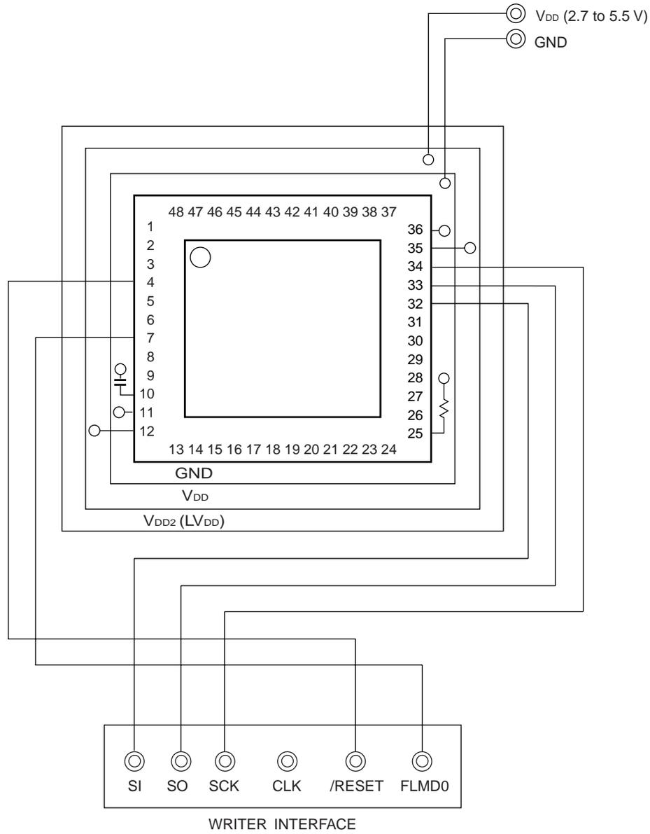
**Figure 24-6. Example of Wiring Adapter for Flash Memory Writing in UART (UART60) Mode
