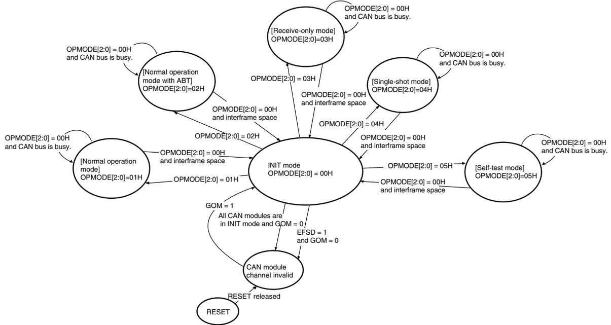
The transition from the initialization mode to an operation mode is controlled by the bit string OPMODE [2:0] in the C0CTRL register.
