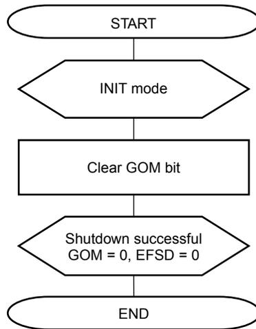
Figure 16-59. Forced Shutdown Process
