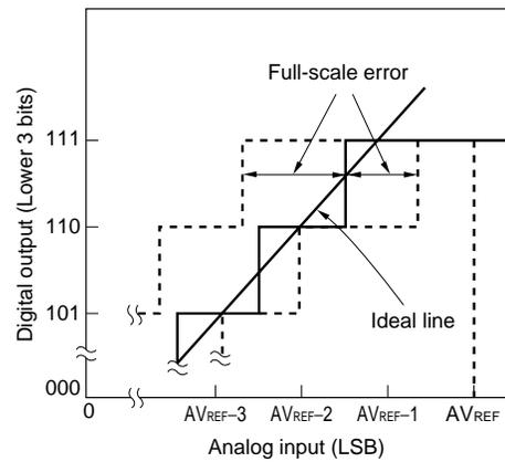
**Figure 13-19. Integral Linearity Error**
