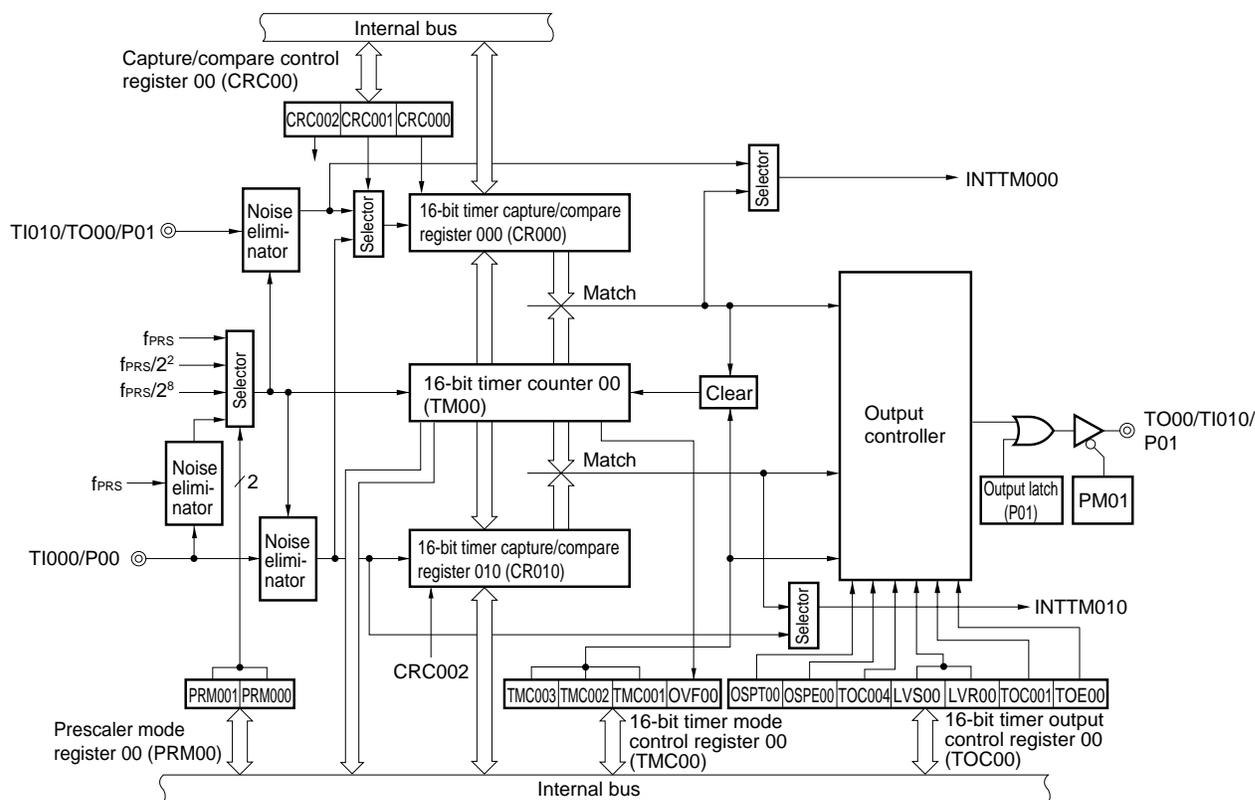
Figure 7-2. Block Diagram of 16-Bit Timer/Event Counter 01 ( $\mu$ PD78F0881A, 78F0882A, 78F0883A of 78K0/FC2)
