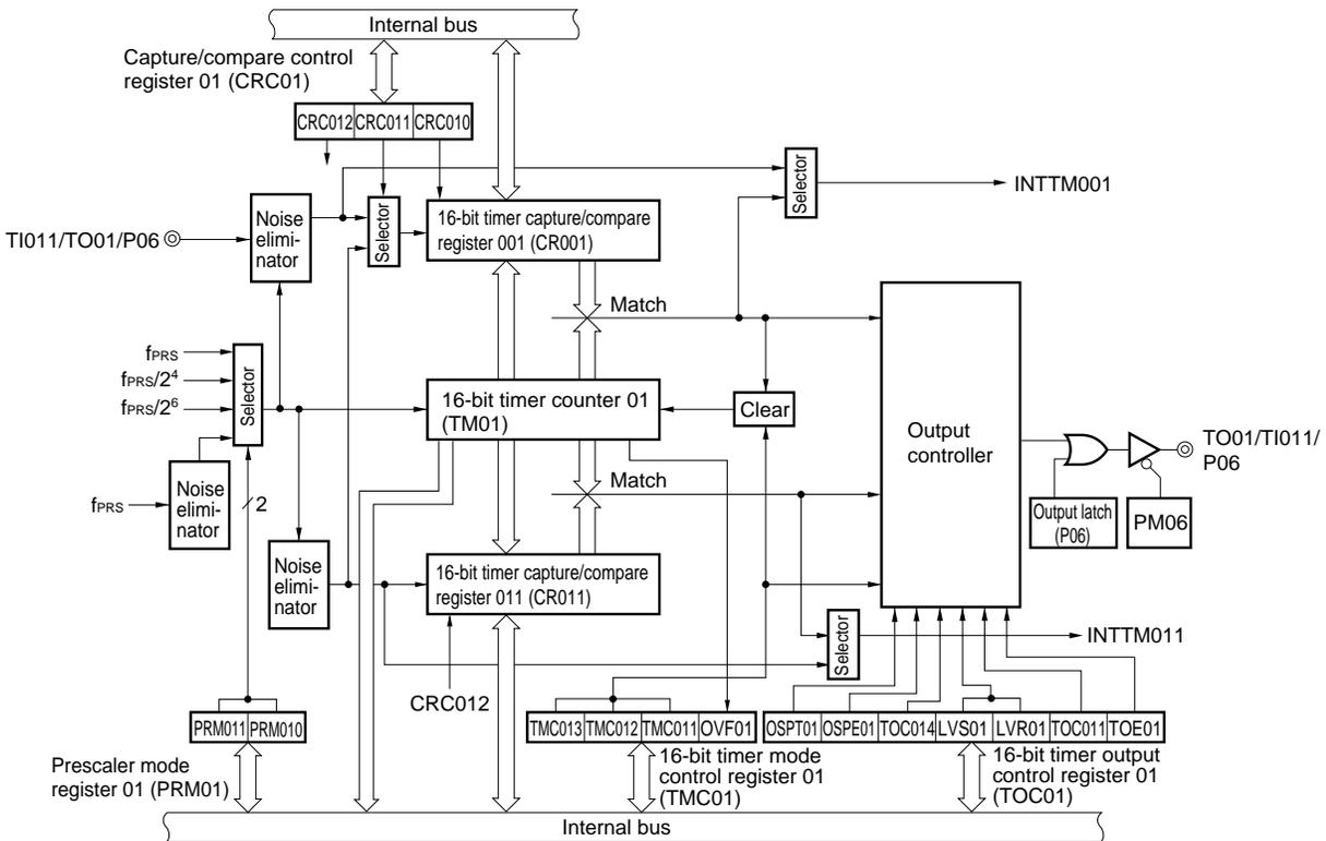
Figure 7-4. Block Diagram of 16-Bit Timer/Event Counter 01 (78K0/FE2, 78K0/FF2)
