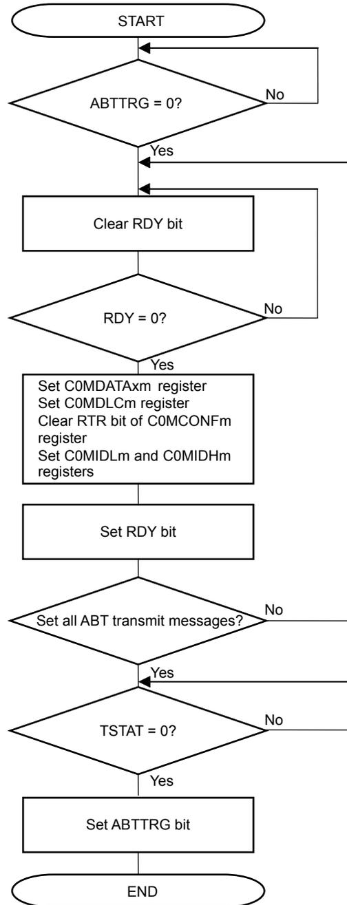
**Caution** The ABTTRG bit should be set to 1 after the TSTAT bit is cleared to 0. Checking the TSTAT bit and setting the ABTTRG bit to 1 must be processed continuously.
