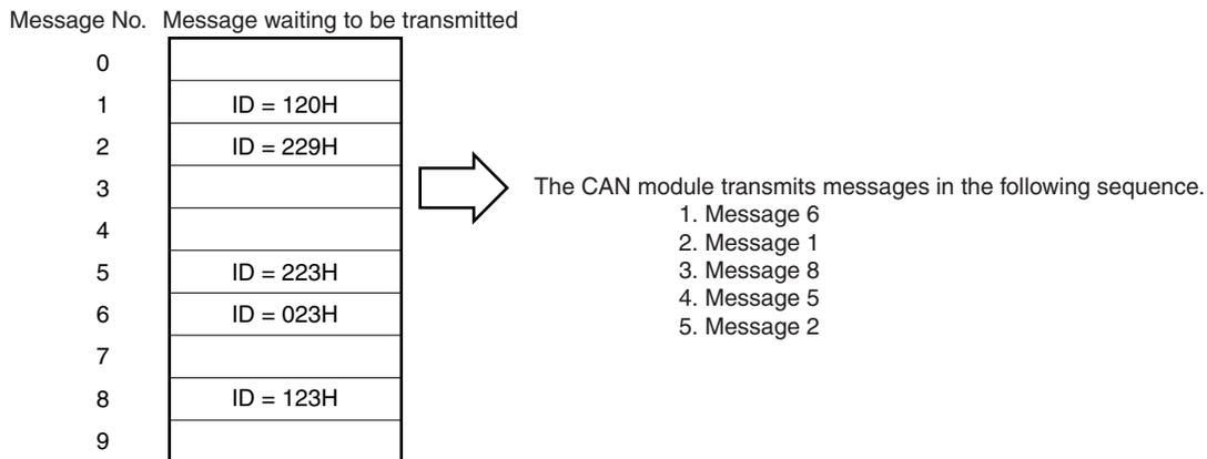
After the transmit message search, the transmit message with the highest priority of the transmit message buffers that have a pending transmission request (message buffers with the TRQ bit set to 1 in advance) is transmitted.
