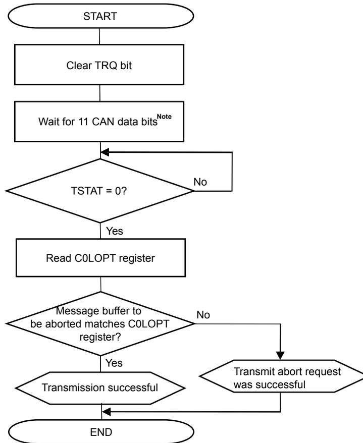
**Note** There is a possibility of starting the transmission without being aborted even if TRQ bit is cleared, because the transmission request to protocol layer might already been accepted between 11 bits, total of interframe space (3 bits) and suspend transmission (8 bits).
