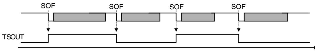
TSOUT signal toggles its level upon occurrence of the selected event during data frame reception (in the above timing diagram, the SOF is used as the trigger event source). To capture a timer value by using TSOUT signal, the capture timer unit must detect the capture signal at both the rising edge and falling edge.
