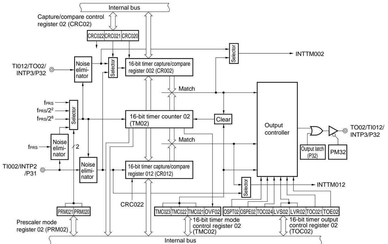
Figure 7-6. Block Diagram of 16-Bit Timer/Event Counter 03
