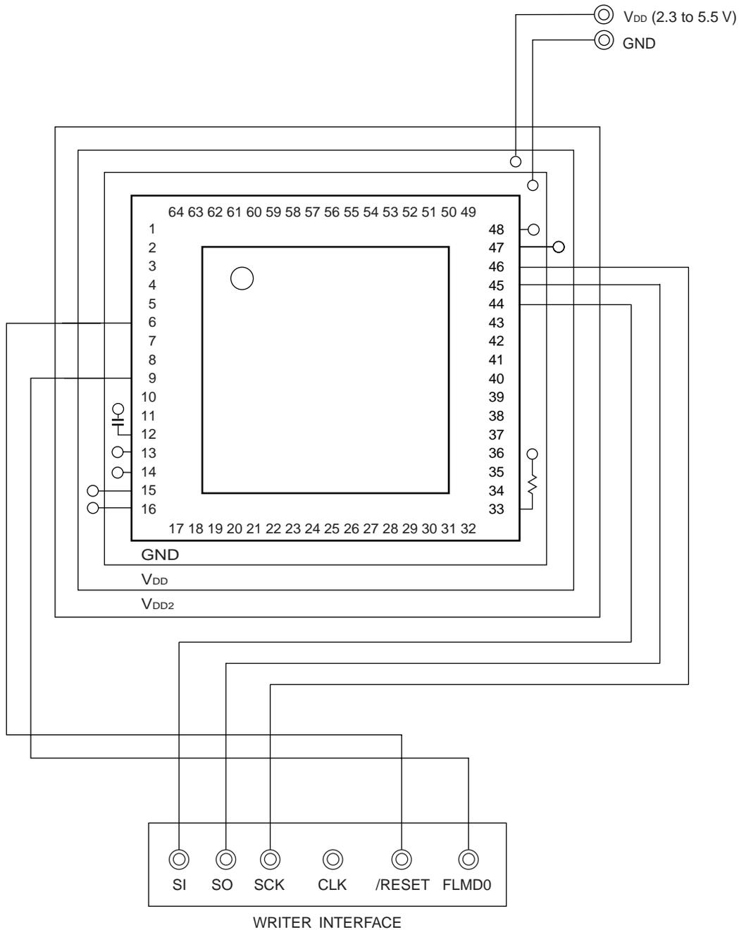
Figure 24-8. Example of Wiring Adapter for Flash Memory Writing in UART (UART60) Mode (78K0/FE2)
