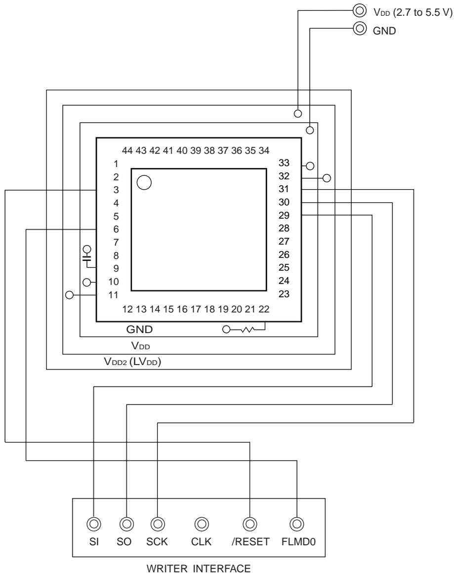
Figure 23-4. Example of Wiring Adapter for Flash Memory Writing in UART (UART60) Mode ( $\mu$ PD78F0881A, 78F0882A, 78F0883A or 78K0/FC2)
