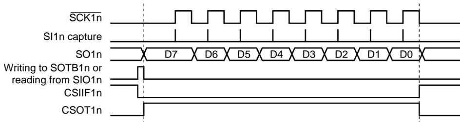
**Remarks 1.** The above figure illustrates a communication operation where data is transmitted with the MSB first.
