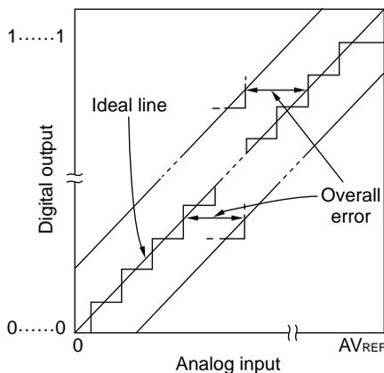
Figure 13-16. Quantization Error
