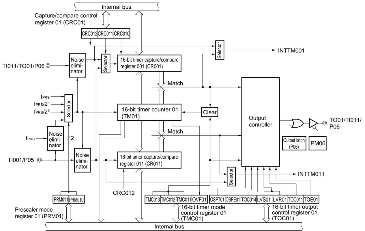
Figure 7-5. Block Diagram of 16-Bit Timer/Event Counter 02
