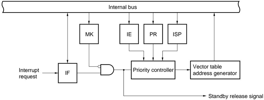
(B) External maskable interrupt (INTP0 to INTP7)
