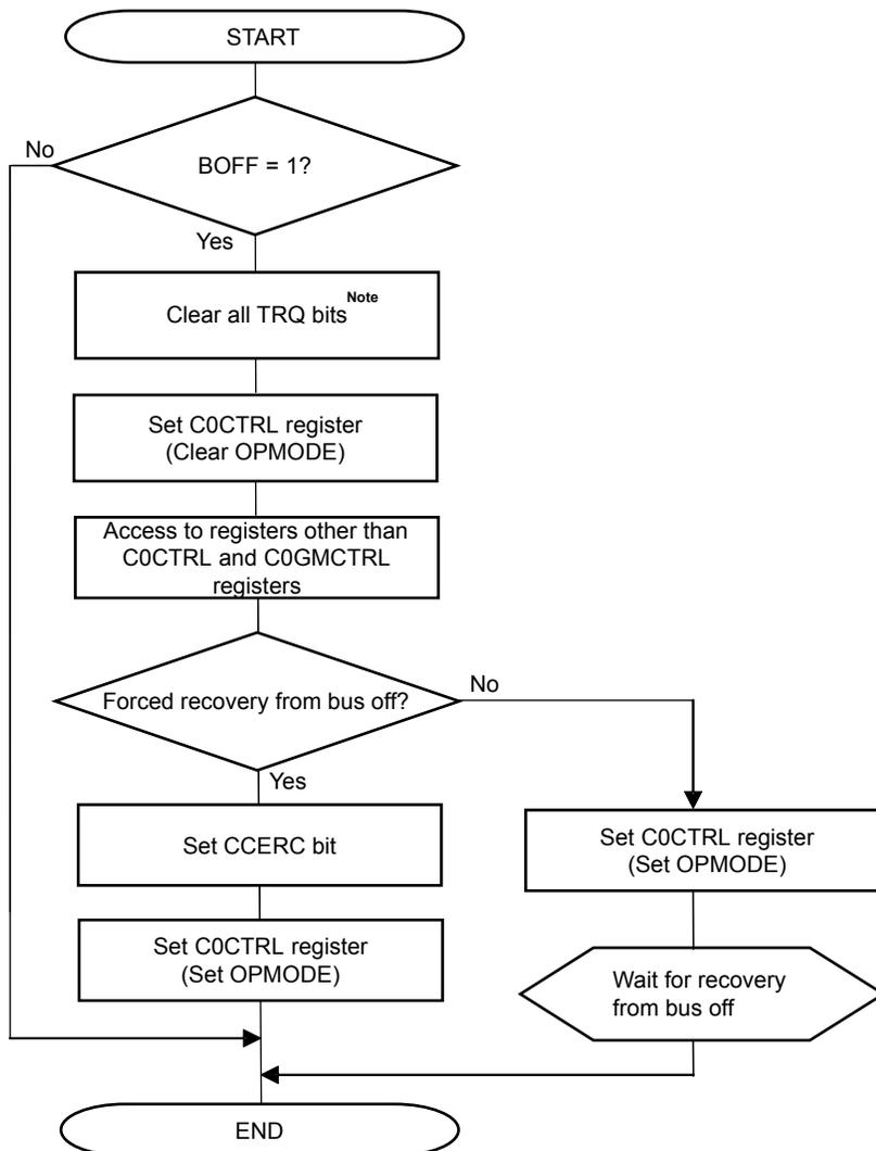
**Note** Clear all TRQ bits when re-initialization of message buffer is executed by clearing RDY bit before bus-off recovery sequence is started.
