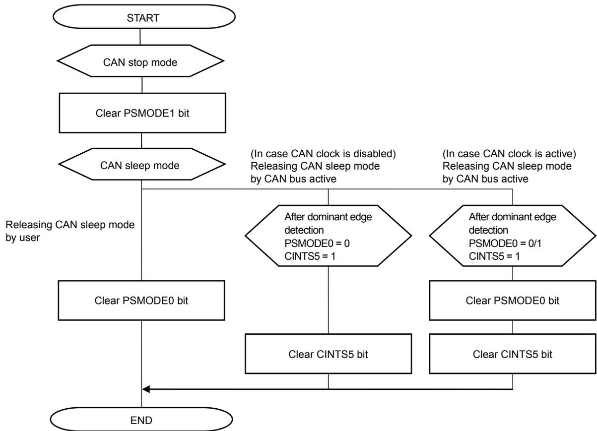
**Remark** "In case CAN clock is disabled": By means of the CPU standby mode, the CAN module clock has been switched off, and the CAN module is in sleep mode.
