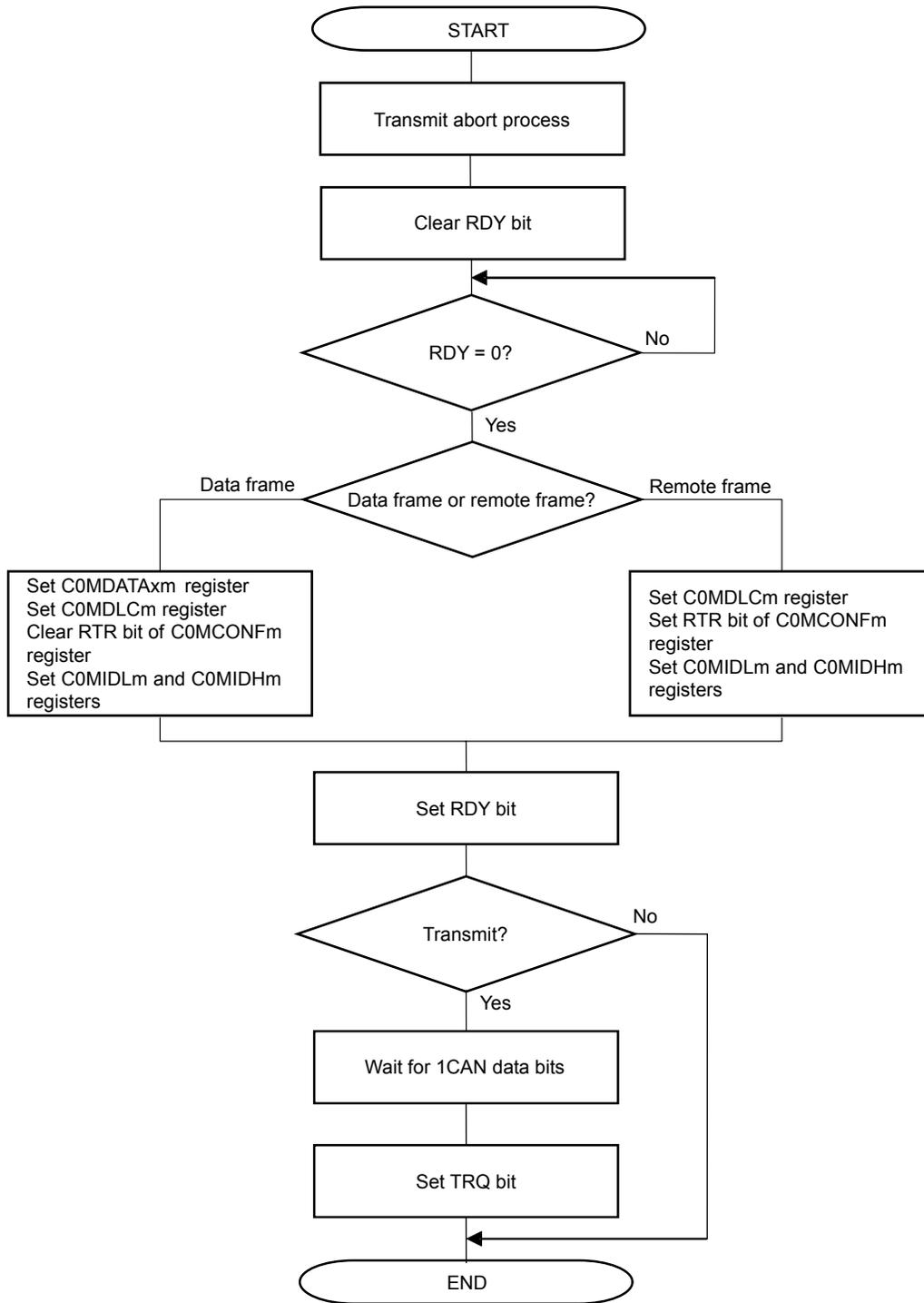
Figure 16-42 shows the processing for a transmit message buffer (MT [2:0] bits of COMCONFm register = 000B).
