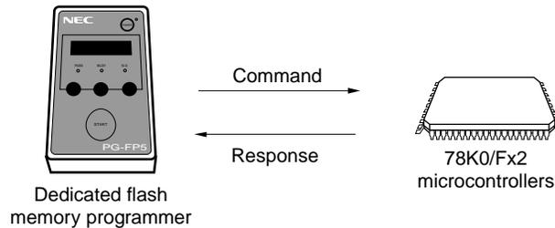
The flash memory control commands of the 78K0/Fx2 microcontrollers are listed in the table below. All these commands are issued from the programmer and the 78K0/Fx2 microcontrollers perform processing corresponding to the respective commands.
