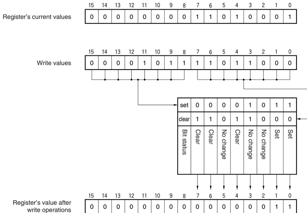
Figure 16-24. 16-Bit Data during Write Operation
