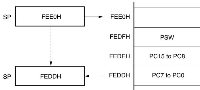
Figure 3-16. Data to Be Restored from Stack Memory
