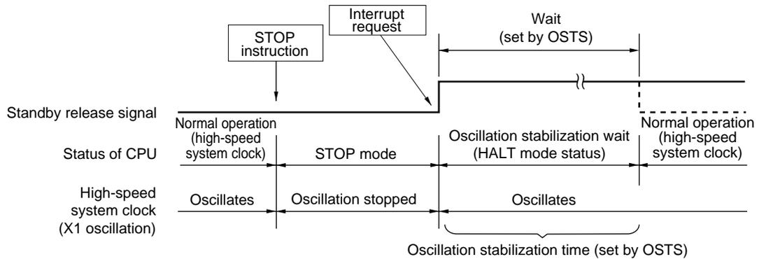
**(2) When high-speed system clock (external clock input) is used as CPU clock (1/2)**
