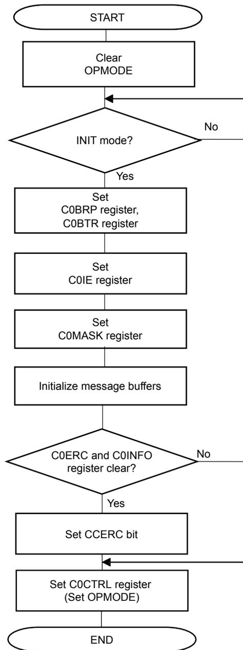
**Caution** After setting the CAN module to the initialization mode, avoid setting the module to another operation mode immediately after. If it is necessary to immediately set the module to another operation mode, be sure to access registers other than the C0CTRL and C0GMCTRL registers (e.g. set a message buffer).
