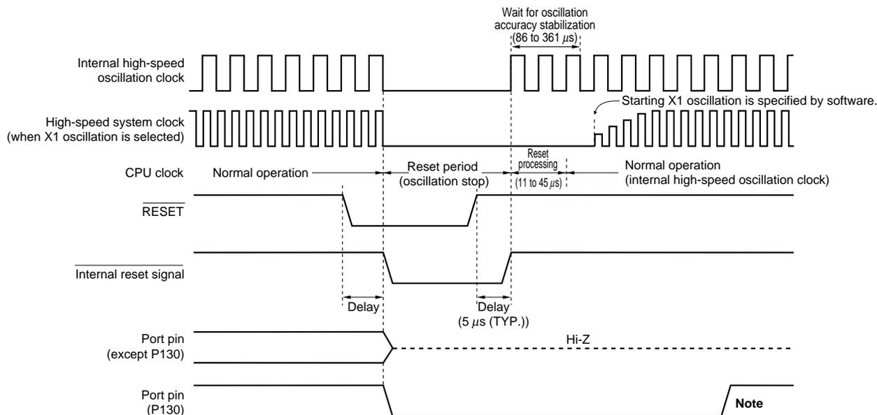
**Note** Set P130 to high-level output by software.
