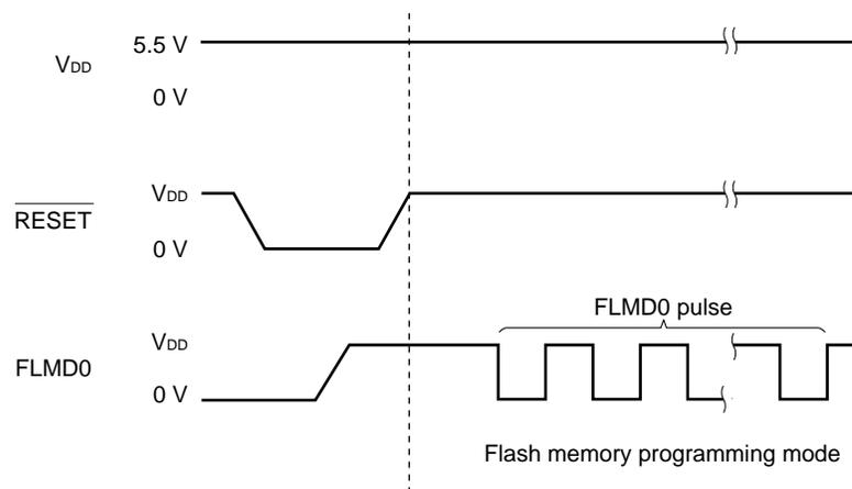
**Table 24-9. Relationship Between FLMD0 Pin and Operation Mode After Reset Release**
