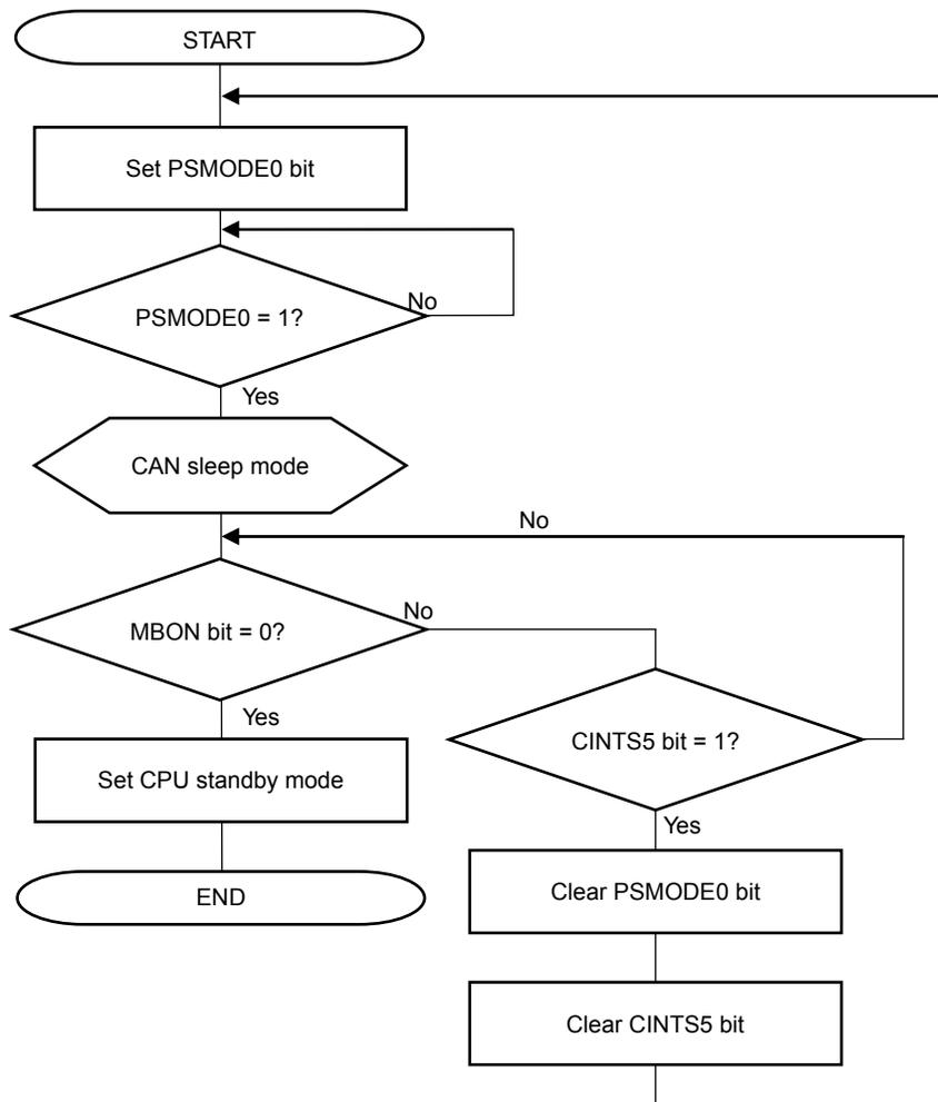
**Caution** Before the CPU is set in the CPU standby mode, please check the CAN sleep mode or not. However, after check of the CAN sleep mode, until the CPU is set in the CPU standby mode, the CAN sleep mode may be cancelled by wakeup from CAN bus.
