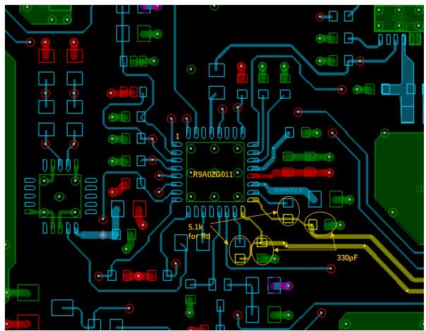
Figure 1-4 Rd resister and decoupling capacitor for CC line
