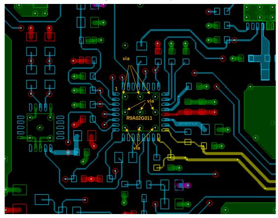
Figure 1-2 Via under E-pad
