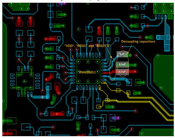
Figure 1-3 Decoupling capacitor
