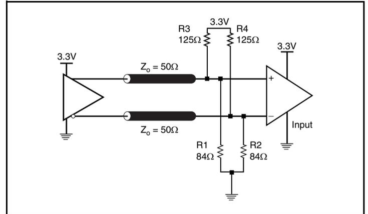
Figure 7B. 3.3V LVPECL Output Termination
