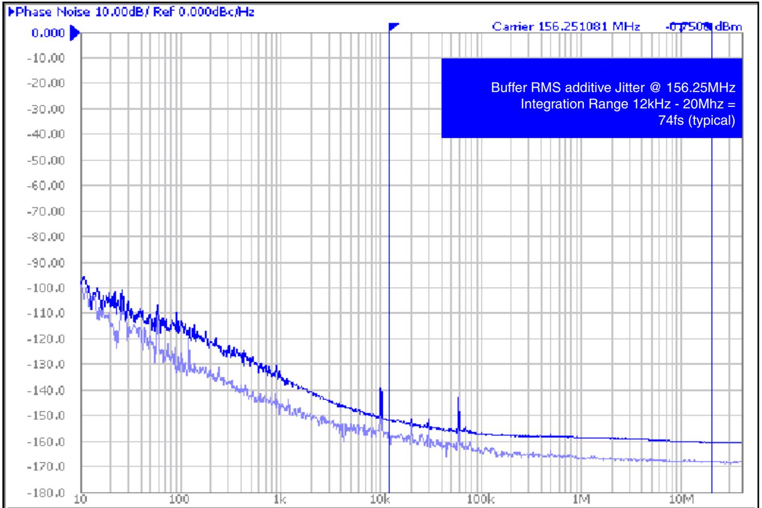
As with most timing specifications, phase noise measurements have issues relating to the limitations of the equipment. Often the noise floor of the equipment is higher than the noise floor of the device. This is illustrated above. The device meets the noise floor of what is shown, but can actually be lower. The phase noise is dependent on the input source and measurement equipment.
