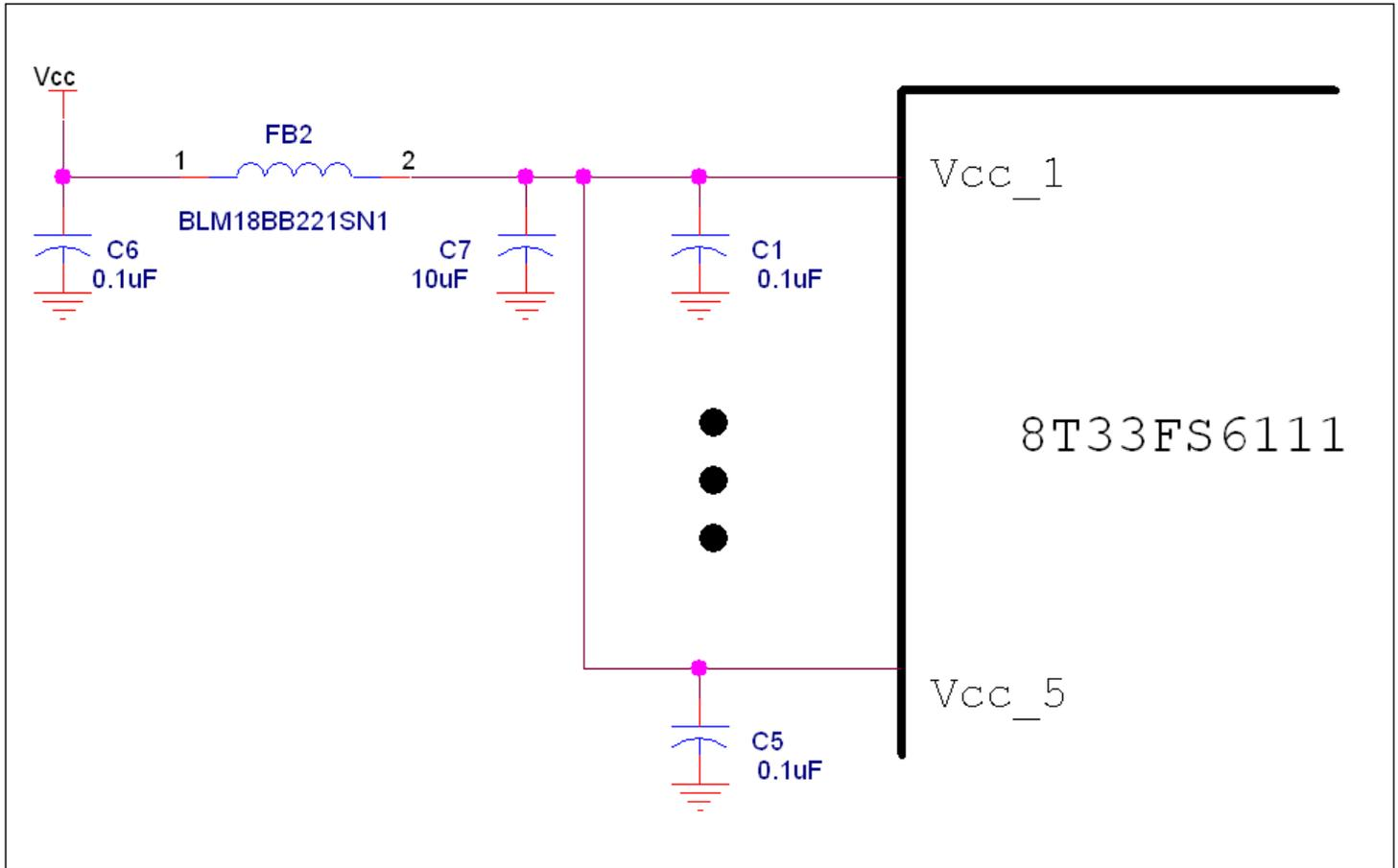
Figure 2. V<sub>CC</sub> Power Supply Bypass
