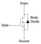
**Remark** Strong electric field, when exposed to this device, can cause destruction of the gate oxide and ultimately degrade the device operation. Steps must be taken to stop generation of static electricity as much as possible, and quickly dissipate it once, when it has occurred.
