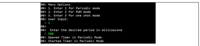
In periodic mode, the user can enter the duty cycle, then LED starts blink.
