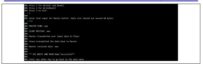
Enter "2" to run WriteRead() example. User can specify the data for Master and Slave. Transmission will be performed after inputting each data. Master received data and Slave received data will be shown on console once the transmission complete.
