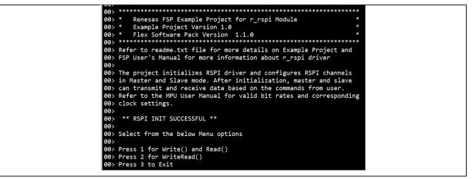
Enter "1" to run Write() and Read() example and transmission will be performed after input data from Master to Slave. Then, Slave sends back same data to Master.
