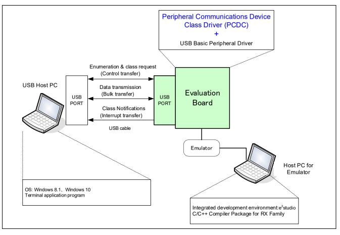
Figure 3-1 Example Operating Environment (Echo Mode)
