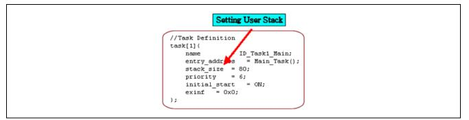
Figure 4 Defining User Stack in Configurator File
