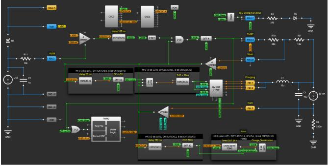
Figure 3. CCCV Battery Charger GreenPAK (HVPAK) Design
