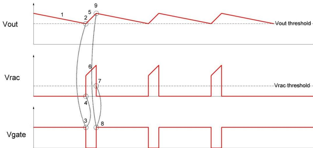
**Figure 2: CCSS Regulator Timing**
