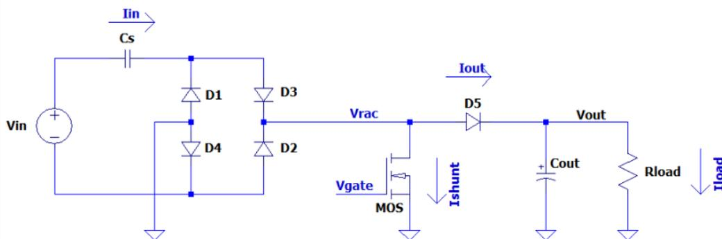
**Figure 1: Capacitor-Coupled Switched Shunt Regulator**
