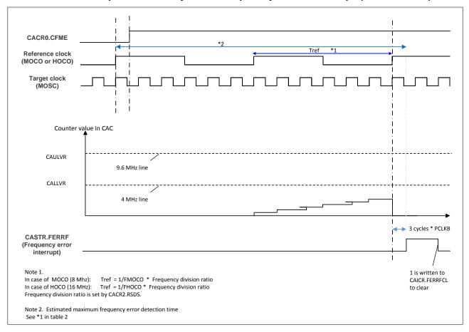
Figure 2 CAC frequency error interrupt for oscillation detection stop
