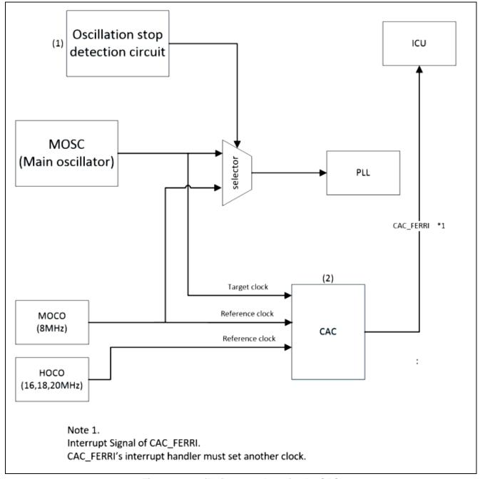
Figure 1 Oscillation stop detection by CAC
