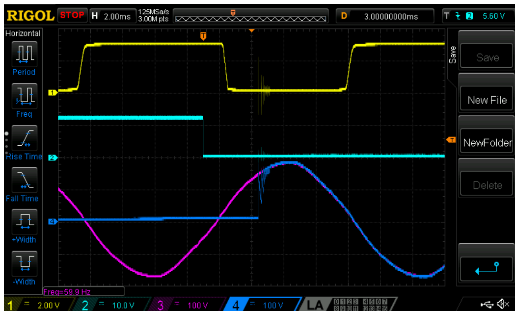
Figure 8: Relay Does Not Close at True Zero-Crossing with 7.407ms Delay
