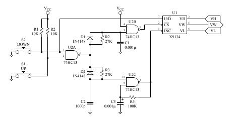
FIGURE 3. SIMPLE 3-WIRE XDCP EVALUATION CIRCUIT
