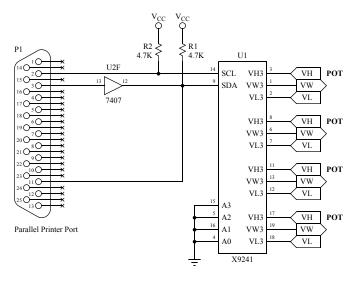
FIGURE 2. X9221, X9241 EVALUATION CIRCUIT
