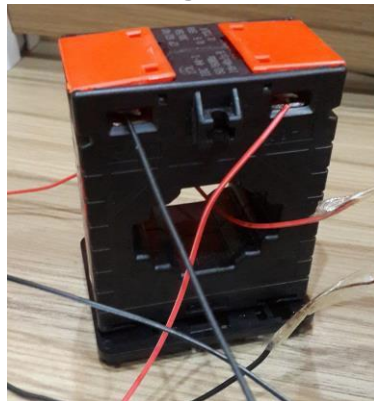
Figure 12. Ring main Current Transformer
