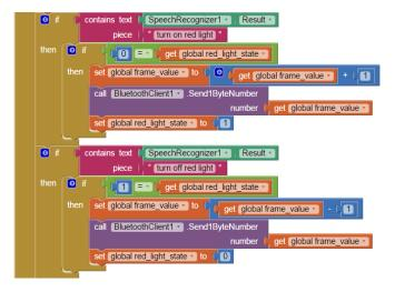
Figure 6. Red Light Control Block Diagram
