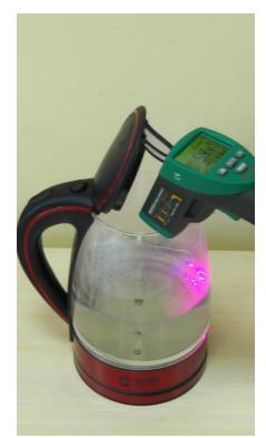
7. LED effect at  $67^{\circ}C^{1}$  8. LED effect at  $72^{\circ}C^{1}$  9. LED effect at  $93^{\circ}C^{1}$
