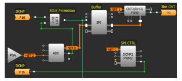
Figure 5. SPI buffer
