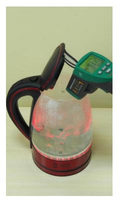
$^{1}\text{Thermometer}$  Accuracy is ±2.5  $^{\text{o}}\text{C}$
