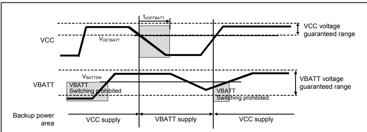
Note. The VBATT voltage when the supplied power source switches from Vcc to  $V_{BATT}$  should not be lower than  $V_{BATTSW}$ , the lower-limit VBATT voltage for switching between power supplies due to a drop in the VCC voltage.
