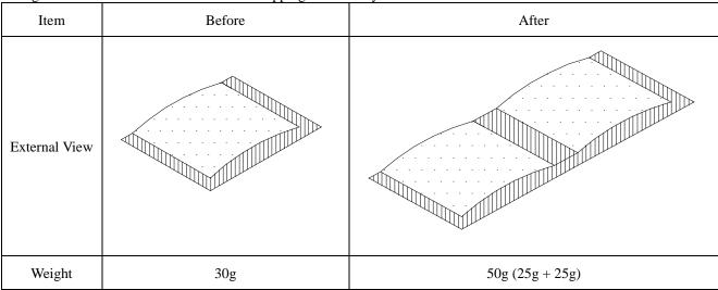
5-4. Change specification of the moisture sensing indicator for JEDEC trays
