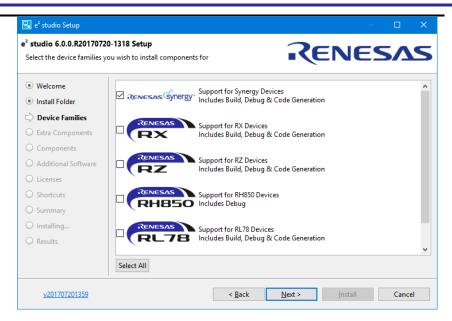
The above example shows a user only installing the Synergy device family. Subsequent updates of other device families will not affect this installation unless the main core of the product is also updated.
