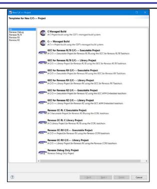
Note the C Managed Build and C++ Managed Build types are default CDT projects. Please use the Renesas project types for the device you wish to use. There are separate entries for each device, toolchain and project type (Executable or Library) combination.
