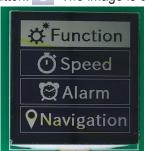
m. Pressing the user switch (one of SW1 to SW2) on the main board changes the image on the MIP-LCD. The following is the image after pressing SW1.
