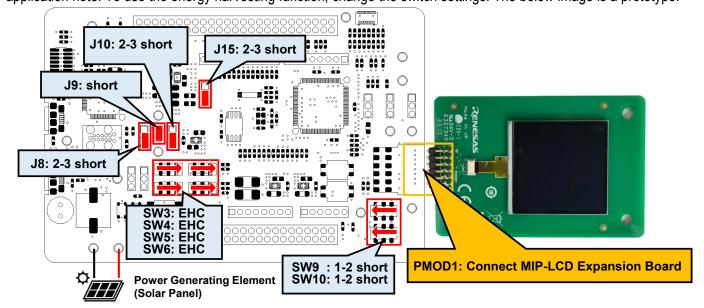
Light blue hatching is a switch to change when using the energy harvesting function.
