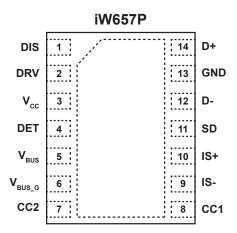
Figure 4.1 : 14-Lead TDFN 4x3mm Package (Top View, Transparent)
