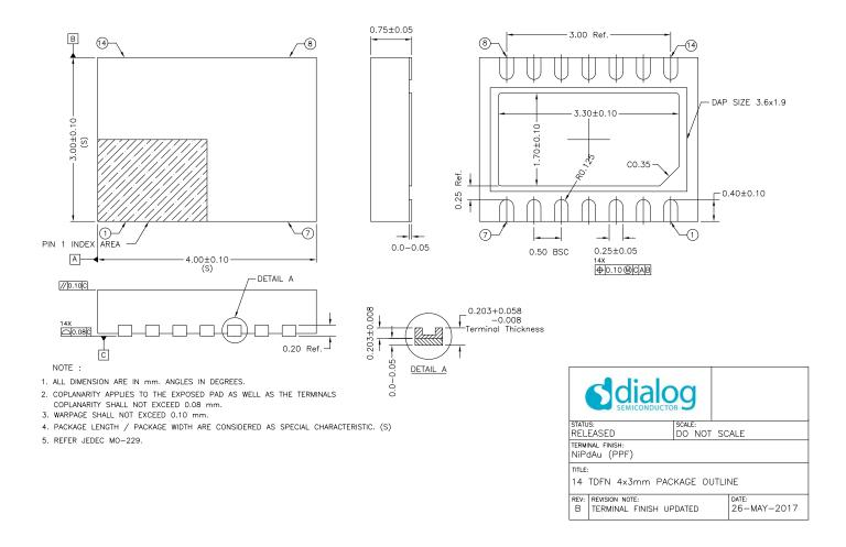
Figure 6.1: 14-Lead TDFN 4x3mm Package
