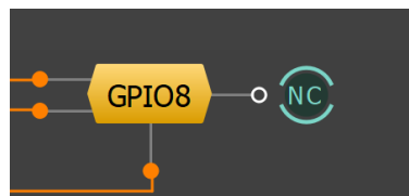
Figure 33. NC (not connected)
