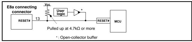
Figure 4.3 Example of a Reset Circuit
