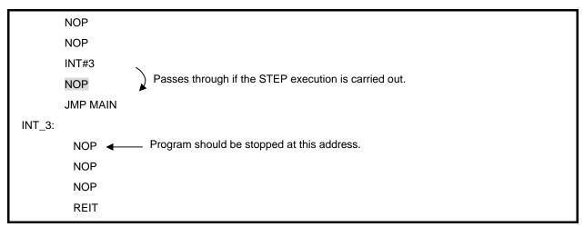
Figure 6.2 Example of Software Interrupt Instruction
