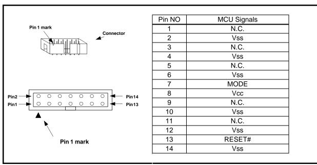
Figure 3.2 E8a Connecting Connector Pin Assignments
