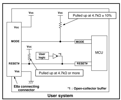
Figure 4.1 Example of an E8a Connection
